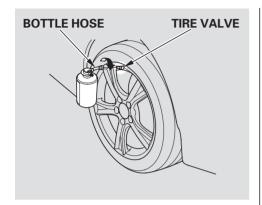
4. Screw the sealant filler hose onto the tire valve. Make sure the bottle remains upright to ensure all of the sealant flows into the tire.
