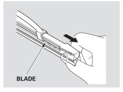
3. Remove the blade from its holder by grasping the tabbed end of the blade. Pull firmly until the tabs come out of the holder.
