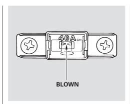
3. Check each of the large fuses in the primary under-hood fuse box by looking through the top at the wire inside. Removing these fuses requires a Phillips-head screwdriver.
