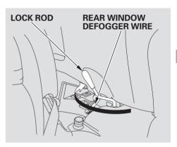
14.Pivot the lock rods backward to lock down the sides of the hardtop. Make sure the rear window defogger wire is set under the lock rod to ensure the wire is not crushed or entangled.
