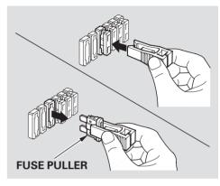
4. Check the smaller fuses in the under-hood fuse boxes and all the fuses in the interior fuse box by pulling out each one with the fuse puller provided in the interior fuse box.
