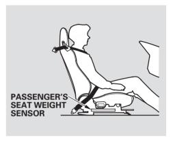
The passenger's advanced airbag system has weight sensors under the seat. Although Honda does not encourage carrying a child in the passenger's seat, if the sensors detect the weight of an infant or small child (up to about 65 lbs or 29 kg), the system will automatically turn the passenger's airbag off.
