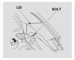
2. Loosen the bolt of the rear cover lid with a flat-tipped screwdriver.
