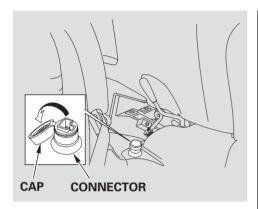
15.Remove the cap from the rear window defogger connector.
