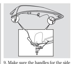
lock pins are pivoted forward to the first stop. However, do not pull the handle all the way forward (touching the inside of the top).
