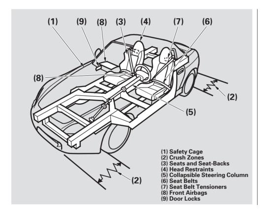
Your vehicle is equipped with many features that work together to protect you and your passenger during a crash.
