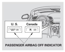
This indicator alerts you that the passenger's airbag has been shut off because weight sensors detect about 65 lbs (29 kg) or less (the weight of an infant or small child) on the passenger's seat. It does *not mean* there is a problem with the airbag.
