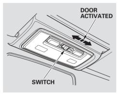
The interior light has a three-position switch: ON, Door Activated, and OFF. In the Door Activated (center) position, the light comes on when you:
