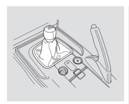
The manual transmission is synchronized in all forward gears for smooth operation. It has a lockout so you cannot shift directly from fifth to reverse instead of sixth (see page 148). When shifting up or down, make sure you push the clutch pedal down all the way, shift to the next gear, and let the pedal up gradually. When you are not shifting, do not rest your foot on the clutch pedal. This can cause your clutch to wear out faster.
