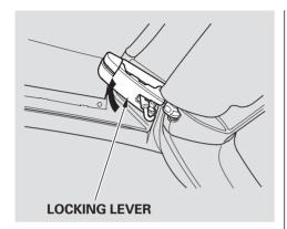
4. With the latches released, push the locking levers up until they latch.
