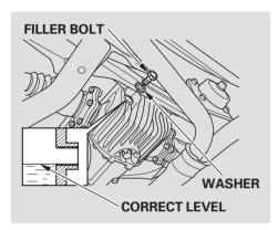
Check the fluid level with the differential at normal operating temperature and the vehicle sitting on level ground. Remove the differential fluid filler bolt and washer, and carefully feel inside the bolt hole with your finger. The fluid level should be up to the edge of the bolt hole. If it is not, slowly add fluid until it starts to run out of the hole.
