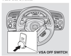
In certain unusual conditions when your vehicle gets stuck in shallow mud or fresh snow, it may be easier to free it with the VSA temporarily switched off. When the VSA system is off, the traction control system is also off. You should only attempt to free your vehicle with the VSA off if you are not able to free it when the VSA is on.
