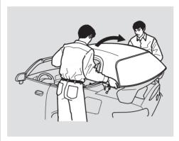
7. Lift the hardtop straight up off the vehicle and set it aside.
