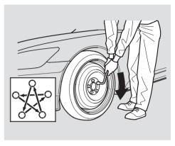
13. Tighten the wheel nuts securely in a crisscross pattern. Have the wheel nut torque checked at the nearest automotive service facility. Tighten the wheel nuts to: 80 lbf·ft (108 N·m, 11 kgf·m)
