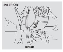
The interior fuse box is underneath the dashboard on the driver's side. To open it, turn the knob.
