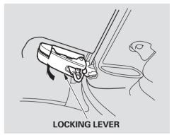
5. With the latches released, pull back on the locking levers and push them up until they latch.
