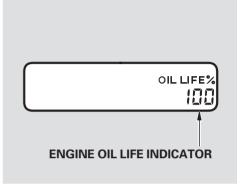
4. Press the TRIP button for about 5 seconds. The maintenance items code(s) will disappear, and the engine oil life will reset to "100."
