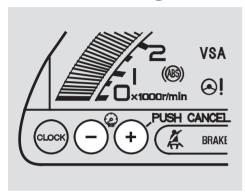
The buttons in the lower left corner of the instrument panel adjust the brightness of the display in five steps. Push the + or - button five times to see the full range.
