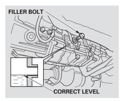
Check the fluid level with the transmission at normal operating temperature and the vehicle sitting on level ground. Remove the transmission filler bolt, and carefully feel inside the bolt hole with your finger. The fluid level should be up to the edge of the bolt hole. If it is not, add Honda Manual Transmission Fluid (MTF) until it starts to run out of the hole. Install the filler bolt, and tighten it securely.
