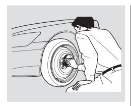
11.Put on the spare tire. Put the wheel nuts back on finger-tight, then tighten them in a crisscross pattern with the wheel nut wrench until the wheel is firmly against the hub. Do not try to tighten the wheel nuts fully.
