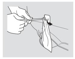
For very short distances, such as freeing the vehicle, you can use the detachable towing hook that mounts on the anchors in the front and rear bumpers.
