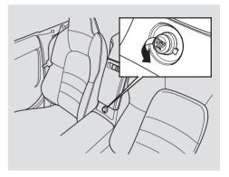
This socket is intended to supply power for 12 volt DC accessories that are rated 120 watts or less (10 amps). It will not power an automotive type cigarette lighter element.
