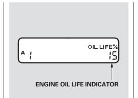
3. Press the TRIP button for about 10 seconds. The engine oil life indicator and the maintenance item code(s) will blink.
