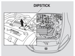
Wait a few minutes after turning the engine off before you check the oil.
