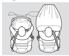
Your vehicle has a supplemental restraint system (SRS) with front airbags to help protect the heads and chests of the driver and a passenger during a moderate to severe frontal collision (see page 22 for more information on how your airbags work).
