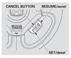
3. Press and release the SET/decel button on the steering wheel. The indicator on the instrument panel comes on to show the system is now activated.
