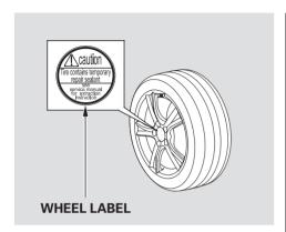
14.Remove the wheel label from the repair kit and attach it to the center of the wheel.
