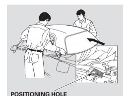
10.Carefully set the removable hardtop on the vehicle, making sure the lock rods go into the positioning holes behind each door. Be careful not to pinch your fingers.
