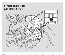
The auxiliary under-hood fuse box is on the driver's side, near the brake fluid reservoir. To open it, push the tab on each side, and remove the lid.
