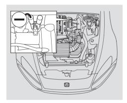
4. Connect the second jumper cable to the negative (—) terminal on the booster battery. Connect the other end to the boss on the intake manifold as shown. Do not connect this jumper cable to any other part of the engine.
