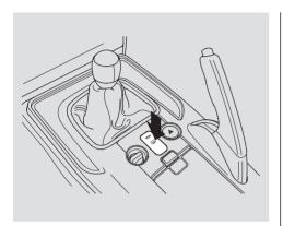
The rear window defogger will clear fog, frost, and thin ice from the window. Push the defogger button to turn it on and off. The indicator in the button comes on to show the defogger is on. If you do not turn it off, the defogger will shut itself off after about 15 minutes. It also shuts off when you turn off the ignition switch. You have to turn the defogger on again when you restart the vehicle.
