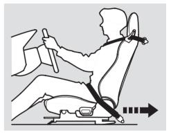
Adjust the driver's seat as far to the rear as possible while allowing you to maintain full control of the vehicle. Have a passenger adjust his or her seat as far to the rear as possible.
