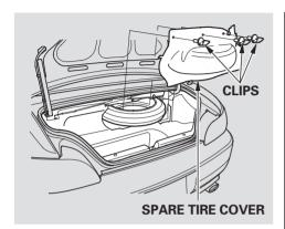
4. Remove the three clips holding the spare tire cover by pulling the rings straight back. Remove the spare tire cover.
