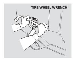
4. Screw the towing hook into the extension, and tighten it securely using the wheel nut wrench.
