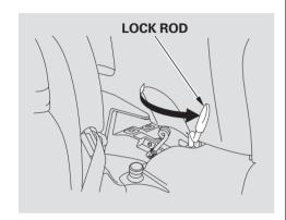
6. Pivot the lock rods forward to release the sides of the hardtop.
