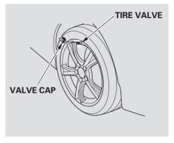
1. Position the vehicle so the tire valve on the flat tire is at the top of the wheel, then remove the tire valve cap.
