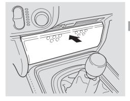
If equipped To open the audio panel, push on the top center, and let the panel swing down. To close, pivot the panel up, and push on it until it latches.
