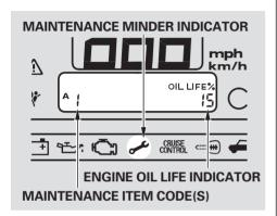
If the remaining engine oil life is 15 to 6 percent, you will see the engine oil life indicator every time you turn the ignition switch to the ON (II) position. The maintenance minder indicator will also come on, and the maintenance item code(s) for other scheduled maintenance items needing service will be displayed next to the engine oil life indicator.
