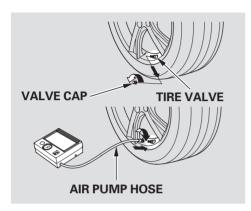
Remove the tire valve cap, screw the air pump hose onto the tire valve, and check the air gauge. (You do not need to attach the power cord or turn the air pump switch on.)
