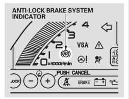
If this indicator comes on, the antilock function of the braking system has shut down. The brakes still work like a conventional system, but without anti-lock. You should have your dealer inspect your vehicle as soon as possible. Important Safety Reminders ABS does not reduce the time or distance it takes to stop the vehicle; it only helps with steering control during braking.
