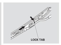
2. Disconnect the blade assembly from the wiper arm by pushing in the lock tab. Hold the lock tab in while you push the blade assembly toward the base of the arm.
