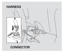
16.Plug the harness for the rear window defogger (see page 61) into the rear connector. Make sure it locks into the connector.
