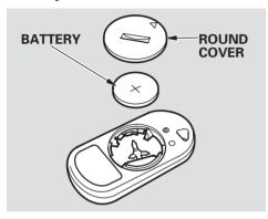
If it takes several pushes on the button to lock or unlock the doors, replace the battery as soon as possible.
