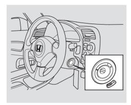
The ignition switch has three positions: LOCK (0), ACCESSORY (I), and ON (II).
