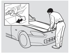
2. Put your fingers under the front edge of the hood near the center. Slide your hand to the left until you feel the hood latch handle. Push this handle to the left to release the hood. Lift up the hood.
