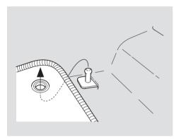
The floor mats that came with your vehicle hook over the floor mat anchors. This keeps them from sliding forward and possibly interfering with vehicle operation.
