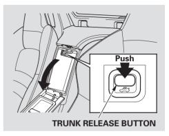
To open the trunk, press the trunk release button in the lower console compartment. To protect items in the trunk when you need to give the key to someone else, lock the lower console compartment with the master key, and give the other
