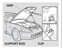
3. Holding the grip, pull the support rod out of its clip. Insert the end into the designated hole in the hood.
