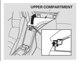
The lever to open the upper compartment is inside the lower compartment. Push up the lever, and lift the lid. To close, lower the lid, and push it down until it latches.
