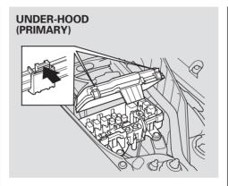
The primary under-hood fuse box is on the passenger's side next to the battery. To open it, push the two tabs as shown.
