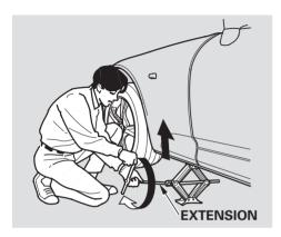
8. Use the extension and the wheel nut wrench as shown to raise the vehicle until the flat tire is off the ground.
