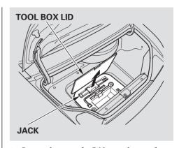
3. Open the trunk. Lift up the tool box lid, and take the jack, the wheel nut wrench, and the extension out of the tool box.
