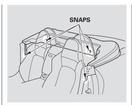
1. Remove the convertible top cover from the trunk, and lay it into position behind the roll bar.
