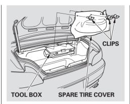
16.Replace the spare tire cover. Secure it with the three clips. Push each clip in securely, and pivot the ring down flat.
