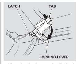
3. There is a latch on each side. Push in the tabs, and pull the locking levers down.
