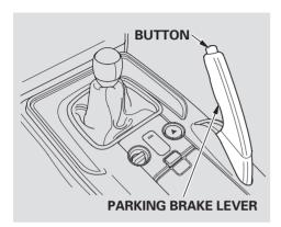
To apply the parking brake, pull the lever up fully. To release it, pull up slightly, push the button, and lower the lever. The parking brake indicator on the instrument panel should go out when the parking brake is fully released (see page 46).
