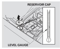
Check the fluid level by looking at the level gauge attached to the cap. Fill the reservoir with a good-quality windshield washer fluid. This increases the cleaning capability and prevents freezing in cold weather.
