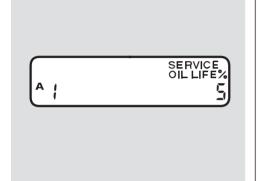
When the remaining engine oil life is 5 to 1 percent, you will see a "SERVICE OIL LIFE" message along with the same maintenance item code(s), every time you turn the ignition switch to the ON (II) position. The maintenance minder indicator ( ) also comes on and remains on in the instrument panel.
