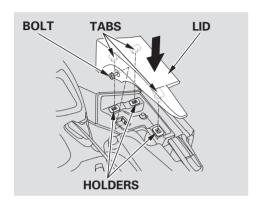
10. When reinstalling the rear cover lid, align the tabs to the appropriate holders and push the lid down while holding the bolt out.
