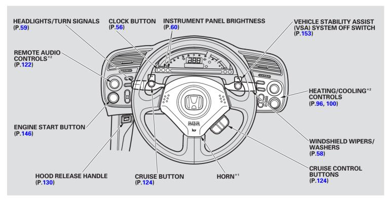
\*1: To use the horn, press the center pad of the steering wheel.
