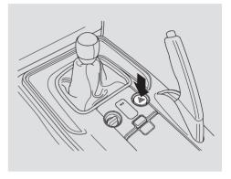
Push the red button next to the parking brake to turn on the hazard warning lights (four-way flashers). This causes all four outside turn signals and both indicators in the instrument panel to flash. Use the hazard warning lights if you need to park in a dangerous area near heavy traffic, or if your vehicle is disabled.
