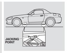
7. Place the jack under the jacking point nearest the tire you need to change. Turn the end bracket clockwise until the top of the jack contacts the jacking point. Make sure the center of the jacking point tab is resting in the jack notch.
