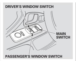
The driver's armrest has a master power window control panel. To open the passenger's window, push down on the switch and hold it until the window reaches the desired position. To close the window, pull back on the window switch. Release the switch when the window gets to the position you want.
