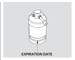
3. Remove the sealant bottle and check the expiration date on the label. If the date has expired, do not continue. Have your vehicle towed to the nearest Honda service center.
