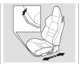
To adjust the seat forward and backward, pull up on the lever under the seat cushion's front edge. Then try to move the seat to make sure it is locked in position.
