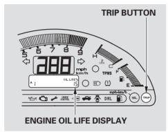
To see the current engine oil life, turn the ignition switch to the ON (II) position, and push and release the TRIP button repeatedly until the engine oil life display appears (see page 53).
