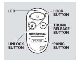
**LOCK** — Press this button once to lock both doors. Some exterior lights will flash. When you push LOCK twice within 5 seconds, you will hear a beep to verify that the doors are locked.
