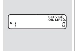
When the remaining engine oil life is 0 percent, the engine oil life indicator will blink. The display comes on every time you turn the ignition switch to the ON (II) position. The maintenance minder indicator ( ) also comes on and remains on in the instrument panel. When you see this message, immediately have the indicated maintenance done by your dealer.
