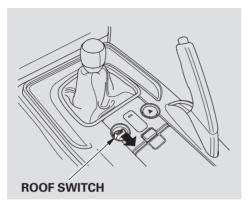
5. Pull back and hold the ROOF switch. The windows lower and the roof folds back. Release the ROOF switch when the roof is retracted completely into the rear shelf.
