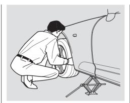
9. Remove the wheel nuts, then remove the flat tire. Handle the wheel nuts carefully; they may be hot from driving. Place the flat tire on the ground with the outside surface facing up.
