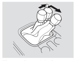
The manual transmission has a lockout so you cannot accidentally shift from fifth to reverse instead of sixth while the vehicle is moving.
