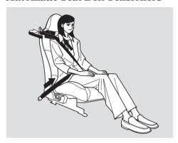
For added protection, the seat belts are equipped with automatic seat belt tensioners. When activated, the tensioners immediately tighten the belts to help hold the driver and a passenger in place.
