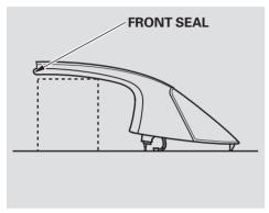
Support the hardtop during storage to prevent the front seal from making contact the floor or any other surface that can deform the rubber.
