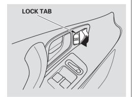
Each door has a lock tab next to the inside door handle. When you push in the lock tab on the driver's door, both doors lock. Pulling out the lock tab on the driver's door only unlocks that door. The lock tab on the passenger's door only locks and unlocks that door.
