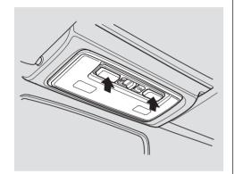
When the switch is in the center position with both doors closed, the two bulbs in the interior light can each be turned on and off with the button next to it.
