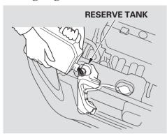
If the coolant level in the reserve tank is at or below the MIN line, add coolant to bring it up to the MAX line. Inspect the cooling system for leaks. Always use Honda All Season Antifreeze/Coolant Type 2. This coolant is pre-mixed with 50 percent antifreeze and 50 percent water. Never add straight antifreeze or plain water.
