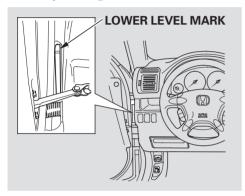
To check the windshield washer fluid level, open the driver's door, then look at the side of the reservoir tank located between the door and the front dashboard.
