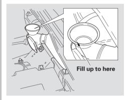
If the fluid level is below the lower level mark, fill the reservoir with windshield washer fluid.
