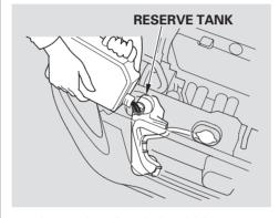
3. The coolant level should be up to the base of the filler neck. Add coolant if it is low.
