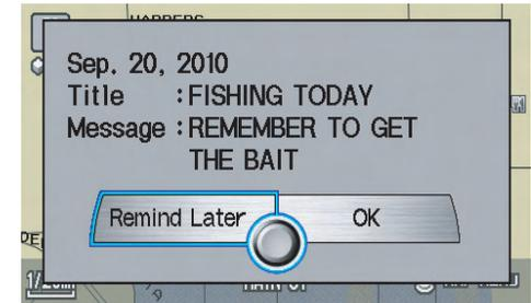
The Calendar reminder screen remains displayed until you select **OK** or **Remind Later** by rotating the **Interface Dial knob** and pushing in on the **Interface Dial**, or press the **CANCEL** button.
