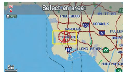
The red arrow indicates your vehicle position. Find your desired destination by moving the **Interface Dial** left, right, up, or down. The map and crosshairs will move in the same direction.
