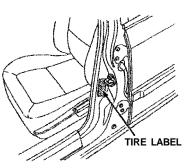
Check the tire pressures at least once a month, including the spare. Lower pressure than recommended lets the tread and sidewalls flex too much, causing increased tire temperatures, uneven wear, and poor handling. Pressure higher than recommended can make the tire too stiff, increasing the chance of damage from road hazards, and also causing uneven wear.
