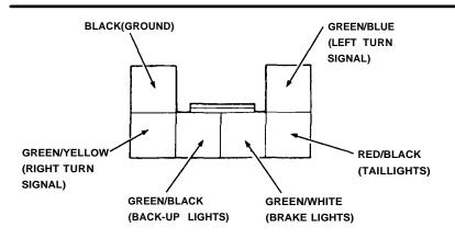
To connect your car's taillights to a trailer, an electrical converter must be installed in the car. Your car has separate bulbs for brake (red) and turn signal lights (amber), while most trailers use the same bulb for brake and turn signal lights. A converter, available at most trailer supply stores, should be installed according to the instructions supplied by the converter manufacturer.
