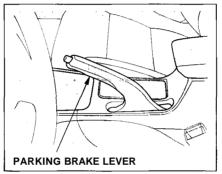
To apply the parking brake, pull the lever up fully. To release it, pull up slightly, push the button, and lower the lever. The parking brake light on the instrument panel should go out when the parking brake is fully released (see page 36). If you try to drive the car without releasing the parking brake, the ABS cannot work properly.
