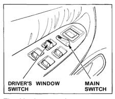
The driver's armrest has a master power window control panel. To open any of the passengers' windows, push down on the appropriate switch and hold it down until the window reaches the desired position. To close the window, push up on the window switch. Release the switch when the window gets to the position you want.
