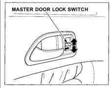
On all models except U.S. DX and Canadian LX models Each front door has a master door lock switch. Either switch locks and unlocks all doors. Push the switch down to lock all doors, and up to unlock them.
