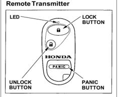
*On U.S. Special Edition model* You can lock and unlock your vehicle with the remote transmitter. When you push the LOCK button, all doors lock.
