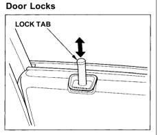
Each door has a lock tab on the top. Push the tab down to lock the door and pull it up to unlock.
