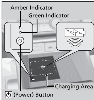
1. To turn the system on and off, press and hold the
