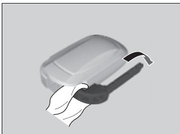
2. Remove the upper half of the cover by carefully prying on the slot with key grip.
