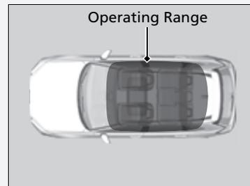
The engine may also start if the keyless remote is close to the door or window, even if it is outside the vehicle.
