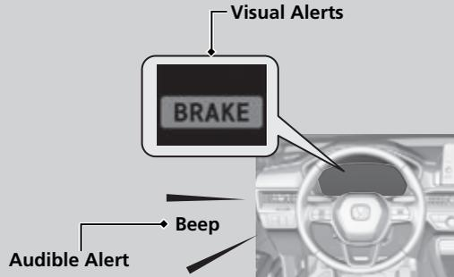
You can change the distance (**Long/Normal/Short**) between vehicles at which the system's earliest collision alert will come on.
