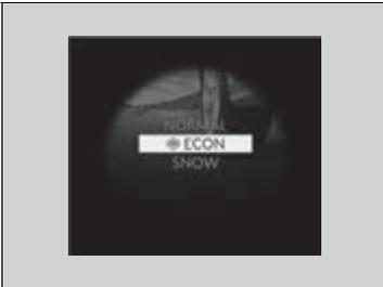
Facilitates fuel-efficient driving.
