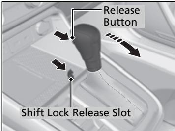
5. Insert the built-in key into the shift lock release slot.
