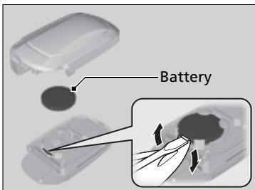
3. Remove the battery by prying on the edge with flat-tip screwdriver. Make sure to replace the battery with the correct polarity.
