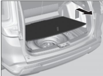
2. Pull the strap upwards to lift the floor lid.
