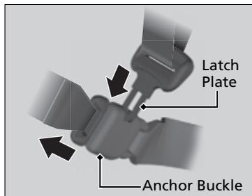
1. Store the center seat belt first. Insert the latch plate into the slot on the side of the anchor buckle.
