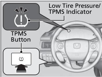
Press and hold the TPMS button until the low tire pressure/TPMS indicator blinks twice, indicating the calibration process has begun.
