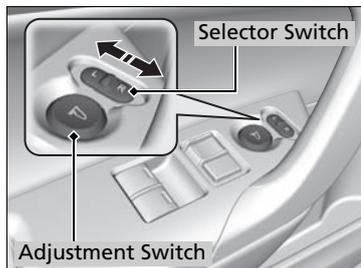
You can adjust the door mirrors when the ignition switch is in ON
