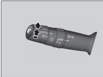
Automatic lighting control can be used when the ignition switch is in ON
