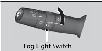
When the low beam headlights are on, turn the fog light switch on to use the fog lights.
