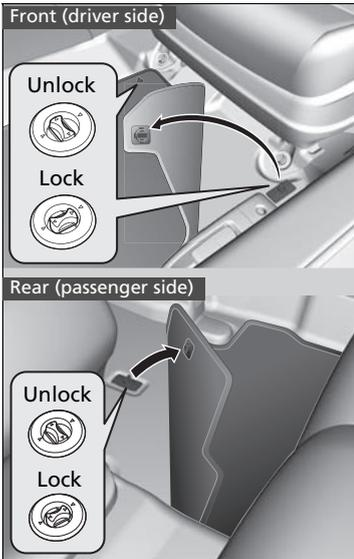
The floor mats for the driver, and the rear passenger on the passenger's side hook over the floor anchors, which keep the mats from sliding forward. To remove a mat for cleaning, turn the anchor knobs to the unlock position. When reinstalling the mat after cleaning, turn the knobs to the lock position.
