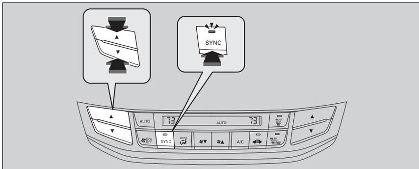
You can set the temperature synchronously for the driver side and the passenger side in synchronized mode.
