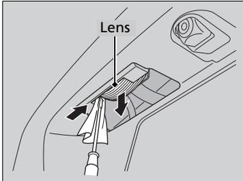
1. Remove the lens by carefully prying on its left edge with a small flat-tip screwdriver.
