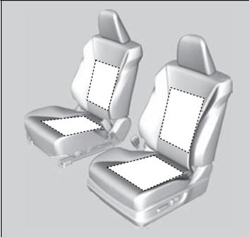
The ignition switch must be in ON **II**\*1 to use the seat heaters. The **HI** setting heats the seats faster than the **LO** setting.
