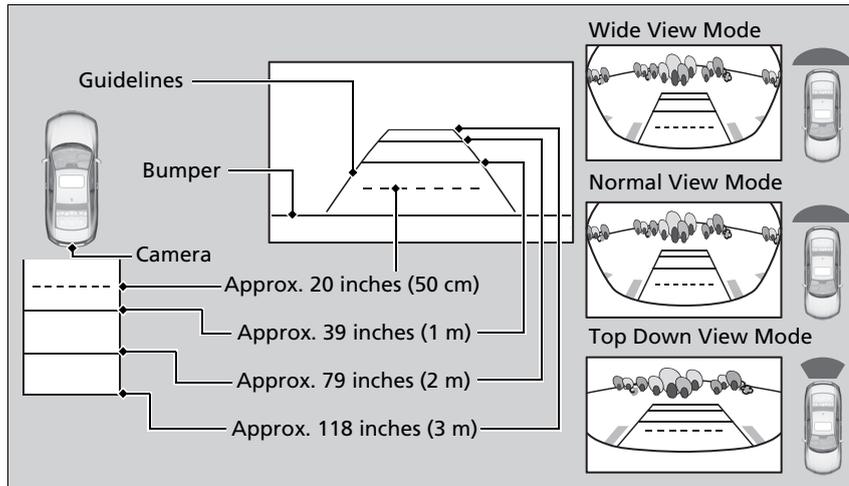
You can view three different camera angles on the rearview display. Press the selector knob or the interface dial to switch the angle.
