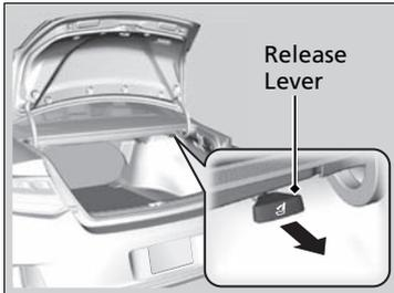
2. Pull the release lever in the trunk to release the lock.
