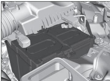
Check the battery terminals for corrosion monthly.
