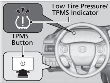
Press and hold the TPMS button until the low tire pressure/TPMS indicator blinks twice, indicating the calibration process has begun.
