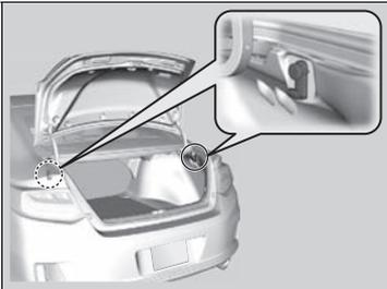
The cargo hooks in the trunk can be used to install a net for securing items.
