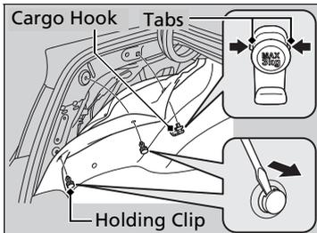
1. Remove the cargo hook by squeezing the tabs on both sides.
