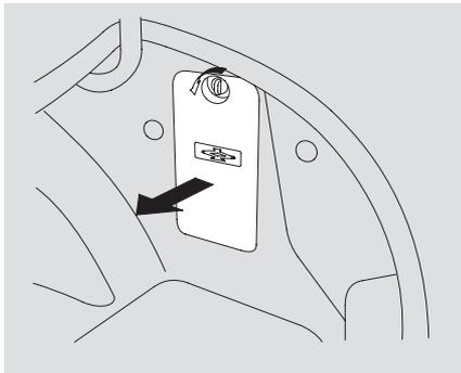
6. The jack is behind a cover in the right fender. Remove the cover by turning the handle counterclockwise, then pulling on the cover.
