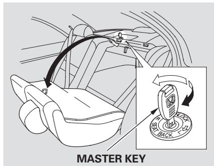
The left and right halves of the rear seat can be folded separately from inside the vehicle or inside the trunk. To fold down the seat-back from inside the vehicle, insert the master key in the lock on the rear shelf. To fold down the driver's side, turn the key clockwise, pull down the top of the seat-back, then release the key. To fold down the passenger's side, turn the key counterclockwise and perform the same procedure.
