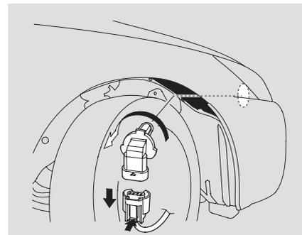
5. Remove the electrical connector from the bulb by squeezing the connector to unlock the tab, then slide the connector off the bulb.
