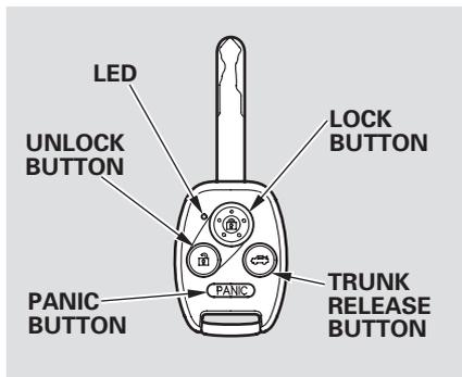
**LOCK** — Press this button once to lock both doors. Some exterior lights will flash once. When you push LOCK twice within 5 seconds, you will hear a beep to verify that the doors are locked and (if equipped) that the security system has set. You cannot lock the doors if either door is not fully closed or the key is in the ignition switch.
