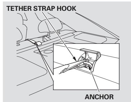
1. After properly securing the child seat (see page 42), route the tether strap over the seat-back.
