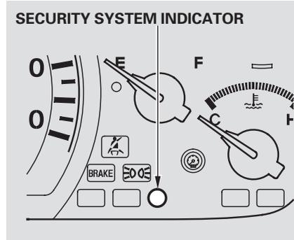
Once the security system is set, opening either door without using the key or the remote transmitter, the hood, or the trunk will cause the system to alarm. It also alarms if the radio is removed from the dashboard or the wiring is cut.
