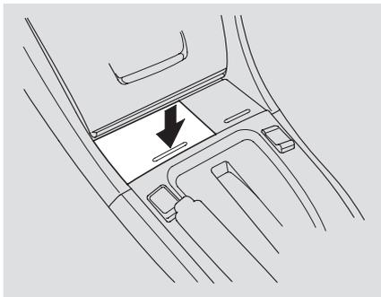
To open the coin pocket, push the top of the lid. To close it, push the lid down until it latches. The compartment cannot be used as an ashtray.
