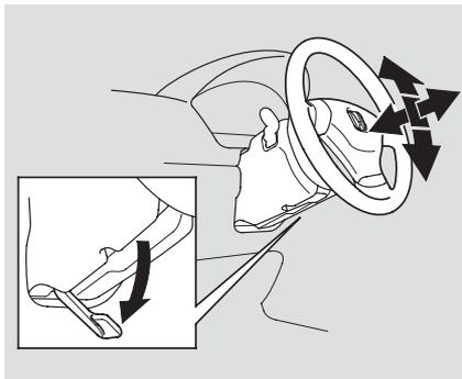
1. Insert the key in the ignition switch, and unlock the steering column.
