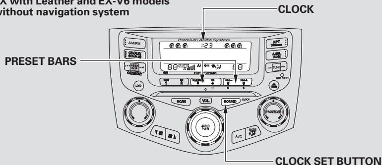
the displayed time is after the half hour, the clock sets forward to the beginning of the next hour.
