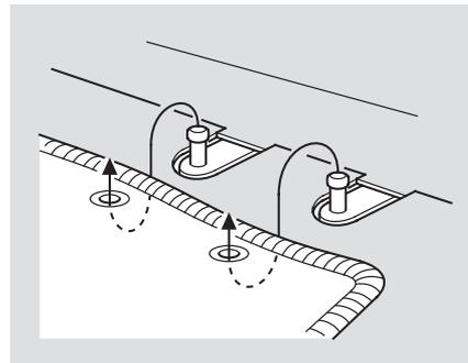
The driver's and the right-rear passenger's floor mats that came with your vehicle hook over the floor mat anchors. This keeps the floor mat from sliding forward and possibly interfering with the pedals or making the front passenger's weight sensors ineffective.
