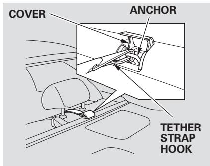
2. Lift the cover, then attach the tether strap hook to the anchor, making sure the strap is not twisted.
