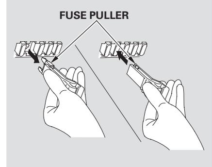
4. Check the smaller fuses in the under-hood fuse box and all the fuses in the interior fuse box by pulling out each one with the fuse puller provided in the under-hood fuse box.
