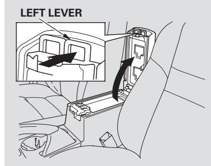
You can put small items in the tray located in the console compartment lid. To use the tray, pull up on the left lever and lift the armrest.
