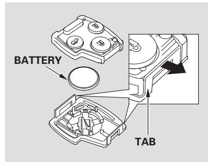
2. Separate the transmitter by prying its middle seam with your fingernail.
