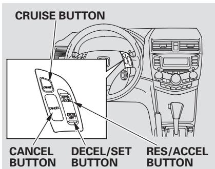
1. Push in the CRUISE button on the steering wheel. The CRUISE MAIN indicator on the instrument panel will come on.
