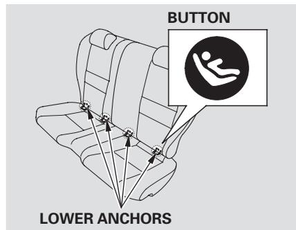
Your vehicle is equipped with LATCH (Lower Anchors and Tethers for Children) at the outer rear seats.
