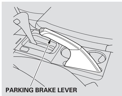
To apply the parking brake, pull the lever up fully. To release it, pull up slightly, push the button, and lower the lever. The parking brake indicator on the instrument panel should go out when the parking brake is fully released with the engine running (see page 57).
