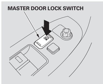
To lock the doors, push the top of the master door lock switch on either door, press the lock tab down on the driver's door, or use the key on the outside lock on the driver's door.
