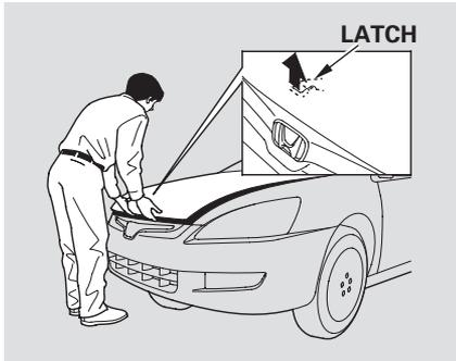
2. Reach in between the hood and the front grille with your finger. The hood latch handle is above and to the left of the “H” logo. Push this handle up until it releases the hood. Lift the hood.
