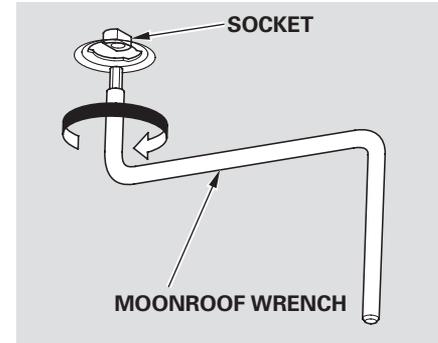
6. Remove the wrench. Reinstall the round plug.
