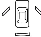
The appropriate indicator comes on in this monitor if the trunk or either door is not closed tightly.
