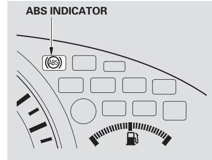
If the ABS indicator comes on, the anti-lock function of the braking system has shut down. The brakes still work like a conventional system, but without anti-lock. You should have your dealer inspect your vehicle as soon as possible.
