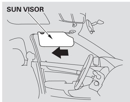
In this position, the sun visor can be adjusted by moving it on its slider. Do not use the sun visor extension over the inside mirror.
