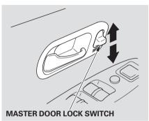
The master door lock switch on the driver's door locks and unlocks all of the doors and tailgate. Push the switch down to lock all of the doors and the tailgate, and up to unlock them.
