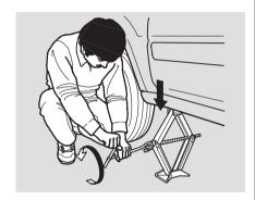
21.Lower the vehicle to the ground and remove the jack.
