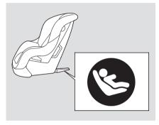
This symbol on rear or forward facing child seats or booster cushions indicates the presence of LATCH compatible hardware.
