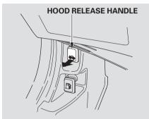
1. Shift to Park or Neutral and set. the parking brake. Pull the hood release handle located under the lower left corner of the dashboard. The hood will pop up slightly.
