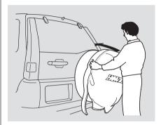
29. Hold the cover at the 10 o'clock and 2 o'clock positions, then place the top of it over the spare tire.
