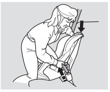
5. After confirming that the belt is locked, grab the shoulder part of the belt near the buckle and pull up to remove any slack from the lap part of the belt. Remember, if the lap part of the belt is not tight, the child seat will not be secure. It may help to put weight on the child seat, or push on the back of the seat, while pulling up on the belt.
