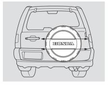
36.Make sure the cover is horizontal. If needed, pivot the cover until the cover is horizontal.
