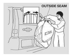
31.Starting at the top of the tire, position the outside seam of the cover slightly over the outside edge of the tire. Pull the cover on, a little at a time, and alternate side to side along the tire until you reach the bottom.
