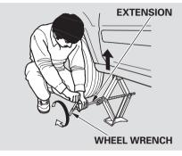
17.Use the extension and wheel wrench as shown to raise the vehicle until the flat tire is off the ground.
