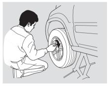
20.Put on the spare tire. Put the wheel nuts back on finger-tight, then tighten them in a crisscross pattern with the wheel wrench until the wheel is firmly against the hub. Do not try to tighten them fully.
