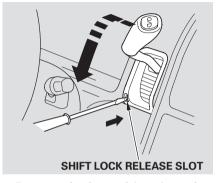
6. Remove the Screwdriver from the Shift Lock Release slot, then install a new cover. Make sure the notch on the cover is on the right side. Depress the brake pedal and restart the engine.
