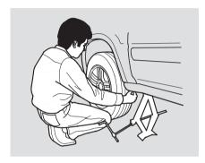
18. Remove the wheel nuts, then remove the flat tire. Temporarily place the flat tire on the ground with the outside surface of the wheel facing up. You could scratch the wheel if you put it face down.
