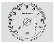
This indicator on the instrument. panel shows which position the shift lever is in
