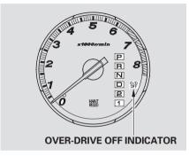
Pressing the O/D switch again turns the Over-drive mode back on.
