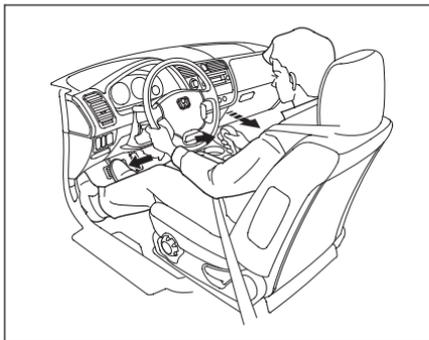
**Park (P)** – This position mechanically locks the transmission. Use Park whenever you are turning off or starting the engine. To shift out of Park, you must press on the brake pedal, have your foot off the accelerator pedal, and press the release button on the front of the shift lever.
