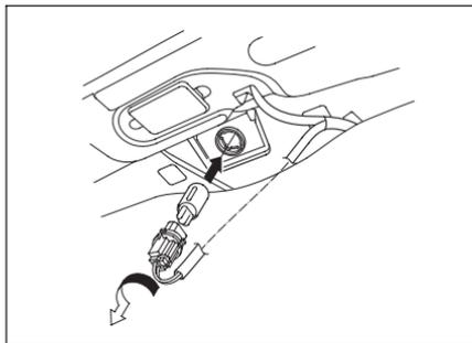
4. Remove the socket from the light assembly by turning it one-quarter turn counterclockwise.
