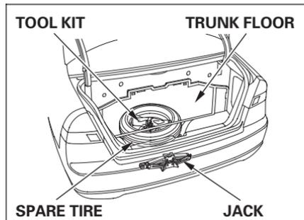
The spare tire is stored in the trunk. To remove the spare tire and the tool kit, open the trunk and raise the trunk floor by lifting up on the back edge.
