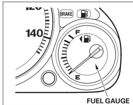
This gauge shows how much fuel you have. The quantity of fuel remaining in the tank is calculated based on the pressure and temperature of the natural gas in the fuel tank.
