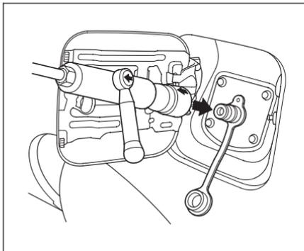
5. Securely connect the CNG fill nozzle to the fuel receptacle by turning the lever until the arrows on the nozzle point to each other.
