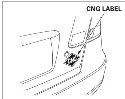
Your vehicle has an identifying “CNG” label attached next to the rear license plate. Do not remove this label. This label is necessary for insuring your vehicle. Driving without this label may violate the laws or regulations in some states.
