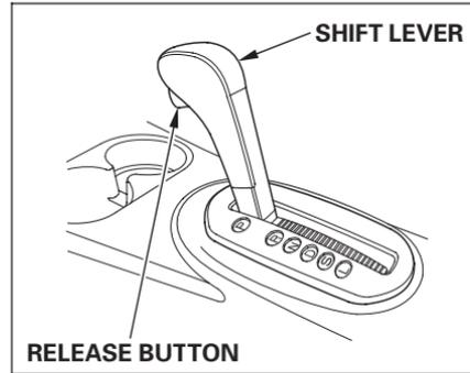
The shift lever has six positions. It must be in Park or Neutral to start the engine. When you are stopped in D, S, L, N or R, press firmly on the brake pedal and keep your foot off the accelerator pedal.
