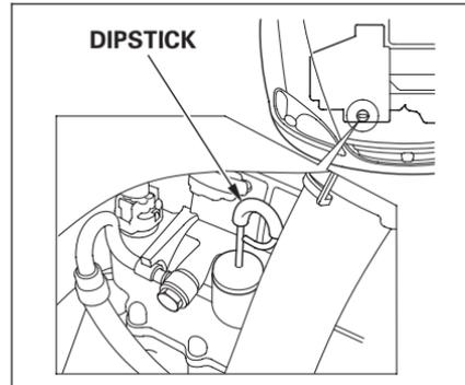
1. Park the car on level ground. Shut off the engine. For accurate results, wait at least 60 seconds, and no more than 90 seconds, after shutting off the engine to check the fluid level.
