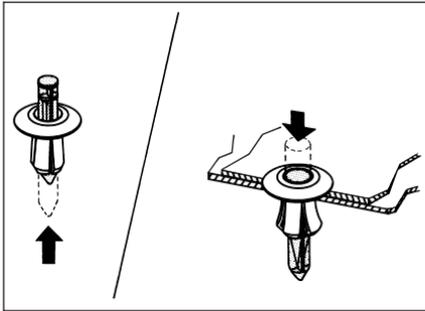
10. Reset each fastener by pushing on its pointed end until it pops back almost flush with the fingers on the housing.
