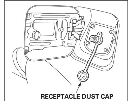
4. Remove the receptacle dust cap from the fuel receptacle. Clean up any dirt and debris around the fuel receptacle.
