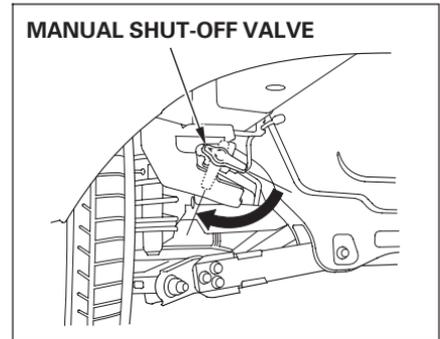
A manual shut-off valve is located underneath the vehicle, near the rear tire on the driver's side. We recommend that you locate this valve so you can find it quickly.
