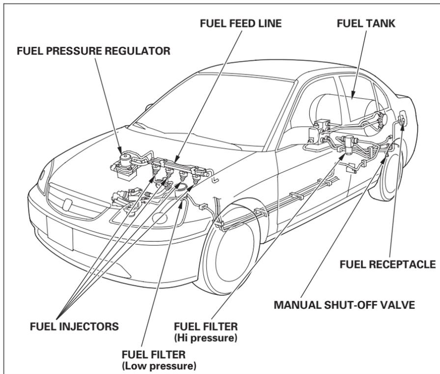
Fuel system components include a fuel tank located in the trunk, an integrated fuel pressure regulator, an in-tank fuel shut-off valve, fuel high pressure lines, electronically controlled multipoint fuel injectors and other equipment.
