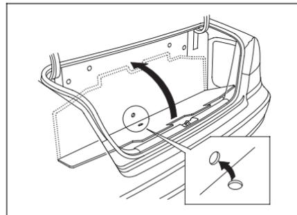
1. Raise the trunk floor and the lower part of the trunk lining as shown. Align the lower hole in the trunk lining with the hole in the trunk floor.
