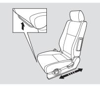
To adjust the seat forward and backward, pull up on the bar under the seat cushion's front edge. Try to move the seat to make sure it is locked in position.
