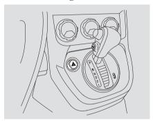
Push the button next to the shift lever to turn on the hazard warning lights (four-way flashers). This causes all four outside turn signals and both turn indicators in the instrument panel to flash. Use the hazard warning lights if you need to park in a dangerous area near heavy traffic, or if your vehicle is disabled.
