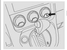
The rear window defogger will clear fog, frost, and thin ice from the window. Push the defogger button to turn it on and off. The indicator in the button comes on to show the defogger is on. If you do not turn it off, the defogger will shut itself off after about 15 minutes. It also shuts off when you turn off the ignition switch. You have to turn the defogger on again when you restart the vehicle.
