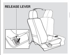
The rear seat passengers can get out through the passenger's door. Push down on the release lever at the base of the front passenger's seat-back, and push the seat-back forward. The seat-back will tilt forward and the entire seat will move forward.
