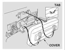
2. Remove the cover between the seat cushion and the side wall by pulling the tab and pulling the cover straight up.
