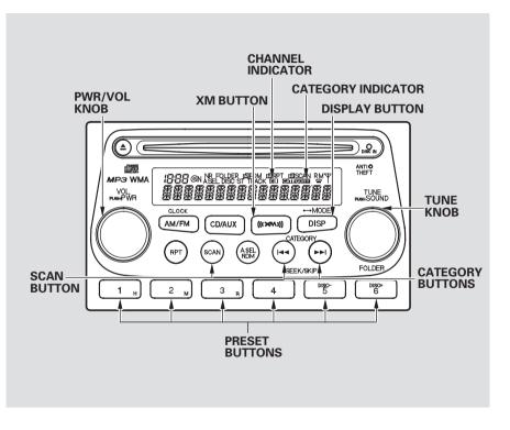
**To Play XM® Satellite Radio** To listen to XM radio, turn the ignition switch to ACCESSORY (I) or ON (II). Push the PWR/VOL knob to turn on the audio system, and press the "XM" button. Adjust the volume by turning the PWR/ VOL knob. The last channel you listened to will show in the display.
