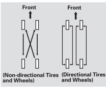
To help increase tire life and distribute wear more evenly, rotate the tires every 10,000 miles (16,000 km). Move the tires to the positions shown in the chart each time they are rotated. If you purchase directional tires, rotate only front-toback. **Replacing Tires and Wheels** Replace your tires with radial tires of the same size, load range, speed rating, and maximum cold tire pressure rating (as shown on the tire's sidewall).
