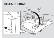
3. Pull the release strap on the seat support, and pivot the seat toward the vehicle's side wall.
