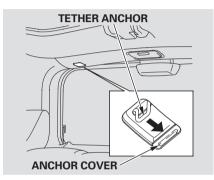
1. After securing the child seat in the desired position (see page 41), remove the head restraint, then route the tether strap over the top of the seat-back
