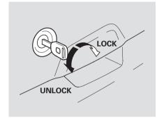
To lock or unlock the hatch.
