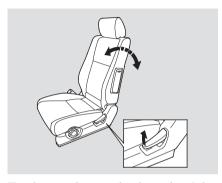
To change the seat-back angle of the front seat, pull up on the lever on the outside of the seat bottom. Adjust the seat-back and make sure it locks into position.
