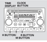
Press and hold the CLOCK button until the numbers flash and you hear a beep. Change the hour by pressing the H button until the numbers advance to the desired time. Change the minute by pressing the M button until the numbers advance to the desired time.
