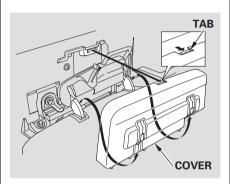
2. Remove the cover between the seat cushion and the side wall by pulling the tab and pulling the cover straight up.
