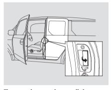
To open the rear door, pull the rear door handle located in the rear door edge. The rear door can be opened only when the front door is open.
