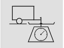
Tongue Load: The weight that the tongue of a fully-loaded trailer puts on the hitch should be approximately 10 percent of the total trailer weight. Too much tongue load reduces front-tire traction and steering control. Too little tongue load can make the trailer unstable and cause it to sway.
