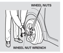
8. Loosen the five wheel nuts 1/2 turn with the wheel nut wrench.
