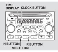
You can quickly set the time to the nearest hour. If the displayed time is before the half hour, press the R (RESET) button to set the clock back to the previous hour. If the displayed time is after the half hour, pressing R sets the clock forward to the beginning of the next hour. For example: 1:06 will reset to 1:00 1:53 will reset to 2:00
