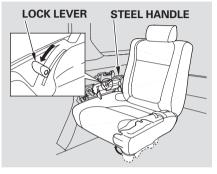
3. Push the lock lever forward to unlock the seat.
