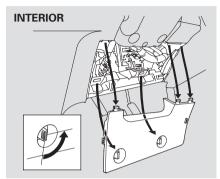
The interior fuse box is underneath the steering column. To remove the fuse box lid, turn the knobs counterclockwise and pull the lid out of its hinges.
