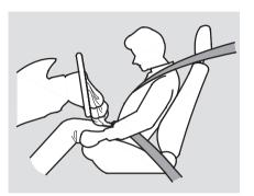
After inflating, the front airbags immediately deflate, so they won't interfere with the driver's visibility, or the ability to steer or operate other controls. The total time for inflation and deflation is one-tenth of a second, so fast that most occupants are not aware that the airbags deployed until they see them lying in their laps.
