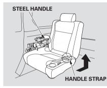
4. Hold the steel handle next to the lock lever and the handle strap at the outside edge of the seat cushion, and remove the entire seat by pulling it up and backward. Reverse this procedure to reinstall the seat. Make sure the seat is securely locked.
