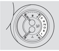
These indicators on the instrument panel show which position the shift lever is in.
