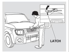
If the hood latch handle moves stiffly, or if you can open the hood without lifting the handle, the mechanism should be cleaned and lubricated.
