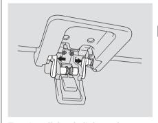
To reinstall the skylight, make sure the air deflector is pushed down. When reinstalling the lever assembly, push in both red pivots, and align with the receptacle holes. Let the pivots move out until they rest in the holes securely. Make sure the skylight is fully closed and latched.
