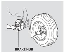
12. Before mounting the spare tire, wipe any dirt off the mounting surface of the wheel and hub with a clean cloth. Wipe the hub carefully; it may be hot from driving.
