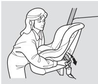
1. With the child seat in the desired seating position, route the belt through the child seat according to the seat maker's instructions, then insert the latch plate into the buckle.
