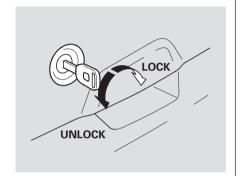
To lock or unlock the hatch.
