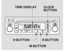
You can use the R button to quickly set the time to the nearest hour. Press the R button while pressing the CLOCK button. If the displayed time is before the half hour, pressing R sets the clock back to the previous hour. If the displayed time is after the half hour, pressing R sets the clock forward to the beginning of the next hour. For example: 1:06 will reset to 1:00 1:53 will reset to 2:00
