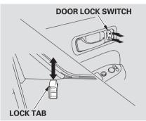
To lock all of the doors and hatch, press the door lock switch on either front door, or press the lock tab down on the driver's door, or use the key on the outside lock. Pressing up on the door lock switch will unlock all of the doors and the hatch.
