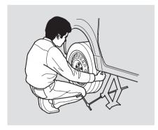
11. Remove the wheel nuts and the flat tire. Temporarily place the flat tire on the ground with the outside surface of the wheel facing up.
