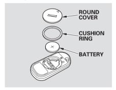
If it takes several pushes on the button to lock or unlock the doors and the hatch, replace the battery as soon as possible. Battery type: CR2025 To replace the battery, remove the round cover on the back of the transmitter by turning it counterclockwise with a coin. Insert a new battery with the + side facing up, and reinstall the cushion ring. Align the  $\bigtriangledown$  mark on the cover with the  $\bigcirc$  mark on the transmitter. Set the cover in place and turn it clockwise.
