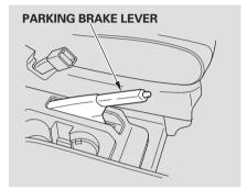
To apply the parking brake, pull the lever up fully. To release it, pull up slightly, push the button, and lower the lever. The parking brake indicator on the instrument panel should go out when the parking brake is fully released (see page 54).
