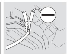
4. Connect the second jumper cable to the negative (-) terminal on the booster battery. Connect the other end to the grounding strap on your vehicle as shown. Do not connect this jumper cable to any other part of the engine.
