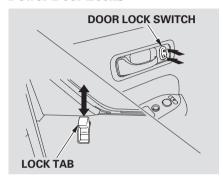
To lock all of the doors and hatch, press the door lock switch on either front door, or press the lock tab down on the driver's door, or use the key on the outside lock.
