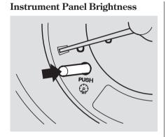
Push the button in the speedometer repeatedly to adjust the brightness of the instrument panel lights. There are six brightness levels. A segment display shows the current brightness level. Hazard Warning Button
