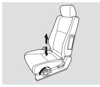
To adjust the height of the driver's seat, turn the dial on the outside of the seat bottom.
