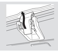
*On 4WD models only* To lift up the rear of the skylight for ventilation, pull down the lever to unlock the skylight, then push it up until the skylight is locked in the tiltup position.
