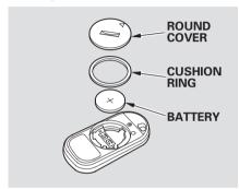
If it takes several pushes on the button to lock or unlock the doors and the hatch, replace the battery as soon as possible.
