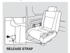
Both seats can be removed to give more cargo capacity. To remove a seat:
