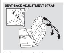
To change the angle of the rear seatback, pull the strap at the inside edge of the seat cushion, make sure the seat-back locks into position.
