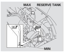
Look at the coolant level in the radiator reserve tank. Make sure it is between the MAX and MIN lines. If it is below the MIN line, see **Adding Engine Coolant** on page 173 for information on adding the proper coolant.
