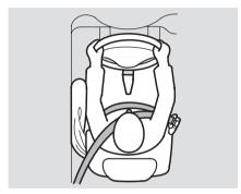
If you ever have a moderate to severe side impact, sensors will detect rapid deceleration and signal the control unit to instantly inflate either the driver's or the passenger's side airbag.
