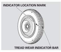
Replace the tire when you can see the tread wear indicator bars. The replacement should be the same size and design tire, mounted on the same wheel. The spare tire is not designed to be mounted on a regular wheel, and the spare wheel is not designed for mounting a regular tire. If you have a flat tire while driving, stop in a safe place to change it. Drive slowly along the shoulder until you get to an exit or an area to stop that is far away from the traffic lanes.
