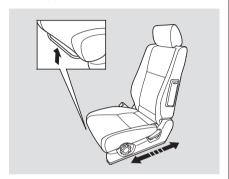
To adjust the seat forward and backward, pull up on the bar under the seat cushion's front edge. Try to move the seat to make sure it is locked in position.
