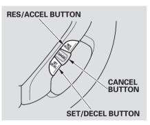
Cruise control may not hold the set speed when you are going up and down hills. If your speed increases going down a hill, use the brakes to slow down. This will cancel cruise control. To resume the set speed, press the RES/ACCEL button. The indicator on the instrument panel will come back on. Features
