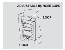
The driver's seat-back and left rear seat-back are equipped with adjustable bungee cords to hold medium-sized, lightweight objects.
