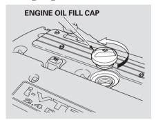
Unscrew and remove the engine oil fill cap on top of the valve cover. Pour in the oil slowly and carefully so you do not spill. Clean up any spills immediately. Spilled oil could damage components in the engine compartment. Install the engine oil fill cap, and tighten it securely. Wait a few minutes, and recheck the oil level. Do not fill above the upper mark; you could damage the engine.
