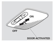
The ceiling light has a three-position switch: ON, Door Activated, and OFF.
