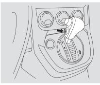
Overdrive (O/D) is on whenever you turn the ignition to ON (II). Press the O/D switch on the side of the shift lever to turn it off; the O/D OFF indicator comes on.
