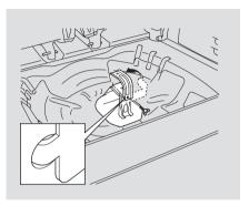
18.Remove the wing bolt on the spare tire mount, and pivot the arm 90° to the upright position. Then tighten the wing bolt securely.
