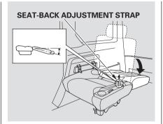
2. Pull the seat-back adjustment strap at the inside edge of the seat cushion and push the seat-back backward as far as it will go.
