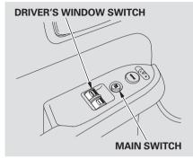
Turn the ignition switch to ON (II) to raise or lower either window. To open the window, push the switch down and hold it. Release the switch when you want the window to stop. Pull back on the switch and hold it to close the window.
