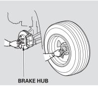
12. Before mounting the spare tire, wipe any dirt off the mounting surface of the wheel and hub with a clean cloth. Wipe the hub carefully; it may be hot from driving. 13. Put on the spare tire. Put the wheel nuts back on finger-tight, then tighten them in a crisscross pattern with the wheel nut wrench until the wheel is firmly against the hub. Do not try to tighten them fully.
