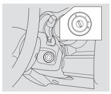
The ignition switch has four positions: LOCK (0), ACCESSORY (I), ON (II), and START (III).
