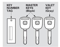
The master key fits all the locks on your vehicle. The valet key works only in the ignition and the door locks. You can keep the glove box and hatch locked when you leave your vehicle and the valet key at a parking facility.
