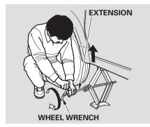
10.Use the extension and the wheel nut wrench as shown to raise the vehicle until the flat tire is off the ground.
