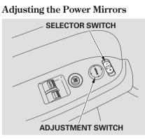
1. Move the selector switch to L (driver's side) or R (passenger's side).
