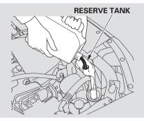
If the coolant level in the reserve tank is at or below the MIN line, add coolant to bring it up to between the MIN and MAX lines. Inspect the cooling system for leaks. Always use Honda All Season Antifreeze/Coolant Type 2. This coolant is pre-mixed with 50 percent antifreeze and 50 percent water. Never add straight antifreeze or plain water.
