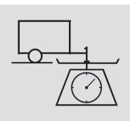
**Tongue Load:** The weight that the tongue of a fully-loaded trailer puts on the hitch should be approximately 10 percent of the total trailer weight. Too much tongue load reduces front-tire traction and steering control. Too little tongue load can make the trailer unstable and cause it to sway.
