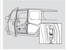
To open the rear door, pull the rear door handle located in the rear door edge. The rear door can be opened only when the front door is open.
