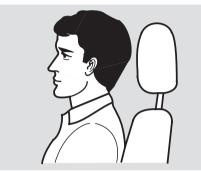
Adjust the driver's head restraint so the back of your head rests against the center of the restraint.
