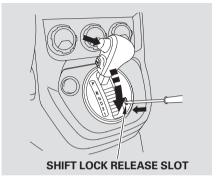
6. Remove the screwdriver from the shift lock release slot, then replace the cover. Make sure the notch on the cover is on the right side. Press the brake pedal and restart the engine.
