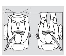
Standard on EX models Your vehicle also has side airbags to help protect the upper torso of the driver or a front seat passenger during a moderate to severe side impact (see page 26 for more information on how your side airbags work).
