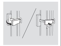
To open a rear window, pull the lever towards you, then push it out until it locks. To close the rear window pull the lever towards you, then push it back. Make sure the window is fully closed and locked
