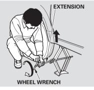
10.Use the extension and the wheel nut wrench as shown to raise the vehicle until the flat tire is off the ground.
