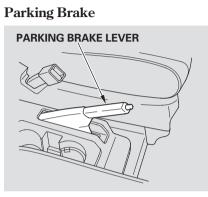
To apply the parking brake, pull the lever up fully. To release it, pull up slightly, push the button, and lower the lever. The parking brake indicator on the instrument panel should go out when the parking brake is fully released (see page 54).
