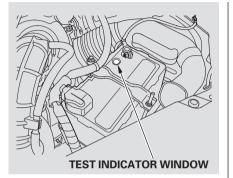
Check the condition of the battery monthly by looking at the test indicator window. The label on the battery explains the test indicator's colors. Check the terminals for corrosion (a white or yellowish powder). To remove it, cover the terminals with a solution of baking soda and water. It will bubble up and turn brown. When this stops, wash it off with plain water. Dry off the battery with a cloth or paper towel. Coat the terminals with grease to help prevent future corrosion.
