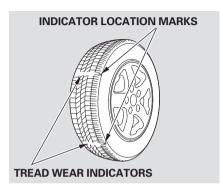
Your tires have wear indicators molded into the tread. When the tread wears down, you will see a band 1/2 inch (12.7 mm) wide across the tread. This shows there is less than 1/16 inch (1.6 mm) of tread left on the tire. A tire that is this worn gives very little traction on wet roads. You should replace the tire if you can see the tread wear indicator in three or more places on the tire.
