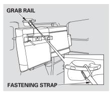
4. A fastening strap is attached to the inside of the seat cushion. While pushing the seat up and toward the side wall, hook the fastening strap to the grab rail.
