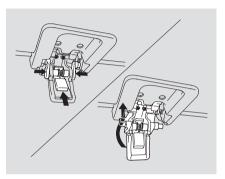
*To remove the skylight:* Turn off the engine, and set the parking brake. Then pull down the lever, squeeze both sides of the pivot while pushing up the red tab in the lever, and pull the lever assembly away from the ceiling.
