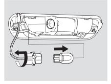
3. Pull the bulb straight out of its socket. Push the new bulb straight into the socket until it bottoms.
