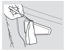
1. Place a cloth between the trim of the lens and the body, at the top of the lens. Remove the front side marker light assembly by carefully prying on the trim of the lens with a small flat-tipped screwdriver.
