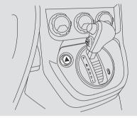
Push the button next to the shift lever to turn on the hazard warning lights (four-way flashers). This causes all four outside turn signals and both turn indicators in the instrument panel to flash. Use the hazard warning lights if you need to park in a dangerous area near heavy traffic, or if your vehicle is disabled. **Rear Window Defogger**
