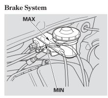
The fluid level should be between the MIN and MAX marks on the side of the reservoir. If the level is at or below the MIN mark, your brake system needs attention. Have the brake system inspected for leaks or worn brake pads.
