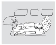
You can recline the seat-backs on the front seats so they are level with the rear seat cushions, making a large cushioned area. To do this:
