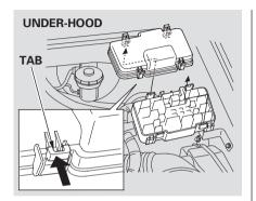
The vehicle's fuses are located in two fuse boxes. The under-hood fuse box is located in the engine compartment on the driver's side. To open it, push the tabs as shown.
