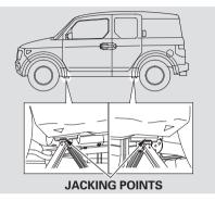
9. Locate the jacking point nearest the tire you need to change. It is pointed to by an arrow molded into the underside of the body. Place the jack under the jacking point. Turn the end bracket clockwise until the top of the jack contacts the jacking point. Make sure the jacking point tab is resting in the jack notch.
