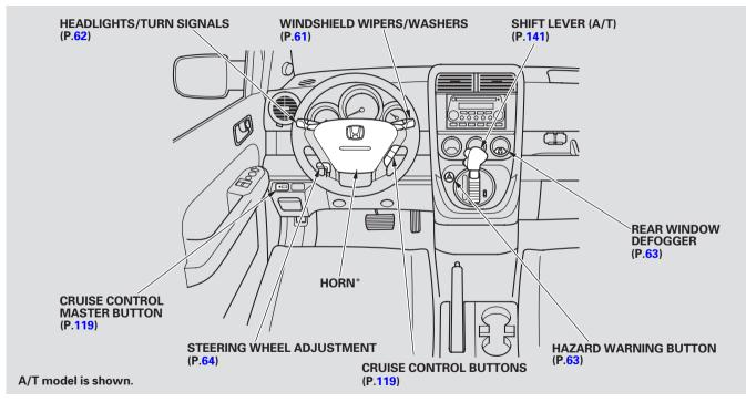
\*: To use the horn, press the center pad of the steering wheel.
