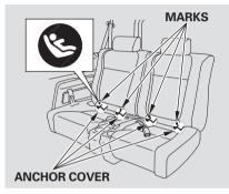
Your vehicle is equipped with LATCH (Lower Anchors and Tethers for Children) at the second row seats. The lower anchors are located between the seat-back and seat bottom, and are to be used only with a child seat designed for use with LATCH.
