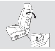
To change the seat-back angle of the front seat, pull up on the lever on the outside of the seat bottom. Adjust the seat-back and make sure it locks into position. Driver's Seat Height Adjustment
