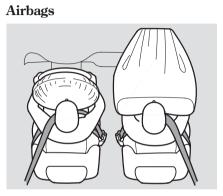
Your vehicle has a supplemental restraint system (SRS) with front airbags to help protect the heads and chests of the driver and a front seat. passenger during a moderate to severe frontal collision (see page 24 for more information on how your front airbags work).
