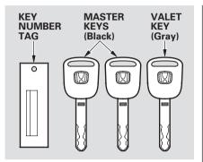
The master key fits all the locks on your vehicle. The valet key works only in the ignition and the door locks. You can keep the glove box and hatch locked when you leave your vehicle and the valet key at a parking facility.
