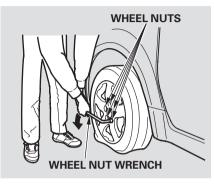
8. Loosen the five wheel nuts 1/2 turn with the wheel nut wrench.
