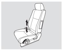
To adjust the height of the driver's seat, turn the dial on the outside of the seat bottom.
