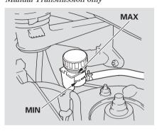
The fluid level should be between the MIN and MAX marks on the side of the reservoir. If it is not, add brake fluid to bring it up to that level. Use the same fluid specified for the brake system.
