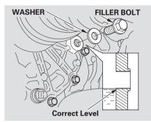
Check the fluid level with the transmission at normal operating temperature and the vehicle sitting on level ground. Remove the transmission filler bolt, and carefully feel inside the bolt hole with your finger. The fluid level should be up to the edge of the bolt hole. If it is not, add Honda manual transmission fluid (MTF) until it starts to run out of the hole. Reinstall the filler bolt, and tighten it securely.
