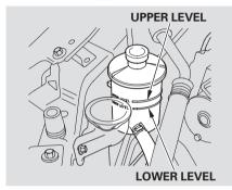
Check the level on the side of the reservoir when the engine is cold. The fluid should be between the UPPER LEVEL and LOWER LEVEL. If not, add power steering fluid to the UPPER LEVEL.
