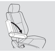
*On EX models* Each front seat has an armrest on the side of the seat-back. To use it, pivot it down. Rear Seat
