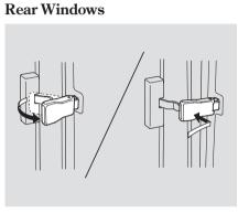
To open a rear window, pull the lever towards you, then push it out until it locks. To close the rear window pull the lever towards you, then push it back. Make sure the window is fully closed and locked.
