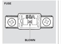
3. Check each of the large fuses in the under-hood fuse box by looking through the top at the wire inside. Remove the screws with a Phillips-head screwdriver.
