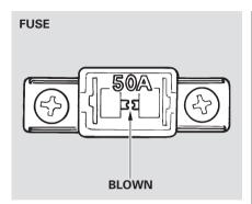
3. Check each of the large fuses in the under-hood fuse box by looking through the top at the wire inside. Remove the screws with a Phillips-head screwdriver.
