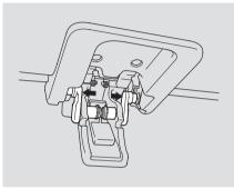
To reinstall the skylight, make sure the air deflector is pushed down. When reinstalling the lever assembly, push in both red pivots, and align with the receptacle holes. Let the pivots move out until they rest in the holes securely. Make sure the skylight is fully closed and latched.
