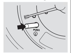
Push the button in the speedometer repeatedly to adjust the brightness of the instrument panel lights. There are six brightness levels. A segment display shows the current brightness level.
