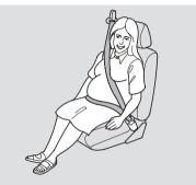
If you are pregnant, the best way to protect yourself and your unborn child when driving or riding in a vehicle is to always wear a seat belt, and keep the lap part of the belt as low as possible across the hips. When driving, remember to sit upright and adjust the seat as far back as possible while allowing full control of the vehicle. When riding as a front passenger, adjust the seat as far back as possible.
