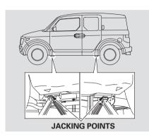
9. Locate the jacking point nearest the tire you need to change. It is pointed to by an arrow molded into the underside of the body. Place the jack under the jacking point. Turn the end bracket clockwise until the top of the jack contacts the jacking point. Make sure the jacking point tab is resting in the jack notch.
