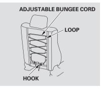
The driver's seat-back and left rear seat-back are equipped with adjustable bungee cords to hold medium-sized, lightweight objects. If the cords are not installed, route one cord through the loops as shown. To attach the hooks, press the top of the hook down, and slide to the desired position, then release. Adjust as needed.
