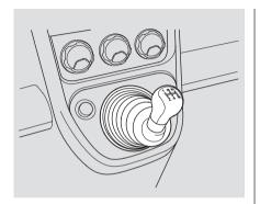
The manual transmission is synchronized in all forward gears for smooth operation. It has a lockout so you cannot shift directly from fifth to reverse. When shifting up or down, make sure you push the clutch pedal down all the way, shift to the next gear, and let the pedal up gradually. When you are not shifting, do not rest your foot on the clutch pedal. This can cause your clutch to wear out faster.
