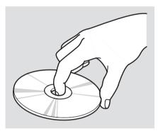
Handle a disc by its edges; never touch either surface. Do not place stabilizer rings or labels on the disc. These, along with contamination from finger prints, liquids, and felttip pens, can cause the disc to not play properly, or possibly jam in the drive. If you see an error message in the display while playing a disc, find the cause in the chart to the right. If you cannot clear the error message, take the vehicle to your dealer.
