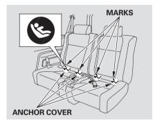
Your vehicle is equipped with LATCH (Lower Anchors and Tethers for Children) at the second row seats. The lower anchors are located between the seat-back and seat bottom, and are to be used only with a child seat designed for use with LATCH.
