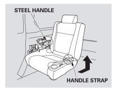
4. Hold the steel handle next to the lock lever and the handle strap at the outside edge of the seat cushion, and remove the entire seat by pulling it up and backward.
