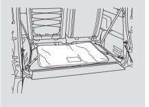
With the rear seats in their upright position, store the skylight, face down in its bag in the cargo area. Secure the bag with four hooks on the cargo area floor. Do not store anything on top of the skylight.
