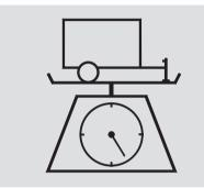
Total Trailer Weight: The maximum allowable weight of the trailer and everything in or on it must not exceed 1,500 lbs (680 kg). Towing a load that is too heavy can seriously affect your vehicle's handling and performance. It can also damage the engine and drivetrain.
