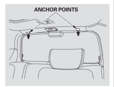
A child seat with a tether can be installed in either seating position in the back seat, using one of the anchorage points shown above.
