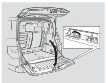
See page 130 for information on cargo loading. Keep the tailgate and the hatch closed at all times while driving to avoid damaging them, and to prevent exhaust gas from getting into the interior. See **Carbon Monoxide Hazard** on page 47.
