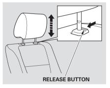
Your vehicle is equipped with head restraints in all seating positions to help protect you and your passengers from whiplash and other injuries. They are most effective when you adjust them so the back of the occupant's head rests against the center of the restraint.
