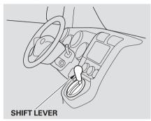
To shift from any position, press firmly on the brake pedal, push the release button, and pull the lever toward you. You cannot shift out of Park when the ignition switch is in the LOCK (0) or ACCESSORY (I) position.
