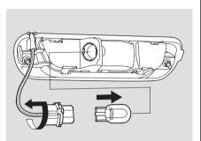
3. Pull the bulb straight out of its socket. Push the new bulb straight into the socket until it bottoms.
