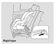
Place the child seat on the vehicle seat, then attach the seat to the lower anchors according to the child seat maker's instructions.
