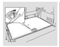
5. Push the rear edge of the handle to raise the handle loop and pull up the loop to raise the cargo area floor.
