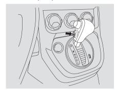
Overdrive (O/D) is on whenever you turn the ignition to ON (II). Press the O/D switch on the side of the shift lever to turn it off; the O/D OFF indicator comes on.
