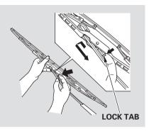
2. Disconnect the blade assembly from the wiper arm by pushing in the lock tab. Hold the lock tab in while you push the blade assembly toward the base of the arm.
