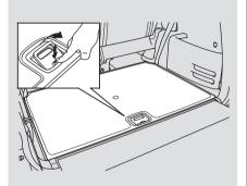
5. Push the rear edge of the handle to raise the handle loop and pull up the loop to raise the cargo area floor.
