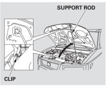
3. Pull the support rod out of its clip and insert the end into the hole in the hood
