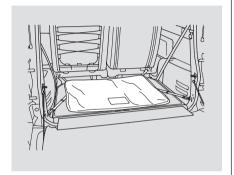
With the rear seats in their upright position, store the skylight, face down in its bag in the cargo area. Secure the bag with four hooks on the cargo area floor. Do not store anything on top of the skylight.
