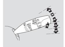
1. MIST 2. OFF 3. INT – Intermittent 4. LO – Low speed 5. HI – High speed 6. Windshield washers Push the right lever up or down to select a position.
