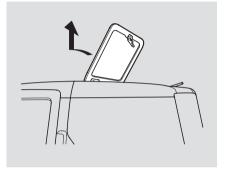
Push up the rear of the skylight. Standing on the tailgate with the hatch down, hold both sides of the skylight and pull it toward you to remove it from the vehicle roof.
