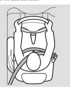
If you ever have a moderate to severe side impact, sensors will detect rapid deceleration and signal the control unit to instantly inflate either the driver's or the passenger's side airbag.
