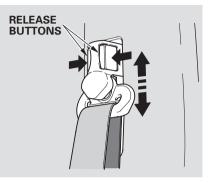
The front seats have adjustable seat belt anchors. To adjust the height of an anchor, press and hold the release buttons and slide the anchor up or down as needed (it has four positions). *Never place the shoulder portion of a lap/shoulder belt under your arm or behind your back.* This could cause very serious injuries in a crash.
