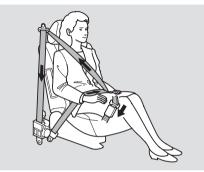
For added protection, the front seat belts are equipped with automatic seat belt tensioners. When activated, the tensioners immediately tighten the belts to help hold the driver and a front passenger in place. The tensioners are designed to activate primarily in frontal collisions, and they should activate in any collision severe enough to cause front-airbag inflation.
