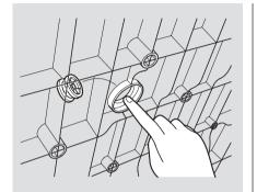
19.Remove the small round plug from the cargo area floor by pushing it from the back side to make a hole. Store the removed plug in a place you can easily remember.
