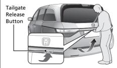
• To open the tailgate, push the tailgate release button, and lift up.
