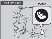
1. Locate the lower anchors under the marks.
