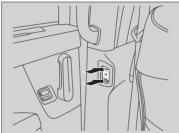
The power sliding door opens when you press the **OPEN** side of the [18] / [21] switch, and closes when you press the **CLOSE** side of the [18] / [21] switch.
