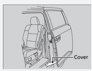
If you try to open the sliding door with the window open more than 3 inch (8 cm), the door stops halfway. Close the door, close the window, and then open the door again.
