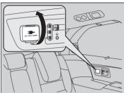
Open the cover to use it. Plug in the appliance slightly, turn it 90° clockwise, then push it all the way.
