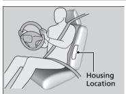
The side airbags are housed in the outside edge of the driver's and passenger's seat-backs.
