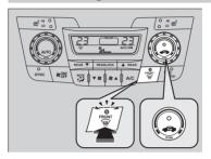
Pressing the button turns the air conditioner system on and automatically switches the system to fresh air mode.
