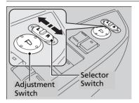
You can adjust the door mirrors when the ignition switch is in ON  $\boxed{\rm II}$ .
