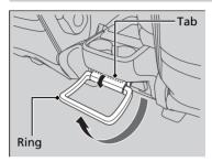
Pull up the ring until it clicks, and lift the tab. Put a plastic bag in the ring. Push the tab down to hold the bag.
