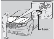
**3.** Slide the hood latch lever in the center of the hood to release the lock mechanism, and open the hood.
