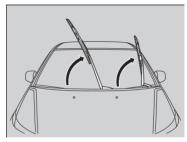
**1.** Lift the driver side wiper arm first, then the passenger side.
