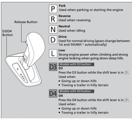
You cannot turn the ignition switch to LOCK  $\boxed{0}$  and remove the key unless the shift lever is in  $\boxed{P}$ .
