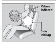
When the sensors detect a moderate-tosevere side impact, the control unit signals the side airbag on the impact side to immediately inflate.
