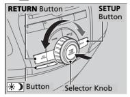
Use the selector knob or **SETUP** button to access some audio functions.
