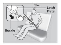
**3.** Insert the latch plate into the buckle.
