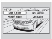
Press the **SETUP** button while the DVD is playing to see the available options. Use the  $\triangle$ ,  $\nabla$ ,  $\triangleright$ , and  $\triangleleft$  buttons to highlight the option and then press the **ENTER** button.
