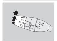
Automatic lighting control can be used when the ignition switch is in ON  $\boxed{II}$ .
