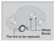
**6.** Place a wheel block or rock in front and rear of the wheel diagonal to the flat tire.
