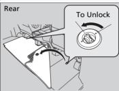
The front and second row passenger's floor mats hook over the floor anchors, which keep the mats from sliding forward. To remove a mat for cleaning, turn the anchor knobs to the unlock position. When reinstalling the mat after cleaning, turn the knobs to the lock position.
