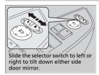
If activated, either side door mirror automatically tilts downward when you put the shift lever in  $\boxed{R}$ ; this improves close-in visibility on the selected side of the vehicle when backing up. The mirror automatically returns to its original position when you shift out of  $\boxed{R}$ .
