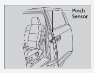
Do not touch the pinch sensor located at the front edge of the power sliding door. Do not damage the sensor. The power sliding door may not operate properly.
