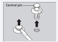
Insert the clip with the central pin raised, and push until it is flat.
