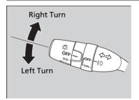
The turn signals can be used when the ignition switch is in ON  $\boxed{II}$ .
