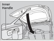
To manually close the tailgate, grab the inner handle, pull the tailgate down, and push it closed from outside.
