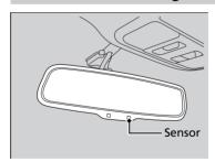
When driving after dark, the automatic dimming rearview mirror always reduces the glare from headlights behind you, based in inputs from the mirror sensor. This feature is always active.
