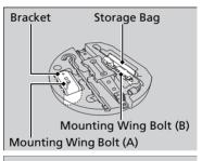
The storage bag, bracket, mounting wing bolt (A) and mounting wing bolt (B) are in the tool case.
