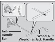
**3.** Raise the vehicle, using the jack handle bar and the jack handle, until the tire is off the ground.
