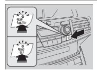
Press the rear defogger and heated door mirror button to defog the rear window and mirrors when the ignition switch is in ON  $\boxed{II}$ .
