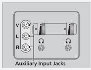
The system also allows for auxiliary inputs from standard video games. The jacks are above the third row seat armrest on the driver's side.
