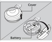
**2.** Make sure to replace the battery with the correct polarity.
