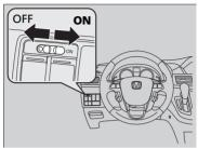
**Automatic operation:** Select the **ON** position of the sliding door main switch. **Manual operation:** Select the OFF position of the sliding door main switch.
