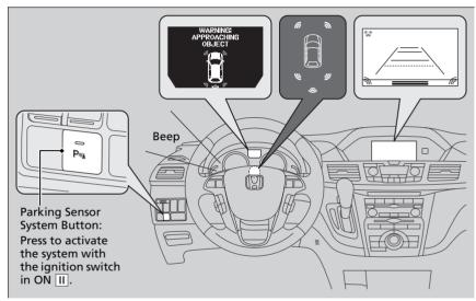
The indicator in the button comes on and the beeper sounds when the system is on.
