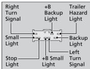
Your trailer lighting connector is located behind the left side panel in the cargo area. Each pin's purpose and wiring color code are shown in the image.
