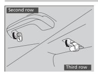
There are coat hooks on the both side of the grab handle and the window frame. Pull it down to use it.
