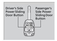
Press the power sliding door button for more than one second to operate.
