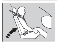
Adjust the driver's seat-back to a comfortable. upright position, leaving ample space between your chest and the airbag cover in the center of the steering wheel.
