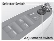
Place the selector switch in the L or R position to use the reverse tilt door mirror feature.
