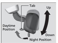
Flip the tab to switch the position.
