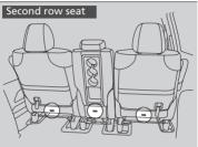
A tether anchorage point is provided behind each second and third row seating position. A child seat that is installed with a seat belt and comes with a tether can use the tether for additional security.
