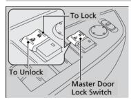
Press the master door lock switch in as shown to lock or unlock all doors and the tailgate.
