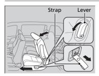
Pull up on the seat-back angle adjustment lever, or pulling the release strap tilts the second row outer seat's seat-back forward.
