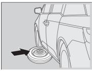
**7.** Place the compact spare tire (wheel side up) under the vehicle body, near the tire that needs to be replaced.
