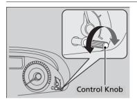
When the ignition switch is in ON III, you can use the brightness control knob to adjust instrument panel brightness.
