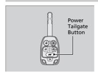
Press the power tailgate button for more than one second to operate.
