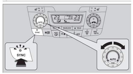
You can set the temperature synchronously for the driver side, the passenger side and the rear passenger compartment in synchronized mode.
