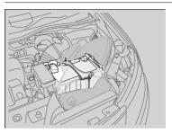
The battery condition is being monitored by the sensor on the negative terminal. If there is a problem with the sensor, the warning message on information display\*/multi-information display\* will let you know. Have your vehicle checked by a dealer.
