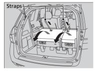
**2.** The front leg automatically latches. Pull the strap to put the seat-back(s) upright.
