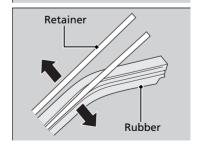
**4.** Remove the retainers from wiper blade and mount it to a new rubber blade.
