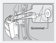
To reinstall, insert the fasteners into the grommets and push the assembly back into place.
