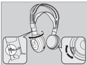
**To turn on the switch:** Pivot the left earpiece outward.
