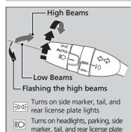
Rotating the light switch turns the lights on and off, regardless of the position of the ignition switch.
