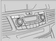
The appropriate indicator will be on while the seat heater is on. Each time you press the switch, the mode changes to HI, LOW and OFF.
