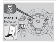
This button is on the driver side control panel. To turn the VSA® system on and off, press and hold it until you hear a beep.
