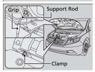
**4.** Remove the support rod from the clamp using the grip. Mount the support rod in the hood.
