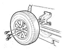
When replacing the spare tire, make sure you put it on the carrier with the outside of the wheel facing out. Tighten the bolts securely.
