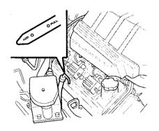
If you check the oil level when the oil is cold, do not run the engine first. The cold oil will not drain into the pan fast enough to give a true reading.
