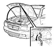
Place the support rod in its retaining clip and lower the hood.
