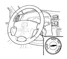
**LOCK** — The normal parking position. This locks the steering and prevents normal use of the steering wheel.
