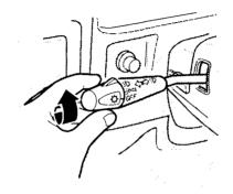
The rotating switch on the left lever controls the lights. Rotating this switch to the DOF position turns on the instrument panel lights and all exterior lights except the headlights. Rotating the switch to the Dosition turns on the headlights.
