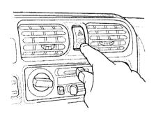
Use the hazard warning lights to warn other drivers that your vehicle is a potential road hazard. Avoid stopping on the roadway if possible.
