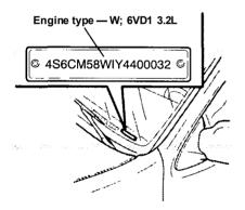
The VIN also appears on the vehicle's Certification Label on the driver's door lock pillar.
