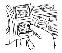
The indicator light in the switch lights to show the defogger is on. The defogger will shut itself off after 10 minutes. If the rear window or mirrors are not completely clear, press the switch
