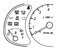
The indicator light should turn on when the ignition switch is turned to the "ON" position, but should go out after a few seconds.
