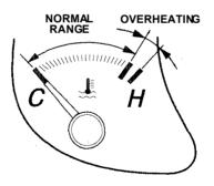
The gray area indicates the normal engine coolant temperature.
