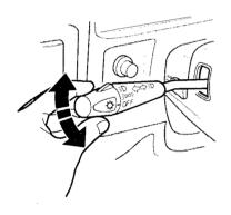
The turn signal will cancel itself as the turn is completed. In some driving maneuvers, such as changing lanes on an expressway, the steering wheel is not turned back sufficiently after completing the turn to automatically cancel the turn signal. In such maneuvers the driver should manually return the lever to the neutral or canceled position when the turn is completed.
