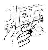
To flash the high beams, pull the lever back about half way and then let it go. The high beams will stay on for as long as you hold the lever back, no matter what position the headlight switch is in.
