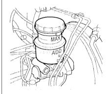
If the diaphragm inside the reservoir cap is deformed, return it to the original (collapsed) condition, then tighten the cap.
