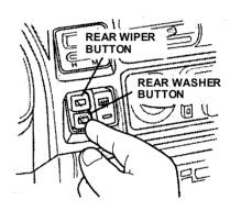
The rear window wiper cannot be operated when the rear window is unlocked.
