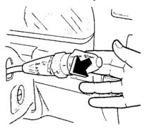
To operate the windshield washers, pull back on the windshield wiper control lever. The washers will spray, and the wipers will run at low speed, for as long as you hold the lever. The wipers will continue to run for a short time after you release the lever.
