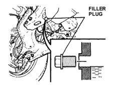
Remove the filler plug and make sure the fluid level is up to the edge of the hole. If it is not, add GL-5 gear oil to bring to that level. Use the same GL-5 gear oil specified for the front axle (see page 212).
