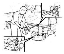
Reverse this procedure to store the spare tire. Connect the spare tire to the bracket with the outside of the wheel facing up. Make sure the tire does not catch on any part of the underbody of the vehicle as you are raising it, and that the spare tire is stored securely before driving.
