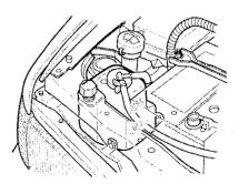
You usually do not need to remove the radiator cap to check the engine coolant level
