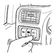
When fog or heavy mist reduces your forward vision, push this switch to turn the fog lights on. The indicator light in the switch turns on. Push the switch again to turn off the fog lights.
