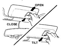
The moonroof has two positions: it can be tilted up in the back for ventilation, or it can be slid back into the roof. Use the switch above the rear view mirror to operate the moonroof. The ignition must be ON.
