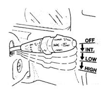
In INT, the wipers operate every few seconds. In LO and HIGH, the wipers run continuously.
