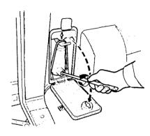
To remove the jack from its compartment, turn the handle counterclockwise. Disconnect the hold-down strap.
