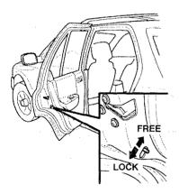
This is done by depressing the lever shown in the illustration. To disengage the lock, open the door from the outside and raise the lever.
