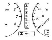
If anything goes wrong, the ABS indicator on the instrument panel comes on (see page 65). This means the anti-lock function of the braking system has shut down. The brakes still work like a conventional system without anti-lock, providing normal stopping ability. You should have the dealer inspect your vehicle as soon as possible if this light stays on after you start the engine, or comes on while driving.
