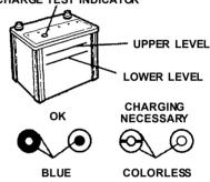
You will never have to add water. The hydrometer (test indicator) in the top of the battery provides information for testing purposes only.
