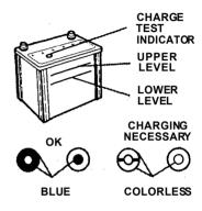
If the battery is a sealed type and if the fluid level is below the lower level line on the side of the battery, do not try to jump start the vehicle or charge or test the battery. Do not add fluid. Instead, install a new battery.
