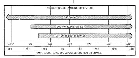
viscosity grade. If cold-weather starting problems are encountered at temperatures below 0°F (—18°C), SAE 5W—30 viscosity oils may be required.
