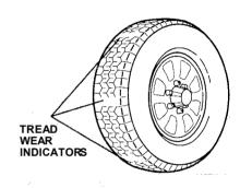
When the tread wears down to that point, you will see a 1/2 inch (12.7 mm) wide band running across the tread. This shows that there is less than 1/16 inch (1.6 mm) of tread left on the tire. A tire that is this worn gives very little traction on wet roads. You should replace the tire if you can see the tread wear
