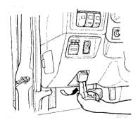
2. Lift the under-hood lever while lifting the hood slightly.
