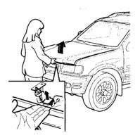
Raise the hood, and hold it open with the hood support rod in the hole on the right side of the hood.
