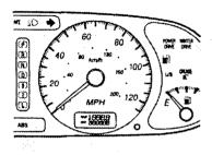
When more powerful acceleration is needed, select the "POWER" driving program. The "POWER DRIVE" indicator light comes on when the driving pattern selector is set in the "POWER" position. Push the button again to turn it off.
