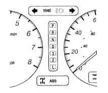
The shift lever position indicator is in the instrument panel. The appropriate letter or number illuminates to show what position the shift lever is in.
