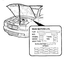
It is located on the center dash wall inside the engine compartment. The plate lists the VIN (Vehicle Identification Number), paint information and all production options and special
