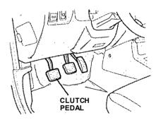
When the pedal is fully released, the clutch is engaged, driving the transmission and the drive wheels.
