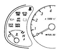
If the light flashes, it means the computer controlling the transmission has found a problem. Have the automatic transmission
