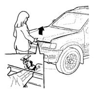
Lift the under-hood lever while lifting the hood slightly. Raise the hood, and hold it open with the hood support rod in the hole on the right side of the hood.
