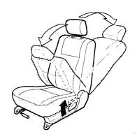
Raise the lever and use body pressure to move the seat-back to the desired position. Let go of the lever and the seat-back will lock into the desired position.
