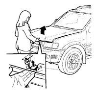
2. Lift the under-hood lever while lifting the hood slightly.
