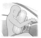
Airbagsare designed to give added protection for the head and chest in a severe frontal collision.
