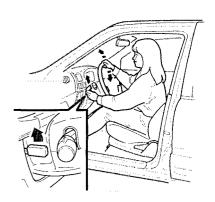
To adjust the height of the steering wheel, push up on the lever. The steering wheel has six
