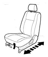
Let go of the lever and the seat will lock into the desired position.
