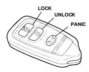
You can lock and unlock your vehicle with the remote transmitter. When you push the LOCK button, all the doors and the tailgate lock. The parking lights, taillights, and license plate light will flash once. If you press the LOCK button a second time, the horn will honk to confirm that everything locked.
