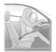
When sensors detect a severe front al collision, the airbags instantly inflate to provide extra protection for an occupant's head and chest.
