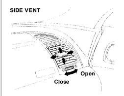
The vents in the corners of the dashboard can be opened and closed with the dials underneath them.
