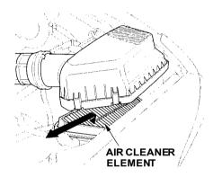
Carefully clean the inside of the air cleaner housing with a damp rag.
