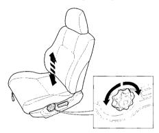
See pages 13 — 14 for important safety information and warnings about how to properly position seats and seat-backs. To adjust the height of the driver's seat, turn the dial on the outside of the seat bottom.
