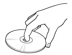
Handle a CD by its edges; never touch either surface. Contamination from fingerprints, liquids, felt-tip pens, and labels can cause the CD to not play properly, or possibly jam in the drive.
