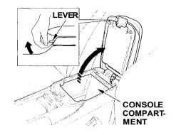
To open the console compartment, pull up on the lower lever and lift the lid.
