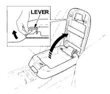
You can put small items in the tray located in the console compartment lid. To use the tray, pull up on the upper lever and lift up the armrest pad.
