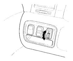
The dial on the dashboard to the left of the instrument panel controls the brightness of the instrument panel lights. Turn the dial to adjust the brightness.
