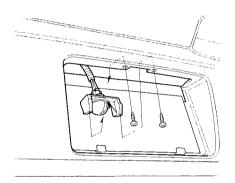
1. Use a Phillips-head screwdriver to remove the two screws holding the license plate light assembly to the bracket. Pull the assembly away from the bracket.
