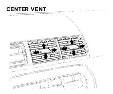
You can adjust the direction of the air coming from the dashboard vents by moving the tab in the center of each vent up-and-down and side-to-side.
