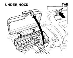
The under-hood fuse box is located in the back of the engine compartment on the passenger's side. To open it, push the tab as shown.
