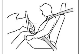
After inflating, the airbags immediately deflate, so they won't interfere with the driver's visibility, or the ability to steer or operate other controls.
