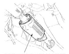
THREE WAY CATALYTIC CONVERTER
