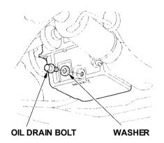
Open the hood and remove the engine oil fill cap. Remove the oil drain bolt and washer from the bottom of the engine. Drain the oil into an appropriate container.
