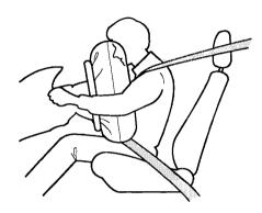
If you ever have a moderate to severe frontal collision, the sensors will detect rapid deceleration and signal the control unit to instantly inflate the airbags.
