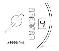
This indicator in the tachometer shows which position the shift lever is in. The illuminated number next to the "D4" indicator shows you the gear you have selected in the Sequential SportShift mode.
