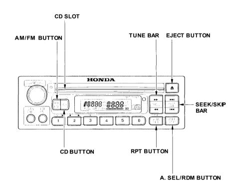
If you turn the system off while a CD is playing, either with the PWR/VOL knob or by turning off the ignition, the disc will stay in the drive. When you turn the system back on, the CD will begin playing where it left off.
