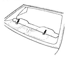
You car has two places on the rear shelf where a tether anchor can be installed. A tether anchor is used to secure a tether-style child seat to the car.
