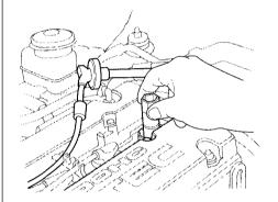
5. Put the new spark plug into the socket; then screw it into the hole. Screw it in by hand so you do not crossthread it.
