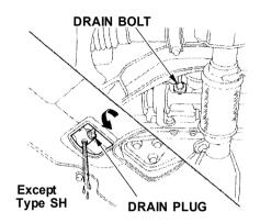
Except Type SH only Remove the drain bolt and washer from the engine block.
