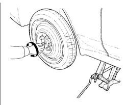
13. Put on the spare tire. Put the wheel nuts back on finger-tight, then tighten them in a crisscross pattern with the wheel wrench until the wheel is firmly against the hub. Do not try to tighten them fully.
