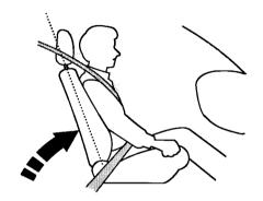
Adjust the driver's seat-back to a comfortable, upright position, leaving ample space between your chest and the airbag cover in the center of the steering wheel. If you sit too close to the steering wheel, you could be injured if the airbag inflates.
