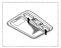
Turn on the spotlight by pushing the button next to each light. Push the button again to turn it off. You can use the spotlights at all times.
