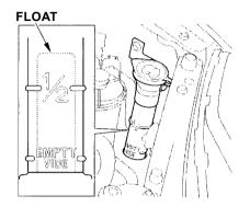
Check the level in the windshield washer reservoir at least monthly during normal usage. In bad weather, when you use the washers often, check the level every time you stop for fuel.
