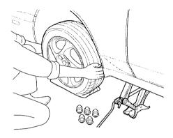
11 Remove the wheel nuts and flat tire. Temporarily place the flat tire on the ground with the outside surface of the wheel facing up. You could scratch the wheel if you put it face down.
