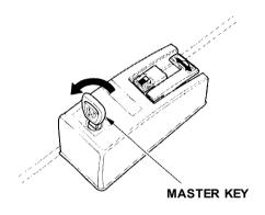
To protect items in the trunk when you need to give the key to someone else, lock the trunk release handle with the master key and give the other person the valet key.
