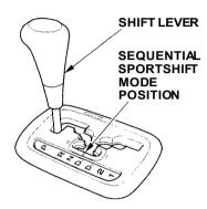
The shift lever has eight positions. It must be in Park or Neutral to start the engine. When you are stopped in D4, D3, 2, 1, N, R, or the Sequential SportShift mode, press firmly on the brake pedal and keep your toot off the accelerator pedal.
