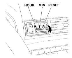
The digital clock displays the time with the ignition switch ON (II).
