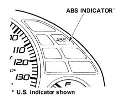
The ABS is self-checking. If anything goes wrong, the ABS indicator on the instrument panel comes on (see page 56). This means the anti-lock function of the braking system has shut down. The brakes still work like a conventional system without anti-lock, providing normal stopping ability. You should have the dealer inspect your car as soon as possible.
