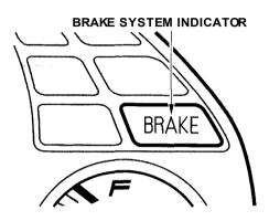
The Brake System indicator light comes on when you turn the ignition ON (II). If the parking brake is not set, it goes off after you start the engine. If the parking brake is set, it goes off when you fully release the parking brake with the engine runnina.
