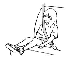
If the shoulder part of the belt rests over the child's collarbone and against the center of the chest, as shown, the child is large enough to wear the seat belt. However, if the belt touches or crosses the child's neck, the child needs to use a booster seat.
