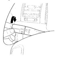
The rotating switch on the left lever controls the lights. Turning this switch to the " FOGE " position turns on the parking lights, taillights, instrument panel lights, side-marker lights, and rear license plate lights. Turning the switch to the " ED " position turns on the headlights.
