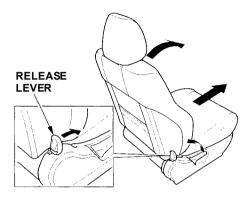
To get into the back seat on the passenger's side, push forward on the release lever at the base of the seat-back. The seat-back will tilt forward and the entire seat will move forward to allow easier entry to the back seat. After you return the seat-back to the upright position, push the whole seat backwards until it latches. Make sure the seat is fully latched before sitting in it.
