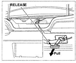
To release the seat-back from inside the trunk, pull the release under the rear shelf.
