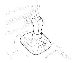
The manual transmission is synchronized in all forward gears for smooth operation. It has a lockout so you cannot shift directly from Fifth to Reverse. When shifting up or down, make sure you push the clutch pedal down all the way, shift to the next gear, and let the pedal up gradually. When you are not shifting, do not rest your foot on the clutch pedal. This can cause your clutch to wear out faster.
