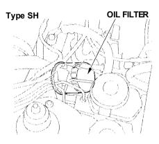
3. Remove the oil filter and let the remaining oil drain. A special wrench (available from your Honda dealer) is required to remove the filter
