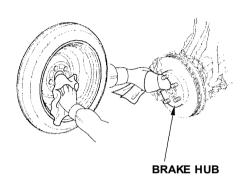
12. Before mounting the spare tire, wipe any dirt off the mounting surface of the wheel and hub with a clean cloth. Wipe the hub carefully, it may be hot from driving.
