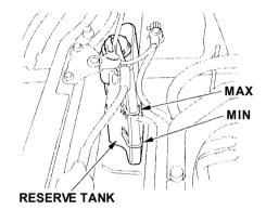
Look at the coolant level in the radiator reserve tank. Make sure it is between the MAX and MIN lines. If it is below the MIN line, see Adding Engine Coolant on page 185 for information on adding the proper coolant.
