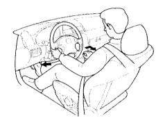
To avoid transmission damage, come to a complete stop before shifting into Park. The shift lever must be in Park before you can remove the key from the ignition switch.
