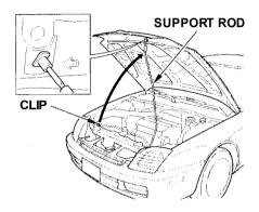
3. Pull the support rod out of its clip and insert the end into the hole on the left side of the hood.
