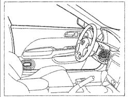
Your car has a courtesy light in the ignition switch. The ignition switch light comes on whenever you open either door. It remains on, then fades out in about 10 seconds after both doors are closed tightly.
