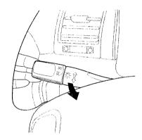
To change between low beams and high beams, pull the turn signal lever until you hear a click, then let go. The blue high beam indicator will light (see page 57).
