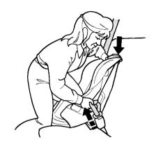
4. After confirming that the belt is locked, grab the shoulder part of the belt near the buckle and pull up to remove any slack from the lap part of the belt. Remember, if the lap part of the belt is not tight, the child seat will not be secure. It may help to put weight on the child seat, or push on the back of the seat, while pulling up on the belt.
