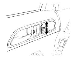
Each door has a master door lock switch. This switch locks and unlocks both doors. Push the switch down to lock both doors and up to unlock them.
