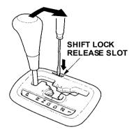
6. Remove the screwdriver from the shift lock release slot, then install a new cover.
