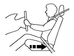
Any driver who sits too close to the steering wheel is at risk of being seriously injured or killed by striking the steering wheel, or from being struck by an inflating airbag during a crash.
