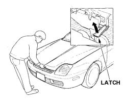
2. Standing in front of the car, put your fingers under the front edge of the hood to the right of center. Slide your hand to the left until you feel the hood latch handle. Push this handle up until it releases the hood. Lift the hood
