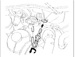
2. Remove the socket from the headlight assembly by turning it one-quarter turn counterclockwise.
