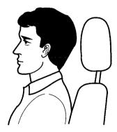
Before driving, make sure everyone with an adjustable head restraint has properly positioned the head restraint. The restraint should be positioned so the back of the occupant's head rests against the center of the restraint. A taller person should adjust the restraint as high as possible.
