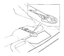
Attach the tether strap hook to the tether anchorage point and tighten the strap according to the child seat maker's instructions.
