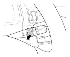
To clean the windshield, pull back on the wiper control lever. The washers spray until you release the lever.
