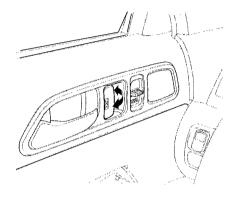
Each door has a lock tab next to the inside door handle. When you push in the lock tab on the driver's door, both doors lock. Pulling out the lock tab on the driver's door only unlocks that door. The lock tab on the passenger's door only locks and unlocks that door.
