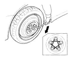
15. Tighten the wheel nuts securely in the same crisscross pattern. Have the wheel nut torque checked at the nearest automotive service facility.
