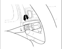
In intermittent, the wipers operate every few seconds. You can vary how often the wipers sweep the windshield by turning the INT TIME ring next to the rotary switch. In low speed and high speed, the wipers run continuously.
