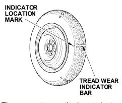
The compact spare tire has a shorter tread life than a regular tire. Replace it when you can see the tread wear indicator bars. The replacement should be the same size and design tire, mounted on the same wheel. The compact spare tire is not designed to be mounted on a regular wheel, and the compact wheel is not designed for mounting a regular tire.
