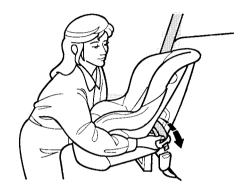
With the child seat in the desired back seating position, route the belt through the child seat according to the seat maker's instructions, then insert the latch plate into the buckle.
