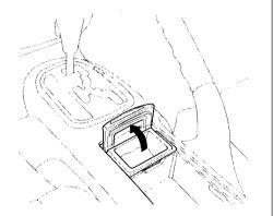
The coin box is located next to the beverage holder. Open the lid by lifting it up.
