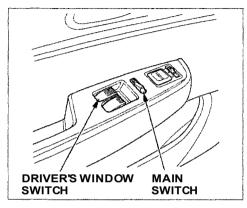
The driver's armrest has a master power window control panel. To open the passenger's window, push down on the switch and hold it down until the window reaches the desired position. To close the window, pull back on the window switch. Release the switch when the window gets to the position you want.
