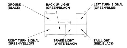
Your vehicle has a trailer lighting connector located behind the left side panel in the cargo area. Refer to the drawing above for the wiring color code and purpose of each pin.
