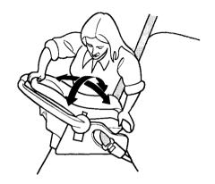
5. Push and pull the child seat forward and from side to side to verify that it is secure enough to stay upright during normal driving maneuvers. If the child seat is not secure, unlatch the belt, allow it to retract fully, then repeat these steps.
