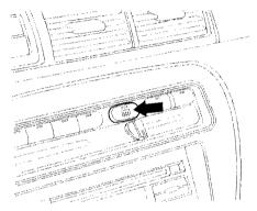
The rear window defogger will clear fog, frost, and thin ice from the window. Push the defogger button to turn it on and off. The light in the button lights to show the defogger is on. If you do not turn it off, the defogger will shut itself off after about 25 minutes. It also shuts off when you turn off the ignition. You have to turn it on again when you restart the car.
