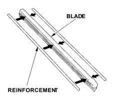
4. Examine the new wiper blades. If they have no plastic or metal reinforcement along the back edge, remove the metal reinforcement strips from the old wiper blade and install them in the slots along the edge of the new blade.
