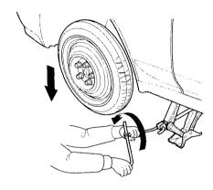
14. Lower the car to the ground and remove the jack.
