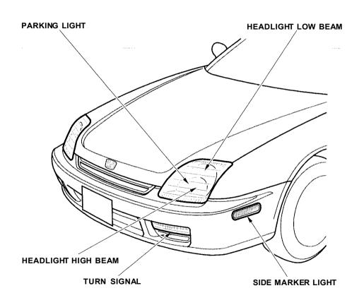
Check the operation of your car's exterior lights at least once a month. A burned out bulb can create an unsafe condition by reducing your car's visibility and the ability to signal your intentions to other drivers.
