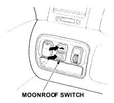
Use the switch on the dashboard to open and close the moonroof. The ignition switch must be ON (II). Push and hold the switch to open the moonroof. Release the switch when the moonroof reaches the desired position. To close the moonroof, press and hold the switch.
