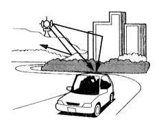
Radio signals, especially on the FM band, are deflected by large objects such as buildings and hills. Your radio then receives both the direct signal from the station's transmitter, and the deflected signal. This causes the sound to distort or flutter. This is a main cause of poor radio reception in city driving.
