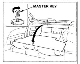
To fold down the seat-back from inside the car. insert the master key in the lock on the rear shelf. Turn the key clockwise, pull down the top of the seat-back, then release the key.
