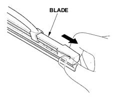
3 Remove the blade from its holder. by grasping the tabbed end of the blade. Pull firmly until the tabs come out of the holder.
