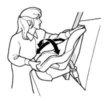
Push and pull the child seat forward and from side to side to verify that it is secure enough to stay upright during normal driving maneuvers. If the child seat is not secure, unlatch the belt, allow it to retract fully, then repeat these steps.
