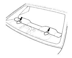
Your car has two tether anchorage points on the rear shelf for securing a tether-style child seat to the car.
