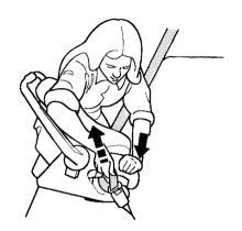
4. After confirming that the belt is locked, grab the shoulder part of the belt near the buckle and pull up to remove any slack from the lap part of the belt. Remember, if the lap part of the belt is not tight, the child seat will not be secure. To remove slack, it may help to put weight on the child seat, or push on the back of the seat, while pulling up on the belt.
