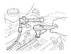
Torque the spark plug. (If you do not have a torque wrench, tighten the spark plug two-thirds of a turn after it contacts the cylinder head.) Tightening torque:
