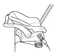
For proper protection, an infant must ride in a reclined, or semi-reclined position. To determine the proper reclining angle, check with the baby's doctor or follow the seat maker's recommendations.
