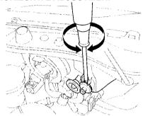
6. If either indicator is not aligned with its "0" mark as described, an adjustment can be made using a Phillips-head screwdriver to realign it with the "0" mark. Please refer to the illustrations.
