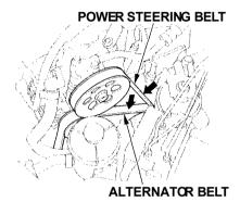
Check the condition of the two drive belts. Examine the edges of each belt for cracks or fraying. Check the tension of each belt by pushing on it with your thumb midway between the pulleys.
