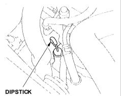
Check the fluid level with the engine at normal operating temperature.
