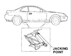
9. Locate the jacking point nearest the tire you need to change. It is pointed to by a  $\triangle$  mark molded into the underside of the body. Place the jack under the jacking point. Turn the end bracket clockwise until the top of the jack contacts the jacking point. Make sure the jacking point tab is resting in the jack notch.
