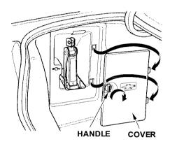
6. The jack is behind a cover in the left fender. Remove the cover by turning the handle clockwise, then pulling on the cover.
