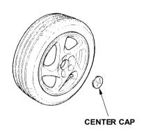
16. Remove the center cap before storing the flat tire in the trunk well.
