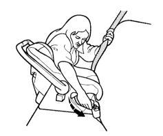
With the child seat in the desired back seating position, route the belt through the child seat according to the seat maker's instructions, then insert the latch plate into the buckle.
