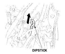
Check the engine oil level every time you fill the car with fuel. Wait a few minutes after turning the engine off before you check the oil.
