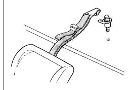
Install the anchor plate and mounting hardware. The hardware is available from your Honda dealer (part number 82410-SE3-C01).
