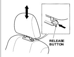
The front head restraints help protect you and your passenger from whiplash and other injuries. They are most effective when you adjust them so the back of the occupant's head rests against the center of the restraint. A taller person should adjust the restraint as high as possible.
