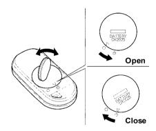
When the remote transmitter's battery begins to get weak, it may take several pushes on the button to lock or unlock the doors, and the LED will get dim. Replace the battery as soon as possible.
