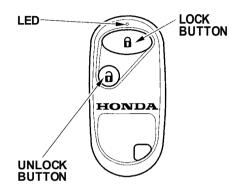
You can lock and unlock your car with the remote transmitter. When you push the LOCK button, both doors lock.
