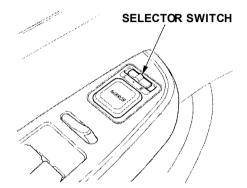
Adjust the outside mirrors with the adjustment switch on the driver's door armrest:
