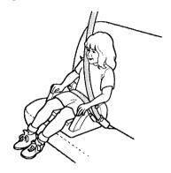
If a child needs a booster seat, we recommend choosing a style that allows the child to use the lap/ shoulder belt directly, without a shield, as shown.
