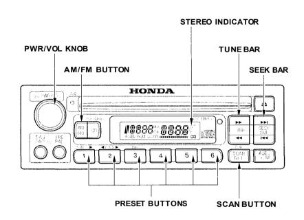
You can use any of four methods to find radio stations on the selected band: TUNE. SEEK. SCAN or the Preset buttons
