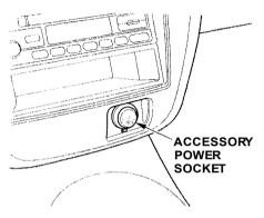
To use the accessory power socket, pull down the cover. The ignition switch must be in ACCESSORY (I) or ON (II).
