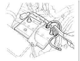
Check the battery terminals for corrosion (a white or yellowish powder). To remove it, cover the terminals with a solution of baking soda and water. It will bubble up and turn brown. When this stops, wash it off with plain water. Dry off the battery with a cloth or paper towel. Coat the terminals with grease to help prevent future corrosion.
