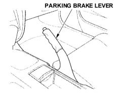
To apply the parking brake, pull the lever up fully. To release it, pull up slightly, push the button, and lower the lever. The parking brake light on the instrument panel should go out when the parking brake is fully released (see page 55).
