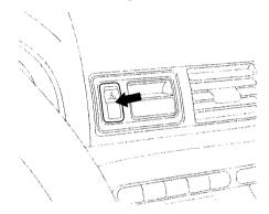
Push the red button to the left of the clock to turn on the hazard warning lights (four-way flashers). This causes all four outside turn signals and both indicators in the instrument panel to flash. Use the hazard warning lights if you need to park in a dangerous area near heavy traffic, or if your car is disabled.
