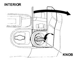
The interior fuse box is underneath the dashboard on the driver's side. To open it, turn the knob as shown.
