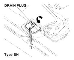
Loosen the drain plug on the bottom of the radiator. The coolant will come out through the hole in the splash cover.
