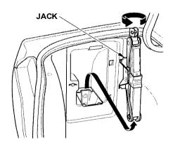
7. Turn the jack's end bracket counterclockwise to loosen it, then remove the jack.
