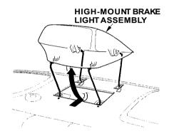
1. Remove the high-mount brake light assembly by pushing it slightly toward the rear windshield and sliding it out of the rear shelf.
