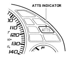
The Active Torque Transfer System (ATTS) is self-checking. If a problem is detected in the system, the ATTS indicator on the instrument panel comes on.
