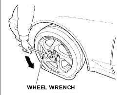
8. Loosen the five wheel nuts 1/2 turn with the wheel wrench.
