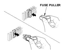
4. Check the smaller fuses in the under-hood fuse box and all the fuses in the interior fuse box by pulling out each fuse with the fuse puller provided in the interior fuse box.
