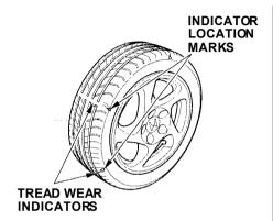
Your car's tires have wear indicators molded into the tread. When the tread wears down to that point, you will see a 1/2 inch (12.7 mm) wide band running across the tread. This shows there is less than 1/16 inch (1.6 mm) of tread left on the tire. A tire that is this worn gives very little traction on wet roads. You should replace the tire if you can see the tread wear indicator in three or more places around the tire.
