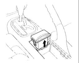
To remove the coin box for emptying, lift the coin box up by pushing up on the middle edge of the coin box on the console guide. Never use the coin box for smoking materials.
