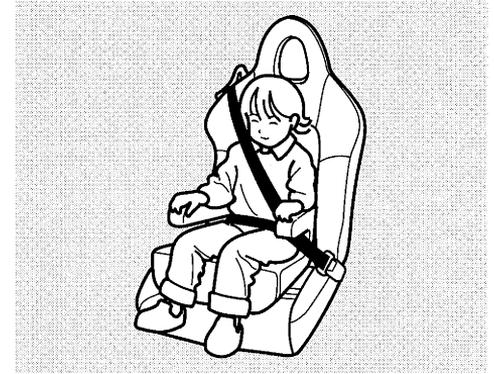
If a child needs a booster seat, we recommend choosing a style that allows the child to use the lap/shoulder belt directly, without a shield, as shown.
