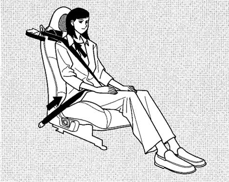
Your Honda has automatic seat belt tensioners for added protection during a moderate to severe frontal collision.
