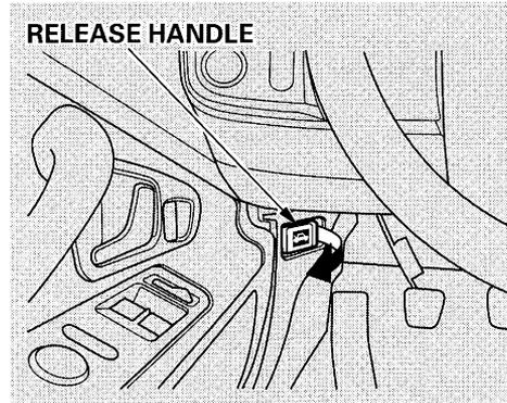
1. Shift to Neutral and set the parking brake. Pull the hood release handle located under the lower left corner of the dashboard. The hood will pop up slightly.
