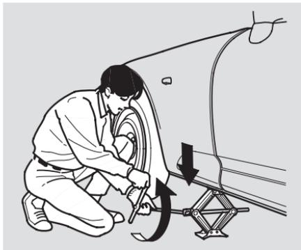
12. Lower the vehicle to the ground, and remove the jack.
