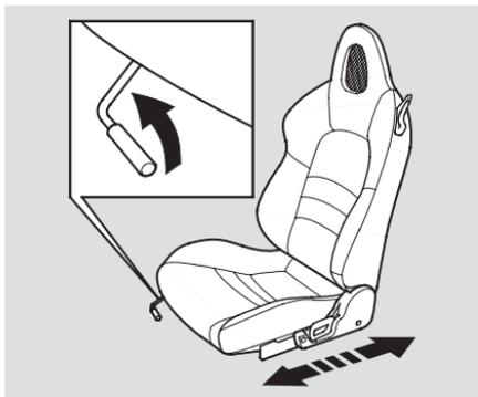
To adjust the seat forward and backward, pull up on the lever under the seat cushion's front edge. Then try to move the seat to make sure it is locked in position.
