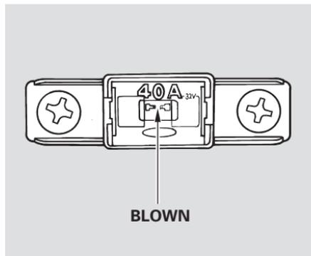
1. Turn the ignition switch to LOCK (0). Make sure the headlights and all other accessories are off.
