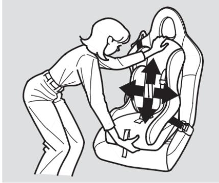
6. Push and pull the child seat forward and from side to side to verify that it is firmly secured. If the child seat is not secure, unlatch the belt, allow it to retract fully, then repeat these steps.
