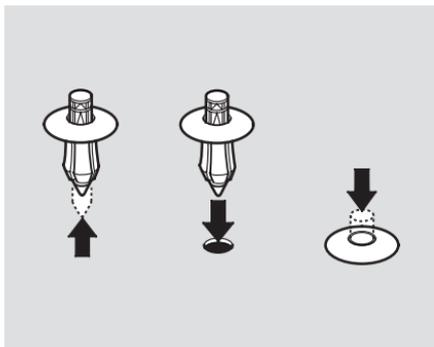
10. Install the trunk lining, and secure it with the fasteners. To reinstall a fastener, reset the fastener by pushing on the pointed end until it pops back almost flush with the fingers on the housing. Put the fastener in the hole of the trunk lining, and push on the center until it locks (the center is flush with the head).
