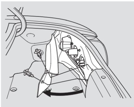
4. Determine which bulb is burned out: turn signal or back-up light.
