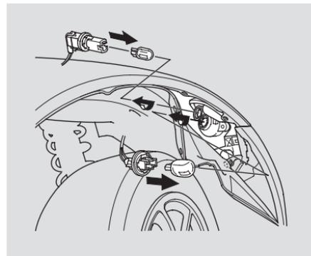
6. Install the new bulb in the socket.
