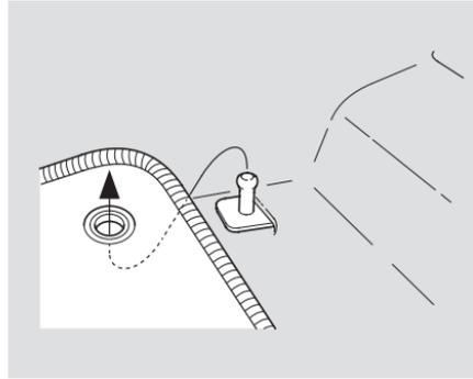
The driver's floor mat that came with your vehicle hooks over the floor mat anchor. This keeps the floor mat from sliding forward and possibly interfering with the pedals.
