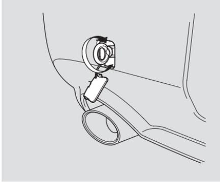
4. Screw the towing hook into the extension and tighten it securely by hand.
