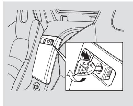
The area between the seat has two compartments. Open the lower compartment by squeezing the handle. Close it with a firm push. You can lock or unlock the lower compartment with the master key.
