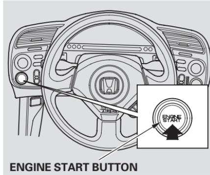
6. If the engine does not start within 15 seconds, or starts but stalls right away, repeat step 5 with the accelerator pedal pressed halfway down. If the engine starts, release pressure on the accelerator pedal so the engine does not race.
