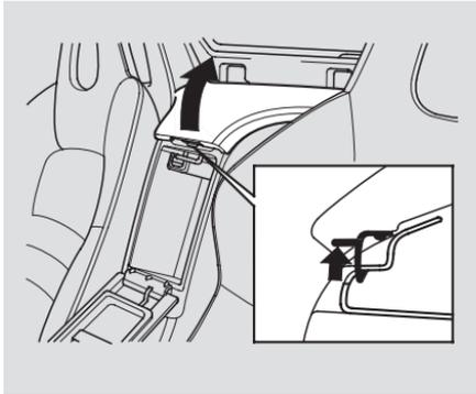
The lever to open the upper compartment is inside the lower compartment. Push up the lever, and lift the lid. To close, lower the lid, and push it down until it latches.
