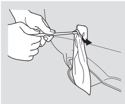
For very short distances, such as freeing the vehicle, you can use the detachable towing hook that mounts on the anchors in the front and rear bumpers.
