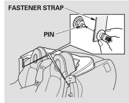
3. Pull the buttons, on the fastener straps, place them on the pin on the side panel just behind the doors, then release the buttons.
