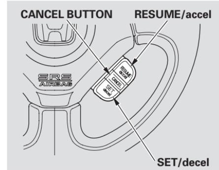
3. Press and release the SET/decel button on the steering wheel. The CRUISE CONTROL indicator on the instrument panel comes on to show the system is now activated.
