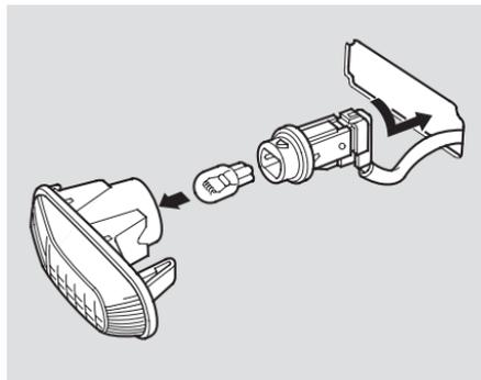
1. Use a small flat-tipped screwdriver to pry carefully on the back edge of the side turn signal assembly until it pops out of the body.
