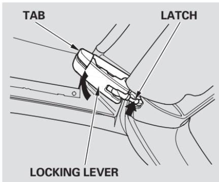
4. Push in the tab to release the locking levers, and pull them down. Note the movement of the latch when you push in the tab.
