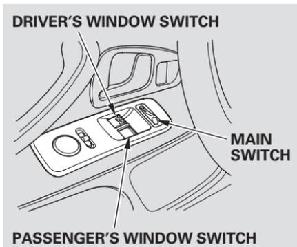
Each door has a switch that controls its window. To open the window, push the switch down and hold it. Release the switch when you want the window to stop. Close the window by pulling back on the switch and holding it.
