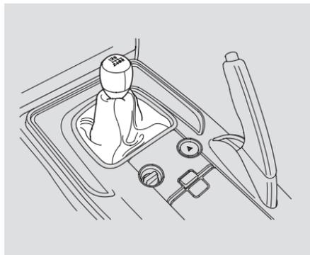
The manual transmission is synchronized in all forward gears for smooth operation. It has a lockout so you cannot shift directly from Fifth to Reverse instead of Sixth (see page 115). When shifting up or down, make sure you push the clutch pedal down all the way, shift to the next gear, and let the pedal up gradually. When you are not shifting, do not rest your foot on the clutch pedal. This can cause your clutch to wear out faster.
