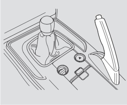
**NOTICE:** *Driving the vehicle with the parking brake applied can damage the rear brakes and axles.*
