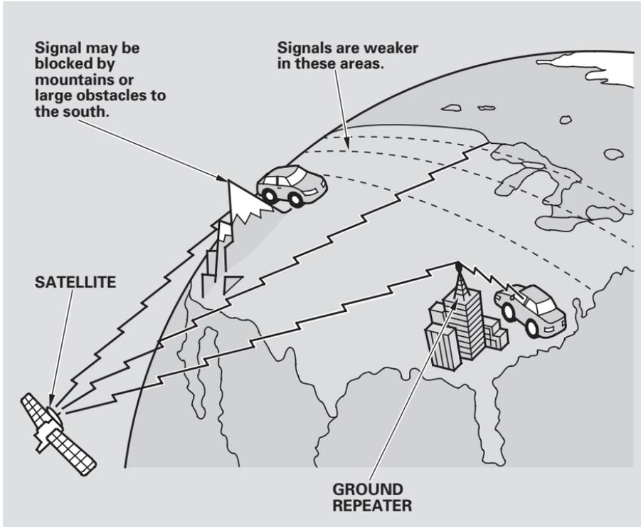
The XM satellites are in orbit near the equator; therefore, objects located south of the vehicle may cause satellite reception interruptions. Ground repeaters help strengthen the satellite signals, but there may be congested areas where these signals cannot be picked up. Signals become weaker the farther north you travel from the equator.
