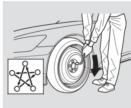
13. Tighten the wheel nuts securely in a crisscross pattern. Have the wheel nut torque checked at the nearest automotive service facility. Tighten the wheel nuts to:
