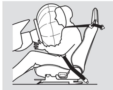
If you ever have a moderate to severe frontal collision, sensors will detect the vehicle's rapid deceleration. If the rate of deceleration is high enough, the control unit will instantly inflate the drivers and passenger's airbags.
