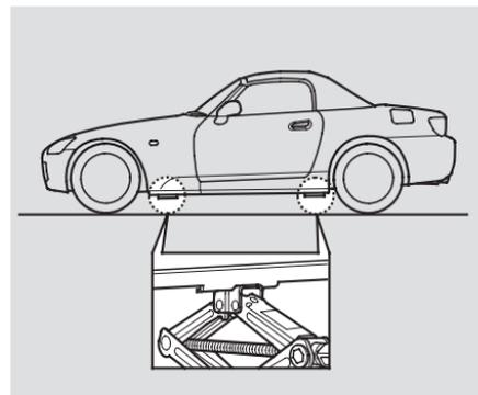
7. Locate the jacking point nearest the tire you need to change. It is pointed to by an arrow molded into the underside of the body. Place the jack under the jacking point. Turn the end bracket clockwise until the top of the jack contacts the jacking point. Make sure the center of the jacking point tab is resting in the jack notch.
