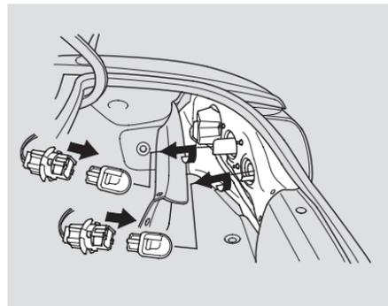
5. Remove the socket by turning it one-quarter turn counterclockwise.
