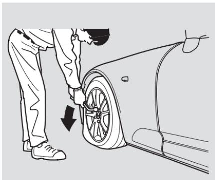
5. Unscrew the wing bolt, and take the spare tire out of the spare tire shelf.
