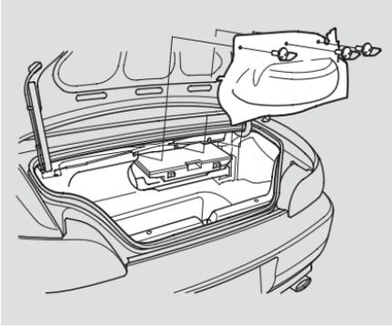
14. Remove the tool box from the trunk well, and replace the jack, wheel wrench, and extension in the tool box.
