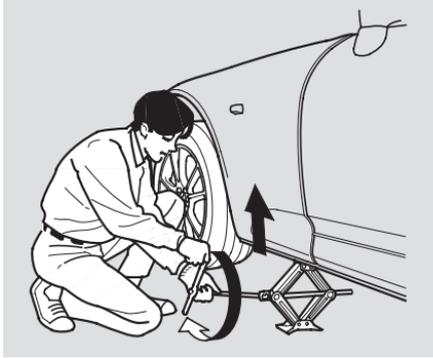
8. Use the extension and wheel wrench as shown to raise the vehicle until the flat tire is off the ground.
