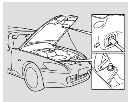
Lift it up slightly to remove the support rod from the hole. Put the support rod back into its holding clip. Lower the hood to about a foot (30 cm) above the fender, then let it drop. Make sure it is securely latched.
