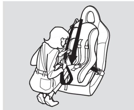
4. After the belt has retracted, tug on it. If the belt is locked, you will not be able to pull it out. If you can pull the belt out, it is not locked, and you will need to repeat these steps.
