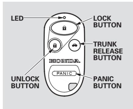
**LOCK** – Press this button to lock both doors. Some exterior lights will flash. When you push LOCK twice within 5 seconds, you will hear a beep to verify that the doors are locked.
