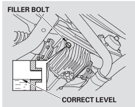
Check the fluid level with the differential at normal operating temperature and the vehicle sitting on level ground. Remove the differential fluid filler bolt and washer, and carefully feel inside the bolt hole with your finger. The fluid level should be up to the edge of the bolt hole. If it is not, slowly add fluid until it starts to run out of the hole.
