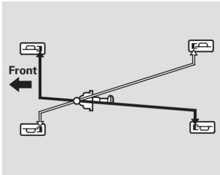
The hydraulic system that operates the brakes has two separate circuits. Each circuit works diagonally across the vehicle (the left-front brake is connected with the right-rear brake,
