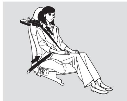
For added protection, the seat belts are equipped with automatic seat belt tensioners. When activated, the tensioners immediately tighten the belts to help hold the driver and the passenger in place.
