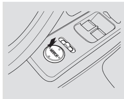
2. Push the appropriate edge of the adjustment switch to move the mirror right, left, up, or down.
