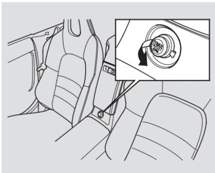
This socket is intended to supply power for 12 volt DC accessories that are rated 120 watts or less (10 amps).
