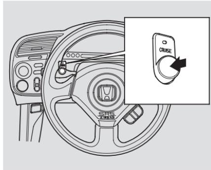
1. Push in the Cruise Control Master Switch. The indicator in the switch will come on.
