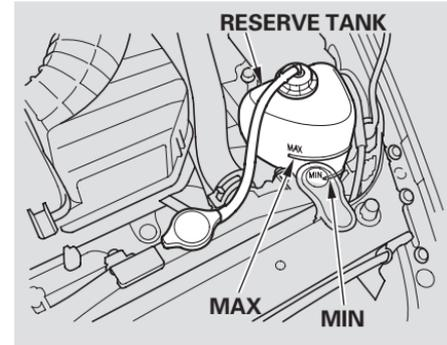
Look at the coolant level in the radiator reserve tank. Make sure it is between the MAX and MIN lines. If it is below the MIN line, see **Adding Engine Coolant** on page 132 for information on adding the proper coolant.
