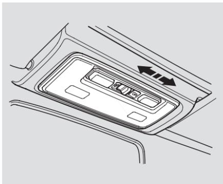
The interior light has a three-position switch. In the OFF position, the light does not come on. In the center position, the interior light comes on when you open either door. In the ON position, the interior light stays on continuously.
