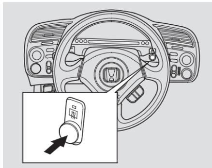
The rear window defogger will clear fog, frost, and thin ice from the window. Push the defogger button to turn it on and off. The indicator in the button comes on to show the defogger is on. If you do not turn it off, the defogger will shut itself off after about 15 minutes. It also shuts off when you turn off the ignition. You have to turn it on again when you restart the vehicle.
