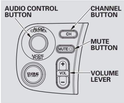
Four controls for the audio system are on the left side of the dashboard by the instrument panel. These let you control basic functions without distracting your attention from driving.
