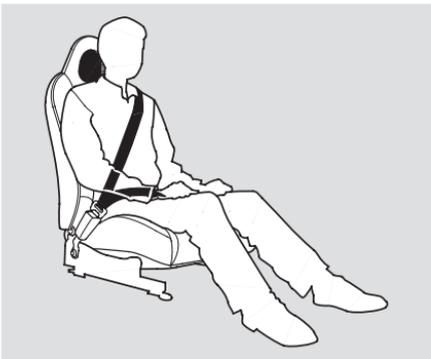
If necessary, pull up on the belt again to remove any slack, then check that the belt rests across the center of your chest and over your shoulder. This spreads the forces of a crash over the strongest bones in your upper body.
