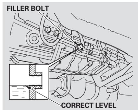
Check the fluid level with the transmission at normal operating temperature and the vehicle sitting on level ground. Remove the transmission filler bolt, and carefully feel inside the bolt hole with your finger. The fluid level should be up to the edge of the bolt hole. If it is not, add Honda Manual Transmission Fluid (MTF) until it starts to run out of the hole. Install the filler bolt, and tighten it securely.
