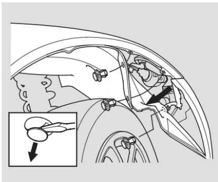
2. Use a flat-tipped screwdriver to remove the three holding clips from the inner fender.
