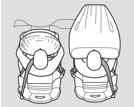
Your vehicle has a Supplemental Restraint System (SRS) with frontal airbags to help protect the heads and chests of the driver and a passenger during a moderate to severe frontal collision (see page 18 for more information on how your airbags work).
