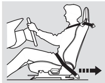
Adjust driver's seat as far to the rear as possible while allowing you to maintain control of the vehicle. Have a passenger adjust his or her seat as far to the rear as possible.
