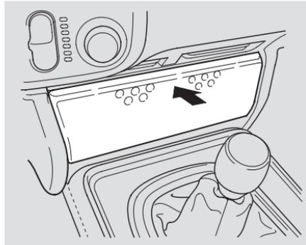
To open the audio panel, push on the top center, and let the panel swing down. To close, pivot the panel up, and push on it until it latches.
