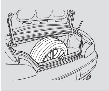
16. Replace the spare tire cover. Secure it with the three clips. Push each clip down securely, and pivot the ring down flat.
