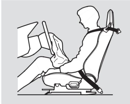
After inflating, the airbags will immediately deflate, so they won't interfere with the driver's visibility, or the ability to steer or operate other controls.
