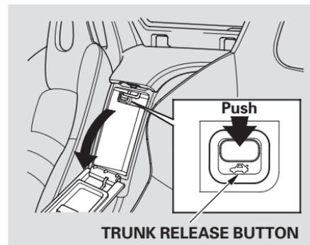
To open the trunk, press the trunk release button in the lower console compartment. To protect items in the trunk when you need to give the key to someone else, lock the lower console compartment with the master key, and give the other person the valet key.
