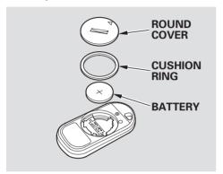
If it takes several pushes on the button to lock or unlock the doors and the hatch, replace the battery as soon as possible. Battery type: CR2025 To replace the battery, remove the round cover on the back of the transmitter by turning it counterclockwise with a coin. Insert a new battery with the + side facing up. Align the  $\bigtriangledown$  mark on the cover with the  $\bigcirc$  mark on the transmitter. Set the cover in place, and turn it clockwise.
