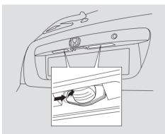
1. Slide the lens to the right until the left side of the lens pops out of the body. Pull out the light assembly.
