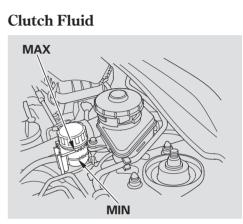
The fluid level should be between the MIN and MAX marks on the side of the reservoir. If it is not, add brake fluid to bring it up to that level. Use the same fluid specified for the brake system.
