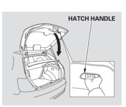
To close the hatch, use the hatch handle to lower the hatch, then press down on the back edge.
