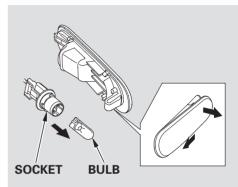
1. Front bumper: Push the front edge of the side marker lens toward the rear of the vehicle. The front edge will pop out of the bumper.
