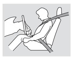
After inflating, the front airbags will immediately deflate, so they won't interfere with the driver's visibility, or the ability to steer or operate other controls. The total time for inflation and deflation is one-tenth of a second, so fast that most occupants are not aware that the airbags deployed until they see them lying in their laps.
