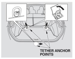
One tether anchor point for each of the outer rear seats is located under the cargo floor carpet and the tailgate sill. Pull up the carpet to access the anchor point (outboard anchor) when securing a tether-style child seat to the vehicle. Since a tether can provide additional security to the lap/shoulder belt installation, we recommend using a tether whenever one is required or available.
