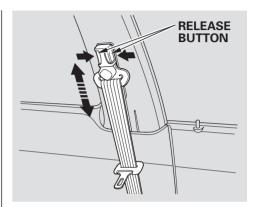
The front seats have adjustable seat belt anchors. To adjust the height of an anchor, press and hold the release buttons and slide the anchor up or down as needed (it has four positions). *Never place the shoulder portion of a lap/shoulder belt under your arm or behind your back.* This could cause very serious injuries in a crash.
