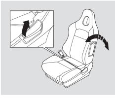
To change the seat-back angle of the front seat, pull up on the lever on the outside of the seat bottom.
