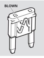
5. Look for a burned wire inside the fuse. If it is burned, replace it with one of the spare fuses of the same rating or lower.
