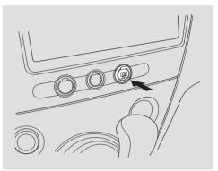
The rear window defogger will clear fog, frost, and thin ice from the window. Push the defogger button to turn it on and off. The indicator above the button comes on to show the defogger is on. If you do not turn it off, the defogger will shut itself off after about 15 minutes. It also shuts off when you turn off the ignition switch. You have to turn the defogger on again when you restart the vehicle.
