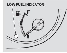
This indicator is located in the fuel gauge. If the indicator comes on, it means you should refuel soon.
