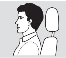
Have passengers with adjustable head restraints adjust their restraint so the back of their head rests against the center of the restraint. Taller persons should adjust their restraint as high as possible.
