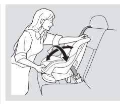
5. Push and pull the child seat forward and from side to side to verify that it is secure enough to stay upright during normal driving maneuvers. If the child seat is not secure, unlatch the belt, allow it to retract fully, then repeat these steps to deactivate the locking mechanism and remove a child seat, unlatch the buckle, unroute the seat belt, and let the belt fully retract.
