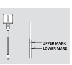
4. Remove the dipstick again and check the level. It should be between the upper and lower marks.
