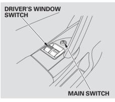
The driver's door armrest has a master power window control panel. To open the passenger's window, push down on the appropriate switch and hold it until the window reaches the desired position. To close the window, pull back on the window switch. Release the switch when the window gets to the position you want.
