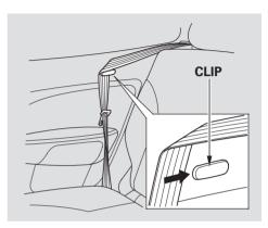
Before folding down the seat-back, move the seat belt out of the way and put the shoulder part of the outside seat belt in the clip on each side.
