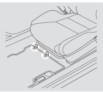
The driver's floor mat that came with your vehicle hooks over the floor mat anchor. This keeps the floor mat from sliding forward and possibly interfering with the pedals.
