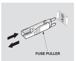
4. Check the smaller fuses in the under-hood fuse box and all the fuses in the interior fuse box by pulling out each one with the fuse puller provided in the under-hood fuse box.
