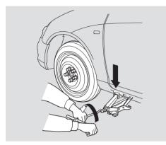
12.Lower the vehicle to the ground and remove the jack.
