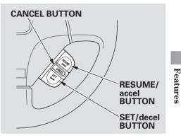
3. Press and release the SET/decel button on the steering wheel. The indicator on the instrument panel comes on to show the system is now activated.
