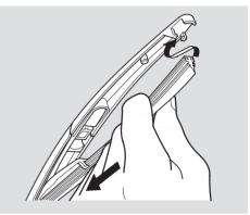
6. Insert both ends of the blade into the holder. Make sure they are secure.
