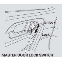
All doors lock when you push down the lock tab on the driver's door, or lock the driver's door from the outside with the key. Only the driver's door unlocks when you use the key or lock tab. To unlock the passengers' doors, use the master door lock switch or the lock tab on each door. Hatch
