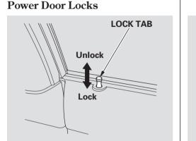
Each door has a lock tab on the top. When you push down the lock tab on the driver's door, both doors and the hatch lock. When you push down the lock tab on the passenger's door, only that door locks.
