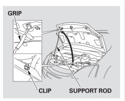
To close the hood, lift it up slightly to remove the support rod from the hole. Put the support rod back into its holding clip. Lower the hood to about a foot (30 cm) above the fender, then let it drop. Make sure it is securely latched.
