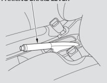
To apply the parking brake, pull the lever up fully. To release it, pull up slightly, push the button, and lower the lever. The parking brake indicator on the instrument panel should go out when the parking brake is fully released (see page 53).
