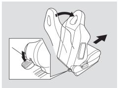
To get into the rear seat on the driver's side, pull up on the seat-back adjustment lever.
