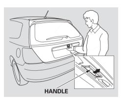
To open the hatch, pull the handle, then lift up.
