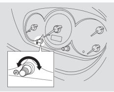
The knob on the instrument panel controls the brightness of the instrument panel lights. Turn the knob to adjust the brightness. Hazard Warning Button
