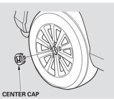
14. Remove the center cap before storing the flat tire in the spare tire well.
