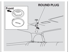
4. Use a screwdriver or coin to remove the round plug in the center of the headliner.
