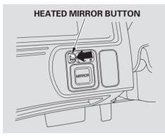
*Canadian model only* The outside mirrors are heated to remove fog and frost. With the ignition switch in the ON (II) position, turn on the heaters by pressing the button. The indicator in the button comes on as a reminder. Press the button again to turn the heaters off.
