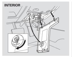
The vehicle's fuses are contained in two fuse boxes. The interior fuse box is located underneath the steering column. To open it, turn the knobs as shown.
