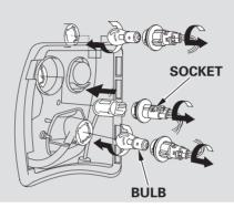
3. Determine which bulb, stop/ taillight, back-up light, or turn signal is burned out.
