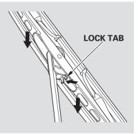
2. Disconnect the blade assembly from the wiper arm by pushing in the lock tab. Hold the lock tab in while you push the blade assembly toward the base of the arm.
