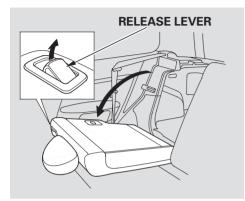
To unlatch either side of the seatback, pull up on the release lever, then fold the seat-back down. Make sure all items in the cargo area are secured. Loose items can fly forward and cause injury if you have to brake hard. See **Carrying Cargo** on page 117.
