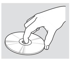
Handle a CD by its edges; never touch either surface. Do not place stabilizer rings or labels on the CD. These, along with contamination from fingerprints, liquids, and felt-tip pens, can cause the CD to not play properly, or possibly jam in the drive. If you see an error message in the display while playing a CD, find the cause in the chart to the right. If you cannot clear the error message, take your vehicle to your dealer.
