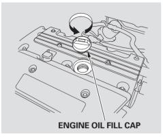
Unscrew and remove the engine oil fill cap on top of the valve cover. Pour in the oil slowly and carefully so you do not spill. Clean up any spills immediately. Spilled oil could damage components in the engine compartment. Install the engine oil fill cap, and tighten it securely. Wait a few minutes, and recheck the oil level. Do not fill above the upper mark; you could damage the engine.
