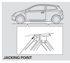
7. Place the jack under the jacking point. Turn the end bracket clockwise until the top of the jack contacts the jacking point. Make sure the jacking point tab is resting in the jack notch.
