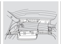
2. Put your fingers between the interior trim and the hatch glass on either side of the high-mount brake light. Carefully pull down on the trim to unsnap the clips from the hatch. Work your way toward each end of the trim. Remove the trim.
