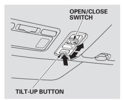
There are two switches on the ceiling near the front ceiling light. The ignition switch must be in the ON (II) position to operate the moonroof. To open the moonroof, pull back the moonroof switch firmly.
