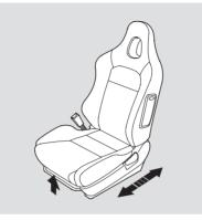
To adjust the seat forward and backward, pull up on the bar under the seat cushion's front edge. Then try to move the seat to make sure it is locked in position.
