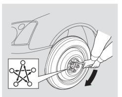
13. Tighten the wheel nuts securely in the same crisscross pattern. Have the wheel nut torque checked at the nearest automotive service facility.
