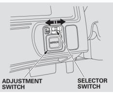
1. Move the selector switch to L (driver's side) or R (passenger's side).
