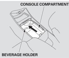
To access the console compartment, slide the lid forward, then slide the beverage holder assembly forward.
