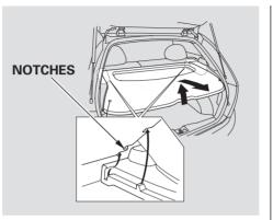
To install the cargo area cover, place it in its normal position over the cargo area. Then push down on each front corner to snap it in place. Lift up the rear of the cover, then reconnect the cables to the hatch. Your vehicle's windows are electrically-powered. Turn the ignition switch to ON (II) to raise or lower any window.
