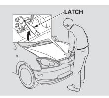
If the hood latch handle moves stiffly, or if you can open the hood without lifting the handle, the mechanism should be cleaned and lubricated.
