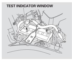
Check the condition of the battery monthly by looking at the test indicator window. The label on the battery explains the test indicator's colors. Check the terminals for corrosion (a white or yellowish powder). To remove it, cover the terminals with a solution of baking soda and water. It will bubble up and turn brown. When this stops, wash it off with plain water. Dry off the battery with a cloth or paper towel. Coat the terminals with grease to help prevent further corrosion.
