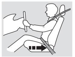
Adjust the driver's seat as far to the rear as possible while allowing you to maintain control of the vehicle. Have a front passenger adjust their seat as far to the rear as possible.
