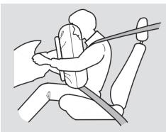
If you ever have a moderate to severe frontal collision, sensors will detect the vehicle's rapid deceleration. If the rate of deceleration is high enough, the control unit will instantly inflate the driver's and front passenger's front airbags, at the time and with the force needed. During a frontal crash, your seat belt restrains your lower body and torso, and the airbag helps protect your head and chest.
