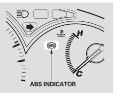
If the ABS indicator comes on, the anti-lock function of the braking system has shut down. The brakes still work like a conventional system, but without anti-lock. You should have a dealer inspect your vehicle as soon as possible.
