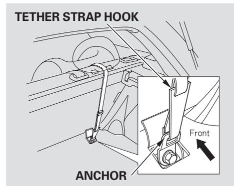
1. After properly securing the child seat (see page 37), lift the head restraint, then route the tether strap over the seat-back and through the head restraint legs.
