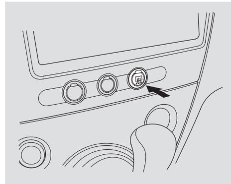
The rear window defogger will clear fog, frost, and thin ice from the window. Push the defogger button to turn it on and off. The indicator above the button comes on to show the defogger is on. If you do not turn it off, the defogger will shut itself off after about 15 minutes. It also shuts off when you turn off the ignition switch. You have to turn the defogger on again when you restart the vehicle.
