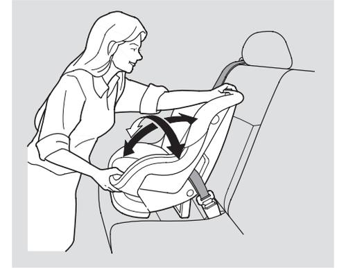
5. Push and pull the child seat forward and from side to side to verify that it is secure enough to stay upright during normal driving maneuvers. If the child seat is not secure, unlatch the belt, allow it to retract fully, then repeat these steps to deactivate the locking mechanism and remove a child seat, unlatch the buckle, unrout the seat belt, and let the belt fully retract.
