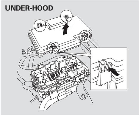
The under-hood fuse box is located in the back of the engine compartment on the left side. To open it, push the tabs as shown.
