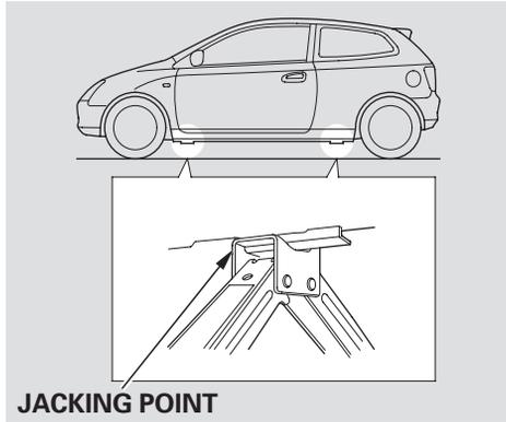
7. Place the jack under the jacking point. Turn the end bracket clockwise until the top of the jack contacts the jacking point. Make sure the jacking point tab is resting in the jack notch.
