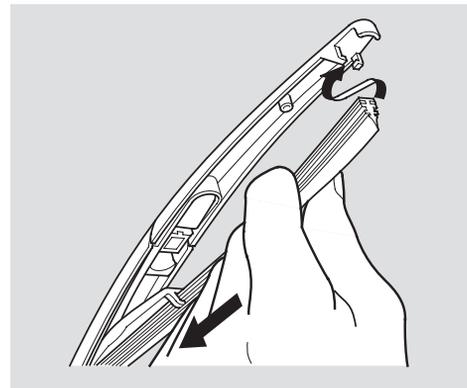
6. Insert both ends of the blade into the holder. Make sure they are secure.
