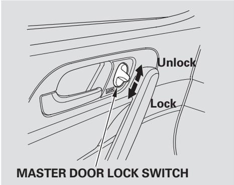
All doors lock when you push down the lock tab on the driver's door, or lock the driver's door from the outside with the key. Only the driver's door unlocks when you use the key or lock tab. To unlock the passengers' doors, use the master door lock switch or the lock tab on each door.
