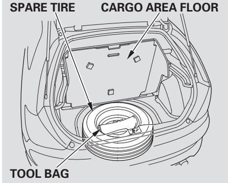
3. Open the hatch. Raise the cargo area floor by lifting up on the back edge.
