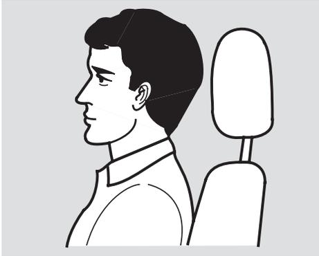
Have passengers with adjustable head restraints adjust their restraint so the back of their head rests against the center of the restraint. Taller persons should adjust their restraint as high as possible.
