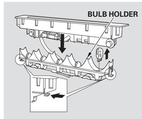
3. Remove the bulb holder from the light assembly by pushing the tabs on both sides and pulling the bulb holder down.
