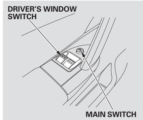
The driver's door armrest has a master power window control panel. To open the passenger's window, push down on the appropriate switch and hold it until the window reaches the desired position. To close the window, pull back on the window switch. Release the switch when the window gets to the position you want.
