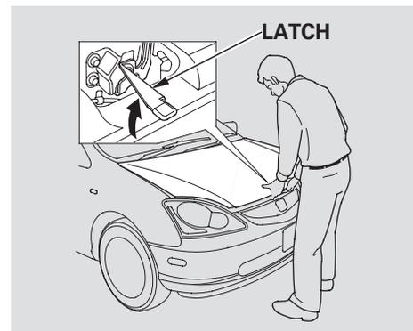
If the hood latch handle moves stiffly, or if you can open the hood without lifting the handle, the mechanism should be cleaned and lubricated.
