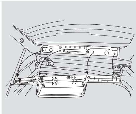
2. Put your fingers between the interior trim and the hatch glass on either side of the high-mount brake light. Carefully pull down on the trim to unsnap the clips from the hatch. Work your way toward each end of the trim. Remove the trim.
