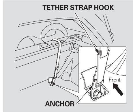
5. Lift the rear head restraint (see page 72 ), then route the tether strap over the seat-back between the legs of the head restraint, making sure the strap is not twisted.
