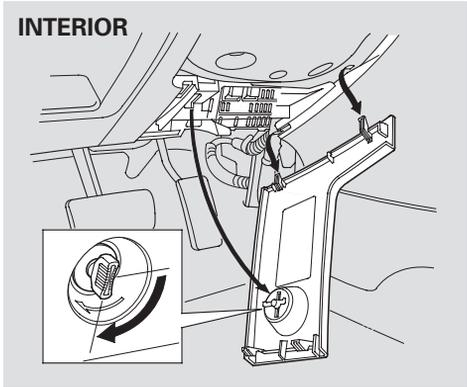
The vehicle's fuses are contained in two fuse boxes. The interior fuse box is located underneath the steering column. To open it, turn the knobs as shown.
