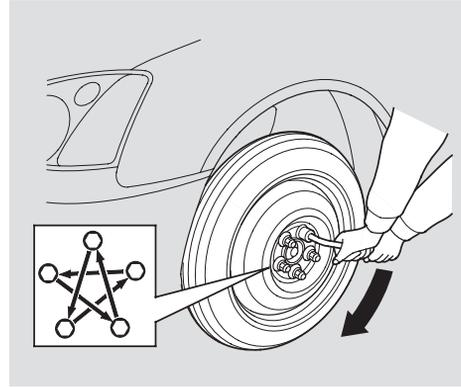
13. Tighten the wheel nuts securely in the same crisscross pattern. Have the wheel nut torque checked at the nearest automotive service facility.
