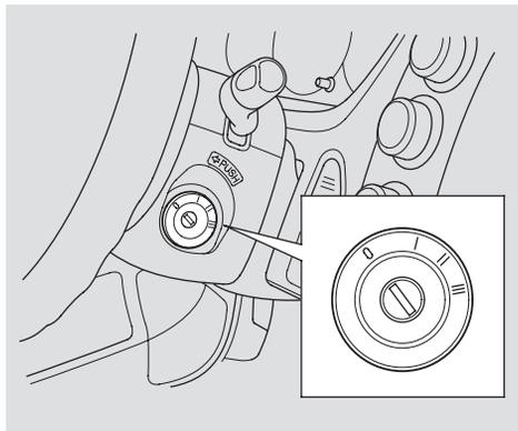
The ignition switch has four positions: LOCK (0), ACCESSORY (I), ON (II), and START (III).
