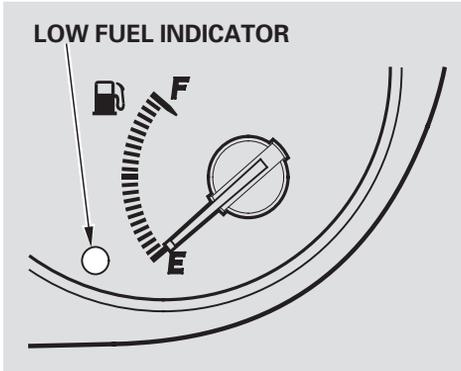
This indicator is located in the fuel gauge. If the indicator comes on, it means you should refuel soon.
