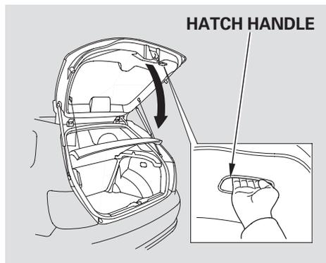
To close the hatch, use the hatch handle to lower the hatch, then press down on the back edge.
