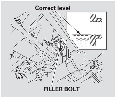
Check the fluid level with the transmission at normal operating temperature and the vehicle sitting on level ground. Remove the transmission filler bolt, and carefully feel inside the bolt hole with your finger. The fluid level should be up to the edge of the bolt hole. If it is not, add Honda Manual Transmission Fluid (MTF) until it starts to run out of the hole. Reinstall the filler bolt, and tighten it securely.
