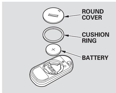
If it takes several pushes on the button to lock or unlock the doors and the hatch, replace the battery as soon as possible.
