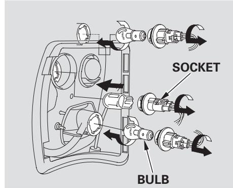
3. Determine which bulb, stop/taillight, back-up light, or turn signal is burned out.
