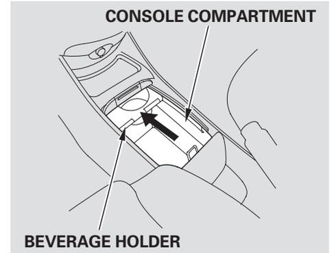
To access the console compartment, slide the lid forward, then slide the beverage holder assembly forward.
