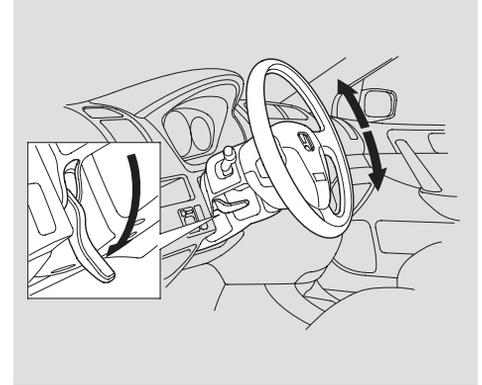
2. Move the steering wheel up or down to the desired position. Make sure you can see the instrument panel gauges and the indicators.
