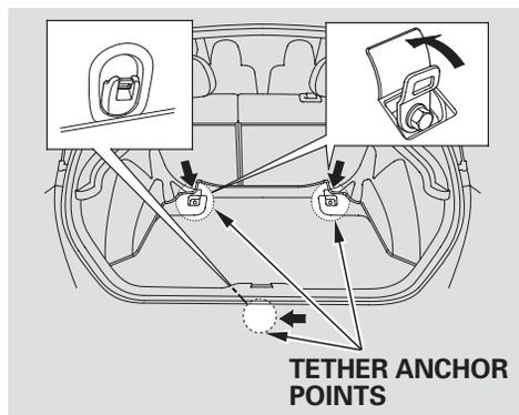
One tether anchor point for each of the outer rear seats is located under the cargo floor carpet and the tailgate sill. Pull up the carpet to access the anchor point (outboard anchor) when securing a tether-style child seat to the vehicle.
