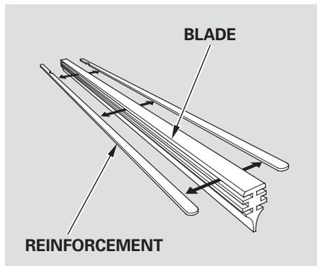
4. Examine the new wiper blade. If it has no plastic or metal reinforcement along the back edge, remove the metal reinforcement strips from the old wiper blade and install them in the slots along the edge of the new blade.
