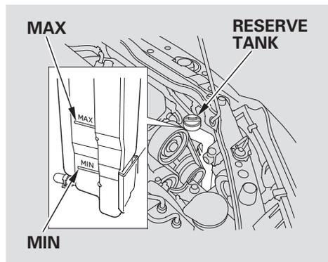
Look at the coolant level in the radiator reserve tank. Make sure it is between the MAX and MIN lines. If it is below the MIN line, see **Adding Engine Coolant** on page [141](#) for information on adding the proper coolant.
