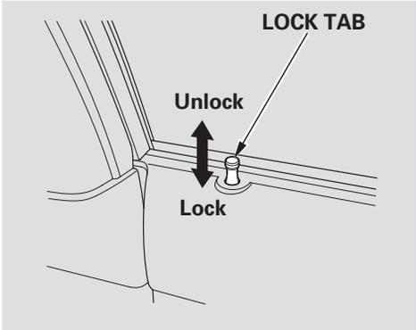
Each door has a lock tab on the top. When you push down the lock tab on the driver's door, both doors and the hatch lock. When you push down the lock tab on the passenger's door, only that door locks.
