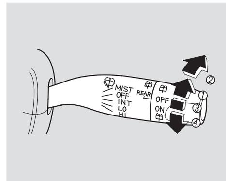
1. Rotate clockwise to turn the rear window wiper ON.
