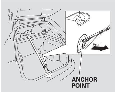
1. After properly securing the child seat (see page [40](#)), route the tether strap over the top of the seat-back.
