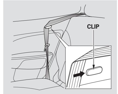
Before folding down the seat-back, move the seat belt out of the way and put the shoulder part of the outside seat belt in the clip on each side.
