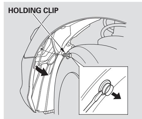
2. Use a flat-tipped screwdriver to remove the holding clip from the inner fender.
