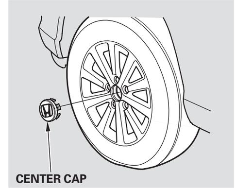
14. Remove the center cap before storing the flat tire in the spare tire well.
