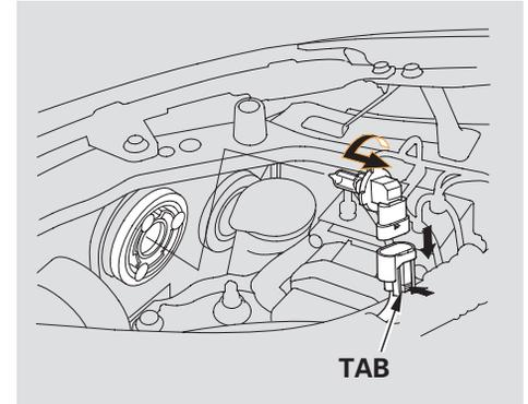
1. When you replace the bulb on the driver's side, if necessary, loosen the bolt on the battery plate, then slide the battery.
