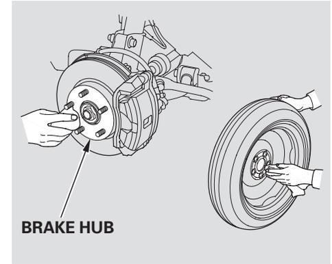
10. Before mounting the spare tire, wipe any dirt off the mounting surface of the wheel and hub with a clean cloth. Wipe the hub carefully; it may be hot from driving.
