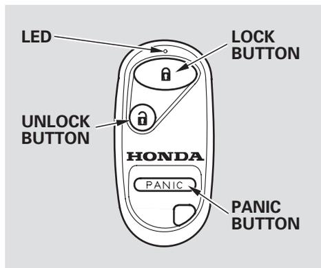
**LOCK** – Press this button once to lock both doors and hatch. Some exterior lights will flash. When you push LOCK twice within 5 seconds, you will hear a beep to verify that the doors are locked. You cannot lock it if any door is not fully closed or the key is in the ignition switch.
