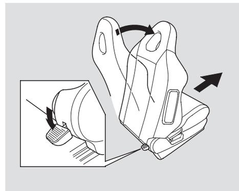
To get into the rear seat on the driver's side, pull up on the seat-back adjustment lever.
