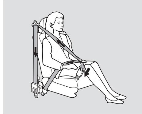
For added protection, the front seat belts are equipped with automatic seat belt tensioners. When activated, the tensioners immediately tighten the belts to help hold the driver and a front passenger in place.
