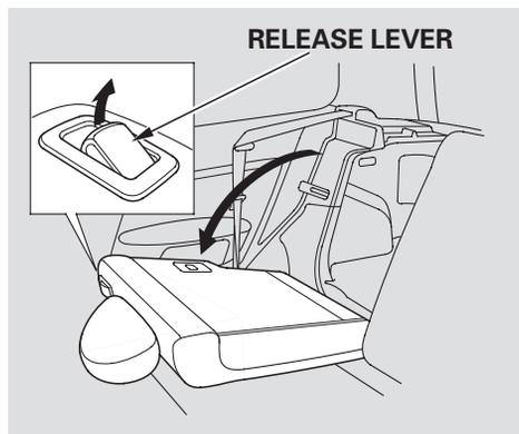
To unlatch either side of the seat-back, pull up on the release lever, then fold the seat-back down.
