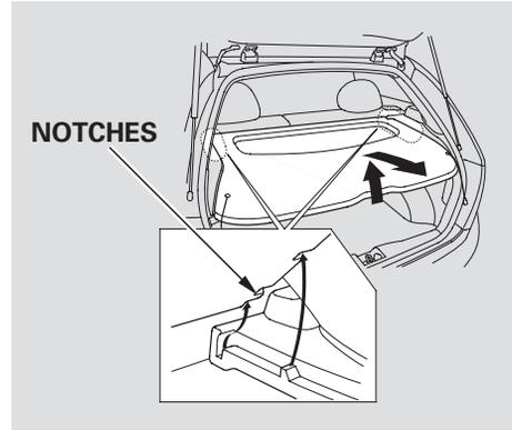
To install the cargo area cover, place it in its normal position over the cargo area. Then push down on each front corner to snap it in place. Lift up the rear of the cover, then reconnect the cables to the hatch.
