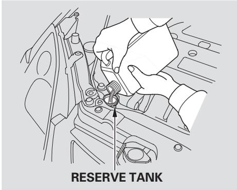
If the coolant level in the reserve tank is at or below the MIN line, add coolant to bring it up to between the MIN and MAX lines. Inspect the cooling system for leaks.
