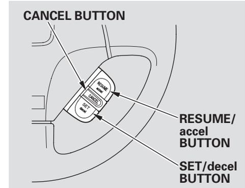
3. Press and release the SET/decel button on the steering wheel. The indicator on the instrument panel comes on to show the system is now activated.
