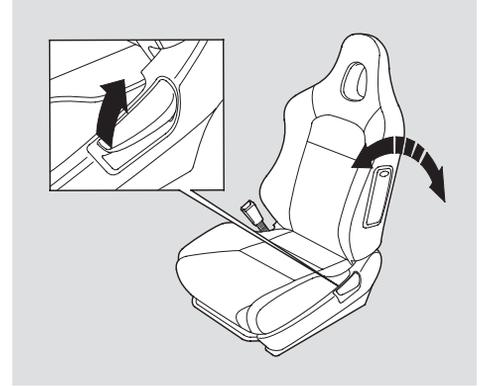
To change the seat-back angle of the front seat, pull up on the lever on the outside of the seat bottom.
