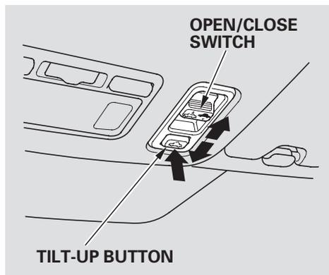
There are two switches on the ceiling near the front ceiling light. The ignition switch must be in the ON (II) position to operate the moonroof.
