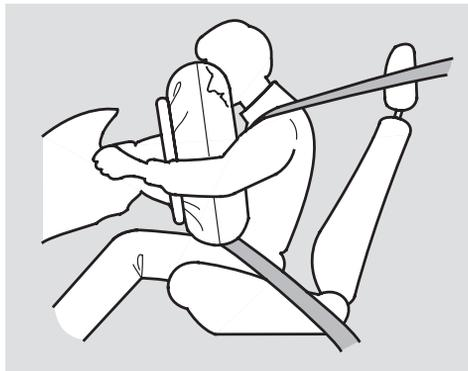
If you ever have a moderate to severe frontal collision, sensors will detect the vehicle's rapid deceleration. If the rate of deceleration is high enough, the control unit will instantly inflate the driver's and front passenger's front airbags, at the time and with the force needed.
