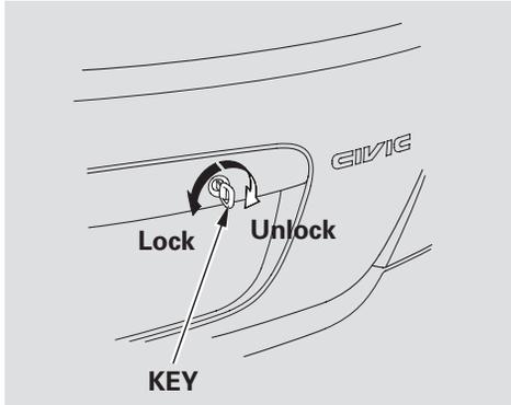
Use your key to lock and unlock the hatch. You can also lock and unlock the hatch with the remote transmitter or the master door lock switch.
