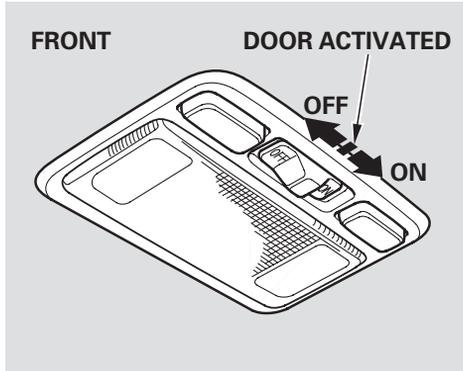
The ceiling light has a three-position switch: ON, Door Activated, and OFF.
