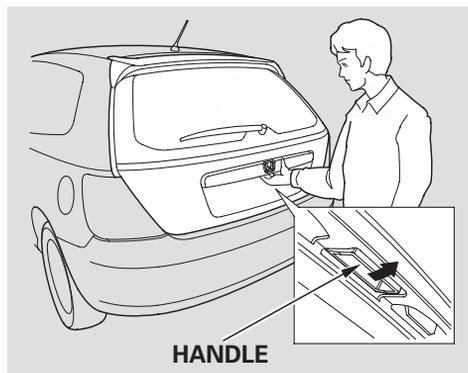
To open the hatch, pull the handle, then lift up.
