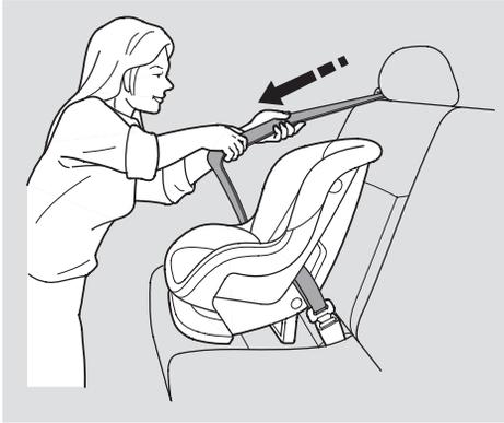
2. To activate the lockable retractor, slowly pull the shoulder part of the belt all the way out until it stops, then let the belt feed back into the retractor.
