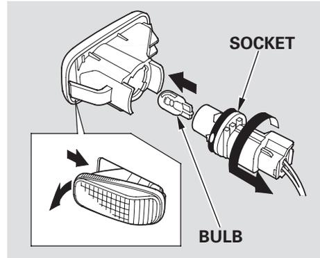
1. Push the front of the side turn signal assembly toward the rear of the vehicle until it pops out of the body.
