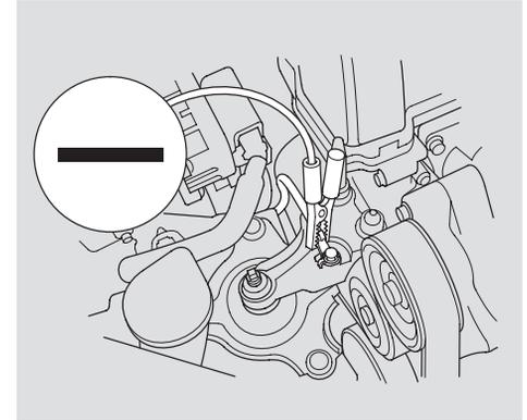
4. Connect the second jumper cable to the negative (–) terminal on the booster battery. Connect the other end to the grounding strap as shown. Do not connect this jumper cable to any other part of the engine.
