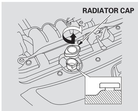
1. When the radiator and engine are cool, relieve any pressure in the cooling system by turning the radiator cap counterclockwise, without pressing down.
