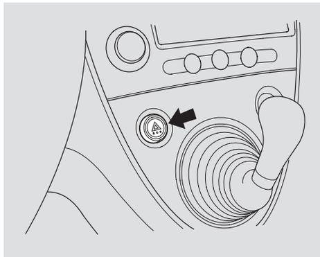
Push the red button to turn on the hazard warning lights (four-way flashers). This causes all four outside turn signals and both indicators in the instrument panel to flash. Use the hazard warning lights if you need to park in a dangerous area near heavy traffic, or if your vehicle is disabled.
