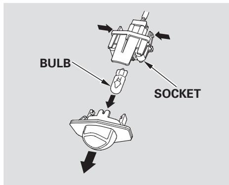
2. Remove the lens from the socket by pulling the lens while squeezing the tabs on both sides of the socket.
