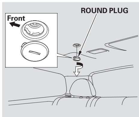
4. Use a screwdriver or coin to remove the round plug in the center of the headliner.
