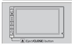
Press the (Eject/CLOSE) button to open the screen.
