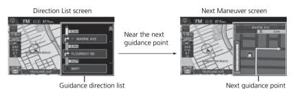
• **3** (Next Maneuver): Displays the map and next guidance point simultaneously on the map screen.
