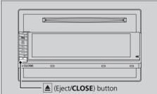
Press the (Eject/CLOSE) button to return the screen to the upright position.
