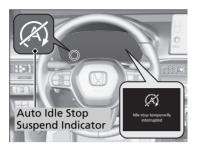
The Auto Idle Stop suspend indicator comes on and a message appears on the driver information interface when the Auto Idle Stop system cannot be activated.
