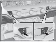
Press the seat heater button: Once - The HI setting (three indicators on) Twice - The MID setting (two indicators on)
