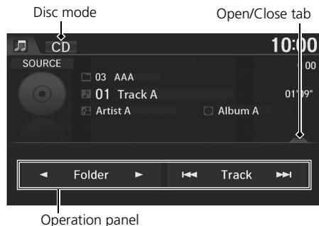
1. Select the open/close tab on the operation panel to display the track list.
