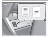
Install the device USB connector or the USB flash drive to the USB port.
