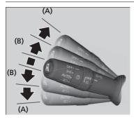
The turn signals can be used when the ignition switch is in ON  $[II]^{*1}$ .
