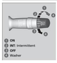
The rear wiper and washer can be used when the ignition switch is in ON  $[II]^{*1}$ .
