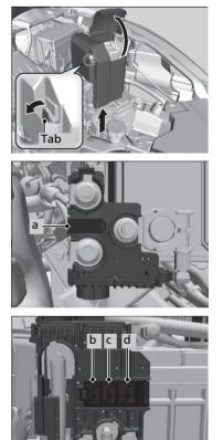
Pull up the cover on the  $\oplus$  terminal, then remove it while pulling out the tab as shown.
