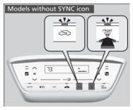
Select the reference icon to turn the air conditioning system on and automatically switch the system to fresh air mode.
