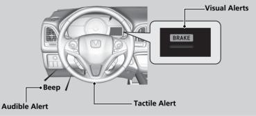
You can change the distance (**Long/Normal/Short**) between vehicles at which the system's earliest collision alert will come on through audio/information screen setting options.
