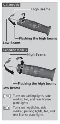
Rotating the light switch turns the lights on and off, regardless of the power mode setting or position of the ignition switch.
