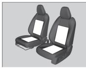
The ignition switch must be in ON  $\boxed{II}^{*1}$  to use the seat heaters.
