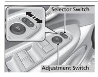
You can adjust the door mirrors when the ignition switch is in ON  $[II]^{*1}$ .
