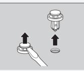
Insert the clip with the center pin raised, and push until it is flat.
