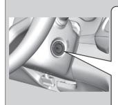
O LOCK: Insert and remove the key in this position.
