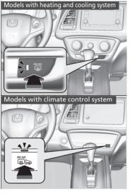
Press the rear defogger button or touch the icon to defog the rear window and mirrors<sup>\*</sup> when the ignition switch is in ON  $[I]^{*1}$ .
