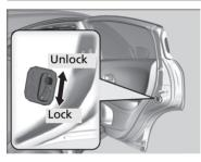
Slide the lever in the rear door to the lock position, and close the door.
