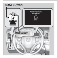
Press the RDM button to turn the system on and off.
