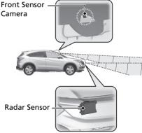
The radar sensor is in the front grille.
