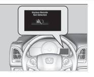
When the power mode is set to any mode other than OFF and you remove the smart entry remote from the vehicle and shut the door, an alarm will sound. If the alarm continues to sound, place the smart entry remote in another location.
