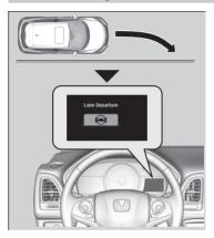
The front camera behind the rearview mirror monitors left and right lane markings (in white or yellow). If your vehicle is getting too close to detected lane markings without a turn signal activated, the system, in addition to a visual alert, applies steering torque and alerts you with rapid vibrations on the steering wheel, to help you remain within the detected lane.
