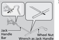
**3.** Raise the vehicle, using the jack handle bar and the jack handle, until the tire is off the ground.
