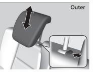
A passenger sitting in a back seating position should adjust the height of their head restraint to an appropriate position before the vehicle begins moving. **To raise the head restraint:** Pull it upward. **To lower the head restraint:** Push it down while pressing the release button.
