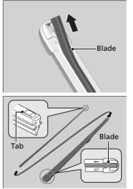
**3.** Slide the wiper blade out of the holder by pulling the tabbed end out.
