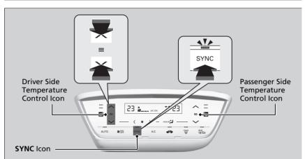
You can set the temperature synchronously for the driver side and the passenger side in synchronization mode.
