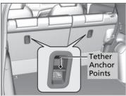
A tether anchor point is provided behind the rear outer seating positions and in the ceiling for the rear center. If you have a child seat that comes with a tether but can be installed with a seat belt, the tether may be used for additional security.
