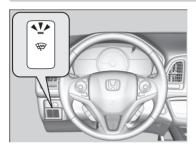
Press the heated windshield button to deice the windshield when the ignition switch is turned to ON  $\boxed{II}^{*1}$ .
