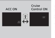
Press and hold the 🖹 (interval) button for one second. **Cruise Mode Selected** appears on the multi-information display for two seconds, and then the mode switches to Cruise. To switch back to ACC, press and hold the 🖺 (interval) button again for one second. **ACC Mode Selected** appears on the multiinformation display for two seconds.
