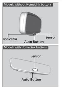
When you are driving after dark, the automatic dimming rearview mirror reduces the glare from headlights behind you. Press the auto button to turn this function on and off. When activated, the auto indicator comes on. Automatic Dimming Rearview Mirror\*
