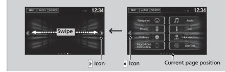
Selecting  $\langle\!\!\langle$  or  $\rangle\!\!\rangle$ , or swiping the screen left or right changes to the next screen.
