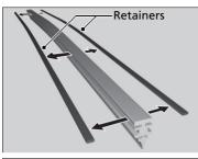
**4.** Remove the retainers from the rubber blade that has been removed, and mount to a new rubber blade.
