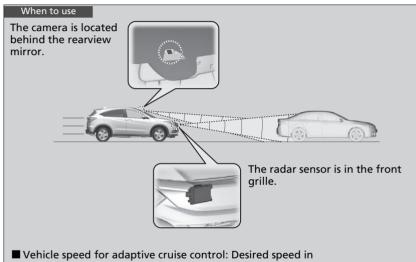
Venicle speed for adaptive cruise control: Desired speed for a range above roughly 25 mph (40 km/h) ~
