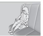
If a lap/shoulder seat belt cannot be used properly, position the child in a booster seat in a rear seat. For the child's safety, check that the child meets the booster seat manufacturer's recommendations.
