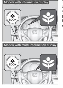
The **ECON** button turns the ECON mode on and off. The ECON mode helps you improve your fuel economy by adjusting the performance of the engine, transmission, heating and cooling system\*/climate control system\*, and cruise control\*.
