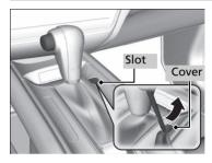
Shift Lock Release Slot Release Button
