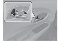
Unlocking and opening the driver's door from the inner handle unlocks all the other doors.
