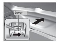
**3.** To open the tailgate, push the tailgate while sliding the lever to the right.
