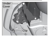
**1.** Remove the clips using a flat-tip screwdriver, and push up the under cover.
