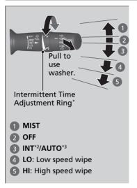
The windshield wipers and washers can be used when the ignition switch is in ON  $[II]^{*1}$ .
