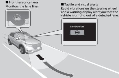
When you operate the turn signals to change lanes, the system is suspended, and resumes after the signals are off.
