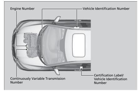
Vehicle Identification Number (VIN), Engine Number, and Transmission Number
