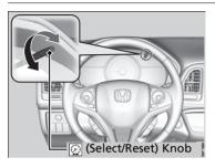
When the ignition switch is in ON II \*1, you can use the (2) (select/reset) knob to adjust instrument panel brightness. Brighten: Turn the knob to the right. Dim: Turn the knob to the left.
