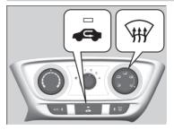
Selecting turns the air conditioning system on and automatically switches the system to fresh air mode.
