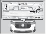
**3.** Push the hood latch lever (located under the front edge of the hood on the driver's side) to the side and raise the hood. Once you have raised the hood slightly, you can release the lever.
