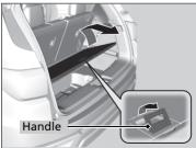
**3.** Pull the rear edge of the handle on the floor lid and remove the lid.
