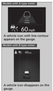
Your vehicle maintains the set speed without having to keep your foot on the brake or accelerator pedal.
