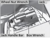
**2.** Take the jack, wheel nut wrench, jack handle bar, and box wrench out of the tool case.
