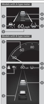
You can see the current state of Adaptive Cruise Control (ACC) with Low Speed Follow, Lane Keeping Assist System (LKAS) and Traffic Jam Assist.
