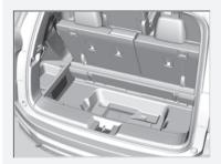
Seat must be secured with included seat storage strap when stored in this position.
