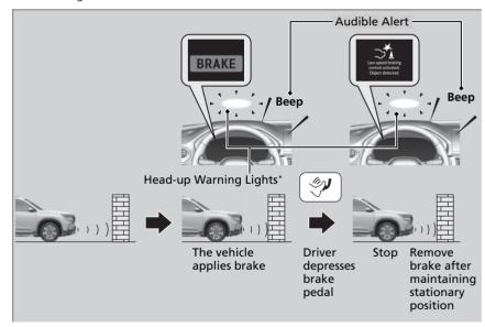
If the only rear sensors are turned off using the parking sensor system, the assistive braking will not work when reversing.
