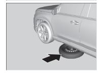
**10.** Place the spare tire (wheel side up) under the vehicle body, near the tire that needs to be replaced.
