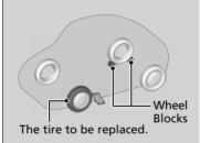
**9.** Place a wheel block or rock in front and rear of the wheel diagonal to the flat tire.
