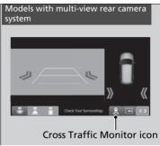
Tap to turn the system on and off. The indicator (green) comes on with the system on.
