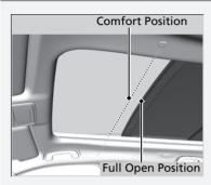
The panoramic roof cannot be fully opened in a single operation. The panoramic roof has a "comfort" position or wind noise reduction position at which the roof first stops. To open fully, pull the switch back again after the roof has stopped at this position.
