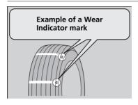
The groove where the wear indicator is located is about 1/16 inch (about 1.6 mm) shallower than elsewhere on the tire. If the tread has worn so that the indicator is exposed, replace the tire.
