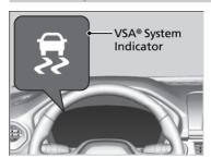
When VSA® activates, you may notice that the engine does not respond to the accelerator. You may also notice some noise from the hydraulic brake system. You will also see the indicator blink.
