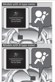
■ When the power mode is set to ON The indicator comes on for a few seconds, then goes off. This tells you the system is working properly.
