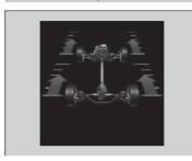
The indicators on the display show the amount of torque being transferred to the right front, left front, right rear, and left rear wheels.
