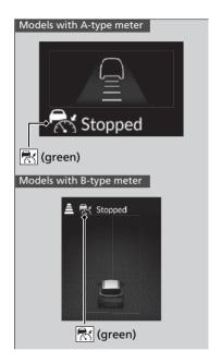
If no vehicle is ahead of you before you resume driving, depress the accelerator pedal and ACC with Low Speed Follow will operate again within the prior set speed.
