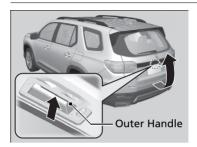
When all the doors are unlocked or you press the tailgate unlock button\* on the remote transmitter, the tailgate is unlocked.
