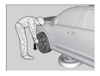
**11.** Loosen each wheel nut about one turn using the wheel nut wrench.
