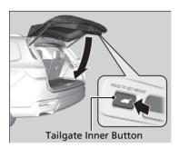
Press the tailgate inner button on the tailgate to close the power tailgate.
