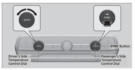
You can set the temperature synchronously for the driver's side, passenger's side and rear in synchronization mode.
