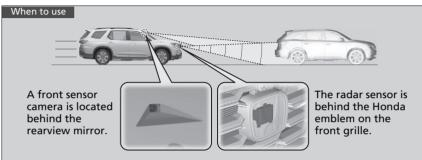
The system starts monitoring the roadway ahead when your vehicle speed is about 3 mph (5 km/h) or above and will search for a vehicle, pedestrian, or moving bicycle in front of you.
