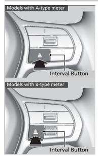
Press the Interval button to change the ACC with Low Speed Follow following-interval. Each time you press the button, the following-interval (the interval behind a vehicle detected ahead of you) setting cycles through furthest, far, mid, and nearest following-intervals.
