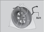
4. Bore through the bag, and pass the holding belt through the hole of the bag and the wheel of the flat tire as shown.
