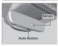
When you are driving after dark, the automatic dimming rearview mirror and power door mirror\* reduces the glare from headlights behind you. Press the AUTO button to turn this function on and off. When activated, the AUTO indicator comes on.
