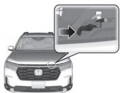
When finished, close the hood and make sure it is firmly locked in place.
