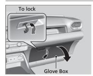
Pull the handle to open the glove box. You can lock the glove box with the built-in key.
