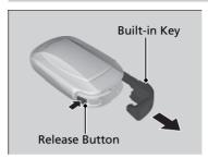
The built-in key can be used to unlock the doors when the keyless remote battery becomes weak and the power door unlock operation is disabled.
