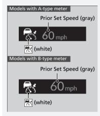
The set speed cannot be set or resumed when ACC with Low Speed Follow has been turned off using the button. Press the button to activate the system, then set the desired speed.
