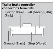
Have a qualified mechanic install your trailer brake controller following the trailer brake controller manufacturer's instructions. Failure to properly install the trailer brake controller may increase the distance it takes for you to stop your vehicle when towing a trailer.
