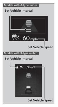
When ACC with Low Speed Follow starts operating, the vehicle icon, interval bars and set speed appear on the gauge.
