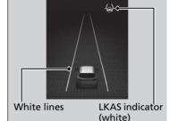
When the LKAS is suspended, green lines on the gauge change to white lines or disappear, and the beeper sounds (if activated).
