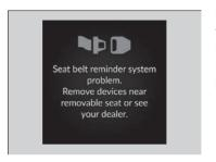
If the vehicle loses connection with the transceiver while the seat belt is fastened, the information for that seat will change to unfastened, and a "Seat belt reminder system problem" warning will be displayed.
