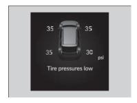
**Tire pressure low** is displayed when a tire has significantly low pressure. The specific tire is displayed on the screen.
