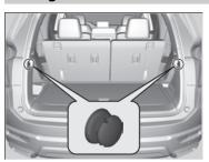
Use the cargo hooks to secure cargo in the cargo area.
