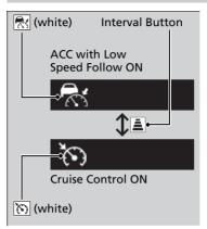
Press and hold the interval button for one second. **Cruise mode selected** appears on the driver information interface for two seconds, and then the mode switches to Cruise.
