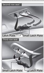
**1.** Pull out the seat belt's small latch plate and the latch plate from each holding slot in the ceiling.
