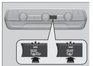
The rear defogger and heated door mirrors\* automatically switch off after 10-30 minutes depending on the outside temperature.
