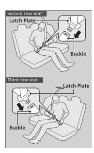
**3.** Insert the latch plate into the buckle. Properly fasten the seat belt the same way you fasten the lap/shoulder seat belt.
