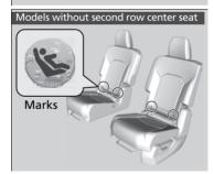
**1.** Locate the lower anchors under the marks.
