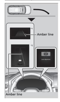
The front camera behind the rearview mirror monitors left and right lane markings in white or yellow, the outer edge of the pavement (bordered by grass or gravel) or a detected oncoming vehicles.
