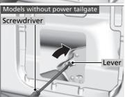
**2.** To open the tailgate, push the tailgate while pushing the lever to the right with the flat-tip screwdriver.
