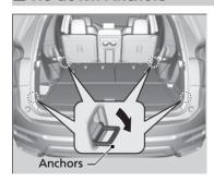
The tie-down anchors on the cargo area floor can be used to install a net for securing items.
