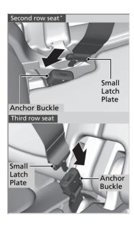
**2.** Line up the triangle marks on the small latch plate and anchor buckle. Make sure the seat belt is not twisted. Attach the belt to the anchor buckle.
