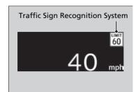
Traffic Sign Recognition System: Shows certain detected traffic signs while driving. If speed limit warning is activated, the sign icon blinks when the maximum speed of the traffic sign detected is exceeded by a threshold, when compared with the vehicle speed.
