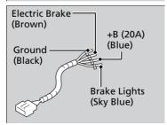
The trailer hitch harness is used to install the controller for the electric trailer brakes. Insert the trailer brake fuse into the engine compartment fuse box.
