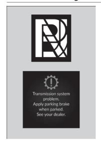
■ Reasons for the indicator to blink The transmission is malfunctioning.
