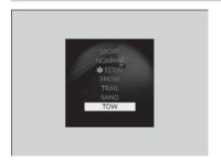
Optimizes balance between driving performance and comfort when towing a trailer
