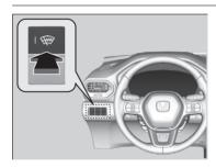
Press the heated windshield button to deice the windshield at the wiper park area of the windshield when the power mode is in ON. The heated windshield will automatically switch off after 15 minutes
