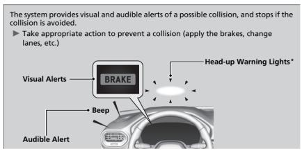
You can change the distance (**Long/Normal/Short**) between vehicles at which the system's earliest collision alert will come on.
