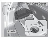
**1.** Turn the knobs counter-clockwise to remove the tool case cover.
