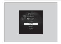
Maximizes controllability on roads with mud, gravel, or loose dirt.
