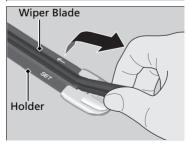
**6.** Pull the wiper blade in the opposite direction to slide it out of the holder.
