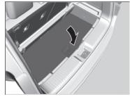
**3.** Push the far end of the lid down to the bottom of the under-floor storage area, then pull the handle and lower the other end.
