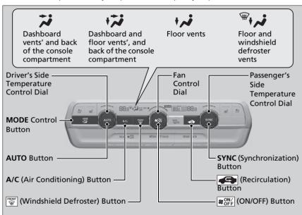
Use the system when the engine is running.
