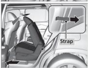
Pulling up on the strap also tilts the seat-back forward.
