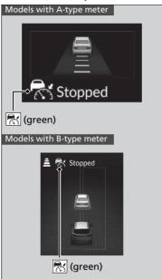
Your vehicle also stops automatically. The **Stopped** message appears on the gauge. When the vehicle ahead of you starts again, if you press the **RES/+/SET/-** switch up or down, or depress the accelerator pedal, ACC with Low Speed Follow operates again within the prior set speed.
