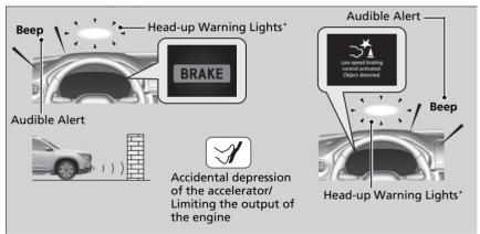
Assistive driving power suppression will not activate in the following situations. When moving forward:
