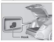
The cargo hook in the cargo area can be used to hang a light items.
