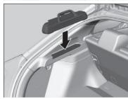
The housing can be installed on either side of the cargo area.
