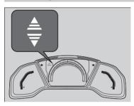
Come on to inform you that upshifting or downshifting is necessary to prevent the engine from over revving or stalling.
