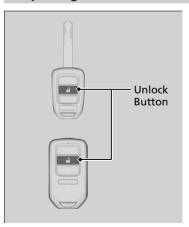
**To open:** Press the unlock button, and then within 10 seconds, press it again and hold it.
