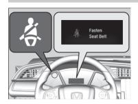
The seat belt system includes an indicator on the instrument panel to remind the driver or a front passenger or both to fasten their seat belts. If the ignition switch is turned to ON  $\overline{\mathrm{III}}^{*1}$  and a seat belt is not fastened, a beeper will sound and the indicator will blink. After a few seconds, the beeper will stop and the indicator will come on and remain illuminated until the seat belt is fastened.
