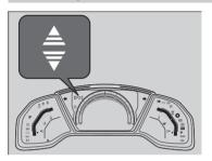
Come on while the vehicle is in the 7-speed manual shift mode to indicate when a speed position change is appropriate to maintain the most fuel efficient driving style.
