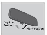
Flip the tab to switch the position.
