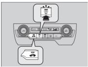
Pressing the (windshield defroster) button turns the air conditioning system on and automatically switches the system to fresh air mode.
