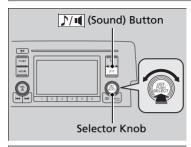
Press the (Sound) button, and rotate to scroll through the following choices:
