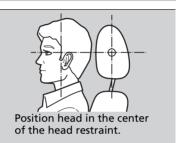
Front head restraints are most effective for protection against whiplash and other rearimpact crash injuries when the center of the back of the occupant's head rests against the center of the restraint. The tops of the occupant's ears should be level with the center height of the restraint.
