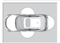
When you carry the smart entry remote, you can lock/unlock the doors and hatch. You can lock/unlock the doors and hatch within a radius of about 32 inches (80 cm) of the outside door handle or hatch release button.
