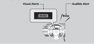
At system's earliest collision alert stage, you can change the distance (**Long/Normal/Short**) between vehicles at which alerts will come on through driver information interface\* or audio/information screen\* setting options.
