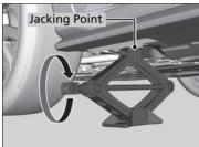
**2.** Turn the end bracket (as shown in the image) clockwise until the top of the jack contacts the jacking point.
