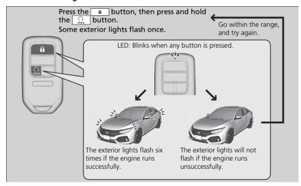
When started remotely, the engine automatically shuts off after 10 minutes of idling and/or the brake pedal and **ENGINE START/STOP** button have not been pressed simultaneously.
