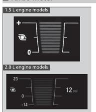
When the turbo charger is producing boost, this meter shows the boost pressure.
