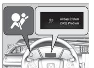
■ When the ignition switch is turned to ON ||||\*1
