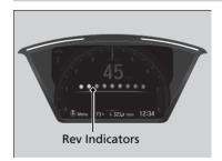
Light up from left to right according to engine speed.
