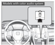
The rear defogger and heated door mirrors automatically switch off after 10-30 minutes depending on the outside temperature. However, if the outside temperature is 32°F (0°C) or below, it does not automatically switch off.
