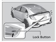
Press the door lock button on the front door or on the hatch.
