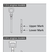
Upper Mark Lower Mark **4.** Remove the dipstick again, and check the level. It should be between the upper and lower marks. Add oil if necessary.
