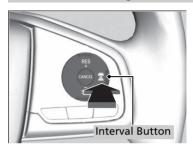
Press the (interval) button to change the ACC with LSF following-interval.
