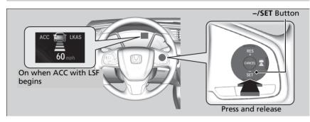
When driving at about 25 mph (40 km/h) or above: Take your foot off the pedal and press the –/SET button when you reach the desired speed. The moment you release the button, the set speed is fixed, and ACC with LSF begins.
