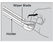
**4.** Pull the wiper blade in the opposite direction to slide it out of holder.
