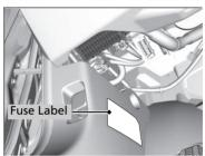
Fuse locations are shown on the label on the side panel. Locate the fuse in question by the fuse number and label number.
