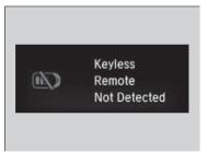
Warning buzzers may sound from inside and/ or outside the vehicle to remind you that the smart entry remote is out of the vehicle. If the buzzer continues even after the remote is put back inside, place it to be within its operational range.
