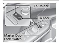
Press the master door lock switch in as shown to lock or unlock all the doors and the hatch.
