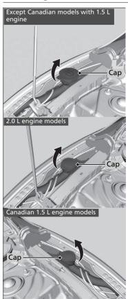
Open the cap and check the amount of window washer fluid.
