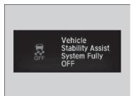
To completely disable VSA®, the VSA® must be in +R mode. Press and hold the VSA® OFF button until you hear a single beep, then later two more beeps.
