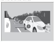
Three lines that appear on the screen can give an idea of how far the vehicles or objects on the screen are from your vehicle, respectively. If an object is near line 1 (in red), it indicates that it is close to your vehicle whereas an object near line 3 is farther away.
