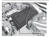
The condition of the battery is monitored by a sensor located on the negative terminal of the battery. If there is a problem with this sensor, the driver information interface will display a warning message. If this happens, have you vehicle inspected by a dealer.
