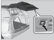
**2.** Press and hold the tailgate inner button until you hear short two beeps following one long buzzer.
