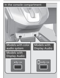
The USB port (1.0A) is for playing audio files on a USB flash drive, connecting a cellular phone, and charging devices.
