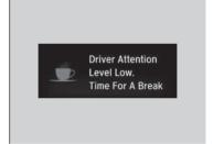
If one bar lights up, the **Driver Attention Level Low. Time For A Break** message will appear, a beep will sound, and the steering wheel will vibrate.
