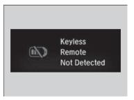
When the power mode is set to any mode other than OFF and you remove the smart entry remote from the vehicle and shut the door, an alarm will sound. If the alarm continues to sound, place the smart entry remote in another location.
