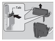
**4.** Pull out the fuse box inside the inner fender, then push the tabs to open the box.
