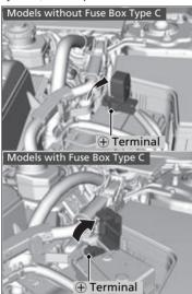
**1.** Open the terminal cover on your vehicle's 12-volt battery positive  $\oplus$  terminal.
