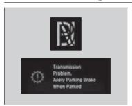
■ Reasons for the indicator to blink The transmission is malfunctioning.
