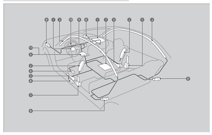
The front, side, and side curtain airbags are deployed according to the direction and severity of impact. Both side curtain airbags are deployed in a rollover. The airbag system includes:
