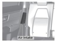
If the air intake is obstructed during vehicle operation, the High Voltage battery can become too hot. To protect the battery, the system may start to limit the battery's output and cause the power system and 12-volt battery charging system indicators to come on.
