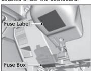
Fuse locations are shown on the label on the steering column lower cover. Locate the fuse in question by the fuse number and label number.
