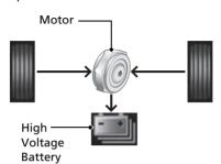
When decelerating without the accelerator being depressed or the brake pedal being applied, or while driving downhill, the electric motor acts as a generator that recovers a portion of the electrical energy that was used to accelerate the vehicle. This regenerative braking slows the vehicle in a manner similar to engine braking in a gasoline-powered vehicle. You can control the rate of deceleration by using the deceleration paddle selector.
