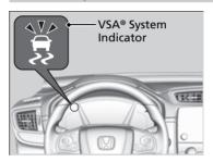
When VSA® activates, you may notice that the engine and motor do not respond to the accelerator. You may also notice some noise from the hydraulic brake system. You will also see the indicator blink.
