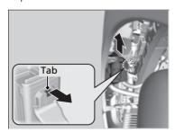
3. Pull the tab to remove the fuse box.
