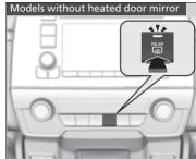
The rear defogger and heated door mirror\* automatically switch off after 10-30 minutes depending on the outside temperature. However, if the outside temperature is 32°F (0°C) or below, it does not automatically switch off.
