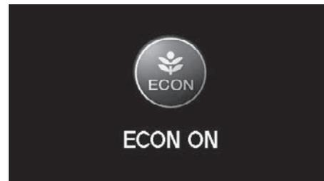
The message is displayed for a few seconds when the ECON button is pressed.
