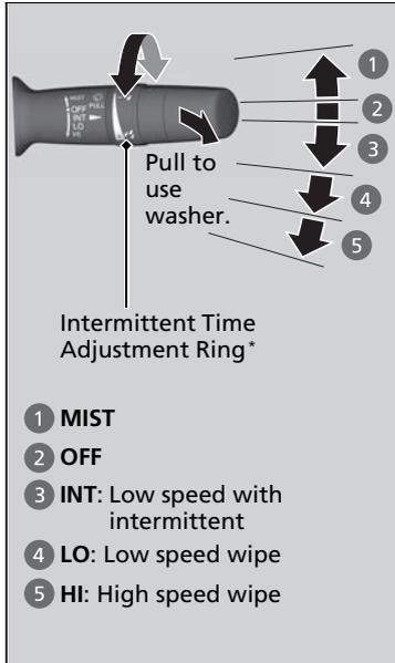
The windshield wipers and washers can be used when the ignition switch is in ON \*1.
