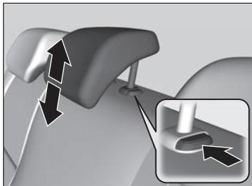
A passenger sitting in a back seating position should adjust the height of their head restraint to an appropriate position before the vehicle begins moving.
