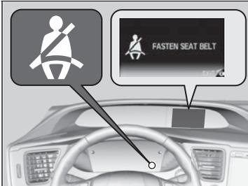
Your vehicle monitors front seat belt use. If the ignition switch is turned to ON **II**\*1 before the driver's seat belt is fastened, the beeper will sound and the indicator will blink. If the driver does not fasten the belt before the beeper stops, the indicator will remain on.
