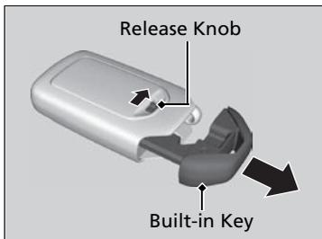
The built-in key can be used to lock/unlock the doors when the smart entry remote battery becomes weak and the power door lock/unlock operation is disabled.
