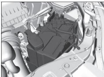
Check the battery terminals for corrosion monthly.
