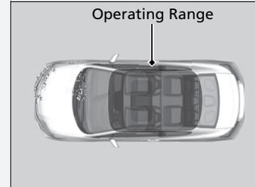
You can start the engine when the smart entry remote is inside the vehicle. The engine may also run if the smart entry remote is close to the door or window, even if it is outside the vehicle.
