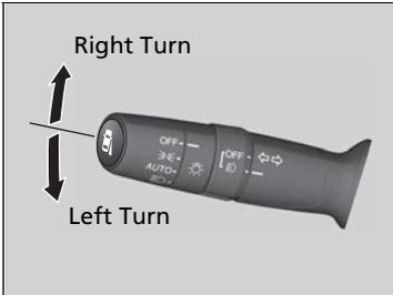
The turn signals can be used when the ignition switch is in ON
