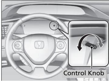
When the parking lights are turned on and the ignition switch is in ON
