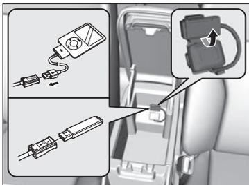
1. Lift the armrest and unclip the USB connector cable.
