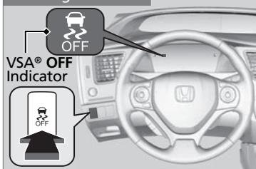
This button is on the driver side control panel. To turn the VSA® system on and off, press and hold it until you hear a beep.
