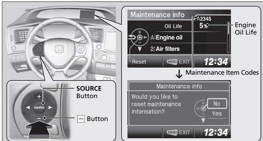
1. Turn the ignition switch to ON \*1.
