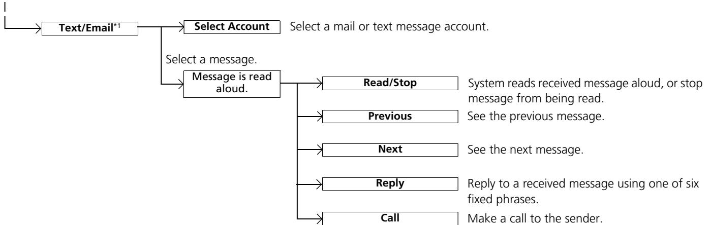
\*1: Appears only when a phone is connected to the system.
