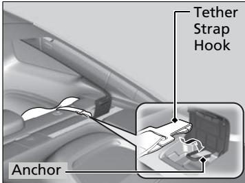
6. Open the tether anchor cover behind the head restraint.
