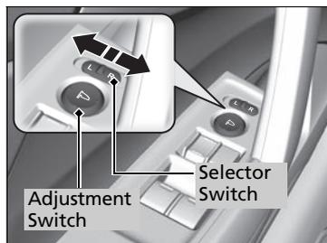
You can adjust the door mirrors when the ignition switch is in ON
