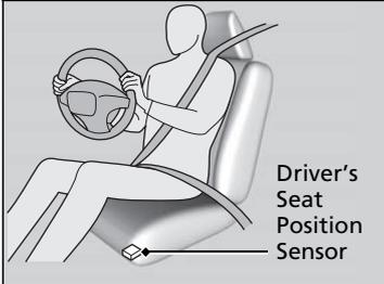
The driver's advanced front airbag system includes a seat position sensor.
