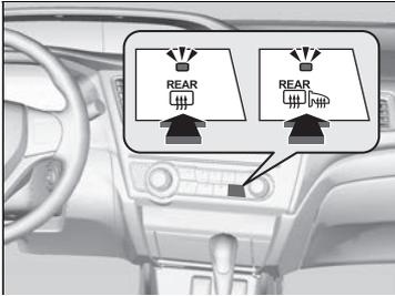
Press the rear defogger and heated door mirror button to defog the rear window and mirrors when the ignition switch is in ON
