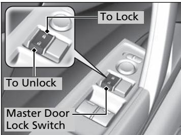
Press the master door lock switch in as shown to lock or unlock both doors.
