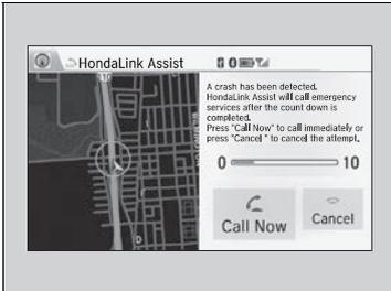
If your vehicle's airbags deploy or if the unit detects that the vehicle is severely impacted, your vehicle automatically will attempt to connect to the HondaLink operator. Once connected, information about your vehicle, its positioning, and its condition will be sent to the operator; you also can speak to the operator when connected.
