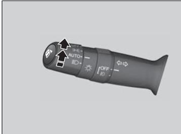
Automatic lighting control can be used when the ignition switch is in ON
