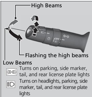
Rotating the light switch turns the lights on and off, regardless of the position of the ignition switch.
