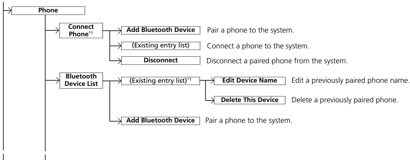
\*1: Appears only when a phone is connected to the system.
