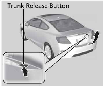
Press the release button on the trunk lid after the doors are unlocked.
