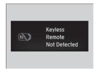
Warning buzzers may sound from inside and/ or outside the vehicle to remind you that the smart entry remote is out of the vehicle. If the buzzer continues even after the remote is put back inside, place it to be within its operational range.
