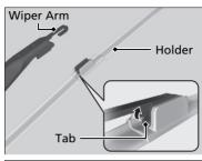
**4.** Press and hold the tab, then slide the holder off the wiper arm.
