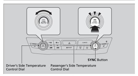
You can set the temperature synchronously for the driver's side and the passenger's side in synchronization mode.
