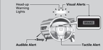
At system's earliest collision alert stage, you can change the distance (**Long/Normal/Short**) between vehicles at which alerts will come on through audio/information screen setting options.
