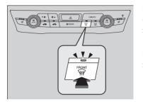
Pressing the button turns the air conditioning system on and automatically switches the system to fresh air mode.
