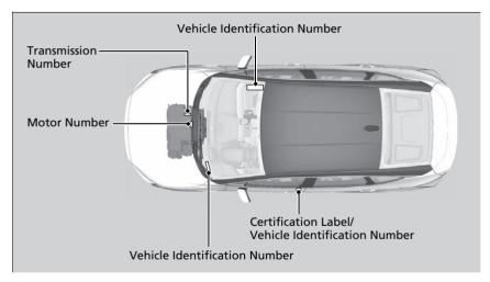
■Vehicle Identification Number (VIN), Motor Number, and Transmission Number
