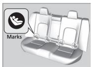
**1.** Locate the lower anchors under the marks
