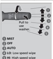
The windshield wipers and washers can be used when the power mode is in ON.
