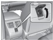
■ Accessory power socket (back of the console compartment)
