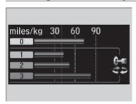
Shows the average fuel economy for the last three driving cycles (1 - 3), and the current driving cycle (0) in miles/kg or km/kg.
