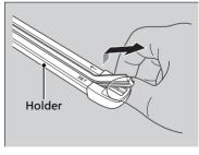
**6.** Pull the wiper blade in the opposite direction to slide it out of the holder.
