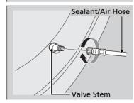
**3.** Attach the sealant/air hose onto the tire valve stem. Screw it until it is tight.
