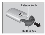
The built-in key can be used to lock/unlock the doors when the smart entry remote battery becomes weak and the power door lock/unlock operation is disabled.
