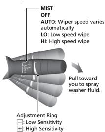
**AUTO** should always be turned **OFF** before the following situations in order to prevent severe damage to the wiper system:
