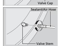
**6.** Attach the air only hose onto the tire valve stem. Screw it until it is tight.
