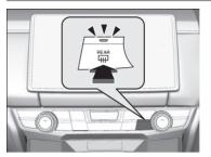
Press the rear defogger button to defog the rear window when the power mode is in ON.
