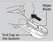
**5.** Pull the end of the wiper blade in the direction of the arrow in the image until it is out of the holder's end cap.
