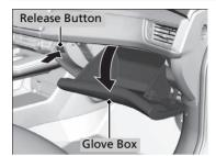
Press the release button to open the glove box.
