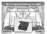
A tether anchorage point is provided behind each rear seating position.
