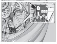
Pull up the cover on the ① terminal, then remove it while pulling out the tab as shown.
