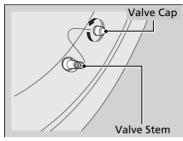
**1.** Remove the valve cap from the tire valve stem.
