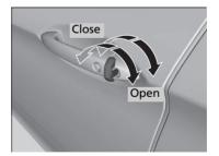
**To open:** Unlock the driver's door with the key. Within 10 seconds of returning the key to the central position, turn the key in the unlock direction and hold it there. **To close:** Lock the driver's door with the key. Within 10 seconds of returning the key to the central position, turn the key in the lock direction and hold it there.
