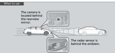
The system starts monitoring the roadway ahead when your vehicle speed is about 3 mph (5 km/h) and there is a vehicle in front of you.
