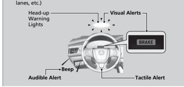
The system provides visual, audible and tactile alerts of a possible collision, and
