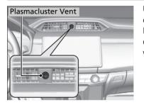
Using air flow generated by the climate control system or the fan blower, the Plasmacluster air purifier helps rid the interior of the vehicle of air-born bacteria and odors as well as inhibit mold growth.
