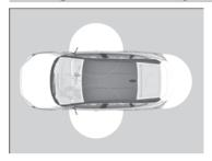
When you carry the smart entry remote, you can lock/unlock the doors and open the trunk. You can lock/unlock the doors within a radius of about 32 inches (80 cm) of the outside door handle or trunk release button.
