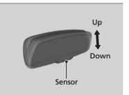
When you are driving after dark, the automatic dimming rearview mirror reduces the glare from headlights behind you, based on inputs from the mirror sensor. This feature is always active.
