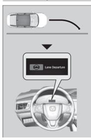
The front camera behind the rearview mirror monitors left and right lane markings (in white or yellow). If your vehicle is getting too close to detected lane markings without a turn signal activated, the system, in addition to a visual alert, applies steering torque and alerts you with rapid vibrations on the steering wheel, to help you remain within the detected lane.
