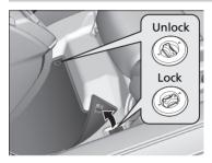
The front and rear floor mats hook over floor anchors, which keep them from sliding forward. To remove a mat for cleaning, turn the anchor knobs to the unlock position. When reinstalling the mat after cleaning, turn the knobs to the lock position.
