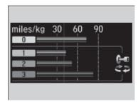
Shows the average fuel economy for the last three driving cycles (1 - 3), and the current driving cycle (0) in miles/kg or km/kg.
