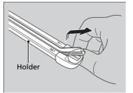
**6.** Pull the wiper blade in the opposite direction to slide it out of the holder.
