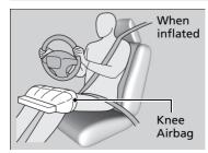
When the driver's front airbag inflates, the driver's knee airbag also inflates.
