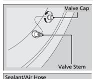
**1.** Remove the valve cap from the tire valve stem.
