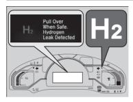
When the hydrogen leak indicator comes on, hydrogen gas is leaking. When a hydrogen gas leak is detected, the warning buzzer sounds, and warning indicator comes on. Follow the message displayed on the driver information interface and contact an authorized Honda Clarity Fuel Cell dealer.
