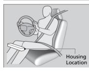
The driver's knee airbag is housed under the steering column.
