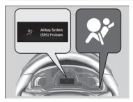
■ When the power mode is set to ON The indicator comes on for a few seconds, then goes off. This tells you the system is working properly. Supplemental Restraint System (SRS) Indicator
