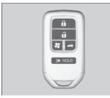
Use the keys to turn on and off the power system, and to lock and unlock the doors and to open the trunk. You can also use the remote transmitter to lock and unlock the doors and trunk.
