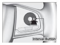
Press the 🖹 (interval) button to change the ACC with LSF following-interval. Each time you press the button, the following-interval (the interval behind a vehicle detected ahead of you) setting cycles through extra long, long, middle, and short following-intervals.
