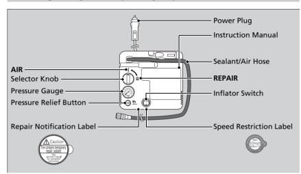
Setting Ready to Temporarily Repair the Flat Tire
