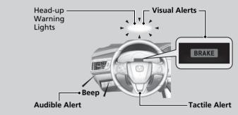
At system's earliest collision alert stage, you can change the distance (**Long/Normal/Short**) between vehicles at which alerts will come on through audio/information screen setting options.
