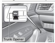
Pressing the trunk opener on the driver's door unlocks and opens the trunk.
