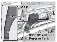
Inspect the coolant level, and check the cooling system components for leaks.
