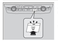
Pressing the witton turns the air conditioning system on and automatically switches the system to fresh air mode.
