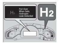
When the hydrogen leak indicator comes on, hydrogen gas is leaking.
