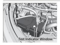
Check the battery condition monthly. Look at the test indicator window and check the terminals for corrosion.
