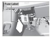
Fuse locations are shown on the label on the under panel.
