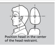
Head restraints are most effective for protection against whiplash and other rearimpact crash injuries when the center of the back of the occupant's head rests against the center of the restraint. The tops of the occupant's ears should be level with the center height of the restraint.
