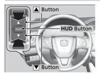
When the head-up display is on, press and hold the **HUD** button until its brightness level indicator on the driver information interface.
