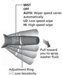
**AUTO** should always be turned **OFF** before the following situations in order to prevent severe damage to the wiper system:
