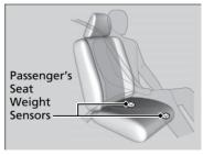
The front passenger's advanced airbag system has weight sensors.
