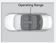
You can start the power system when the smart entry remote is inside the vehicle.
