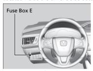
Replacement of fuses in the driver's side outer panel should be done by an authorized Honda Clarity Fuel Cell dealer.
