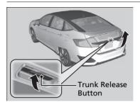
Push up the release button on the trunk lid after the doors are unlocked.
