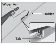
**4.** Press up on and hold the tab, then slide the holder off the wiper arm.
