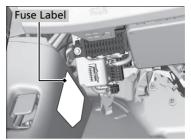
Fuse locations are shown on the label on the under panel.
