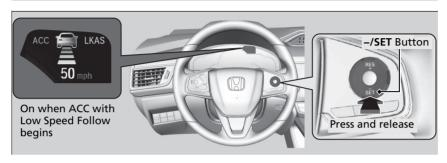
When driving at about 25 mph (40 km/h) or above: Take your foot off the pedal and press the –/SET button when you reach the desired speed. The moment you release the button, the set speed is fixed, and ACC with Low Speed Follow begins.
