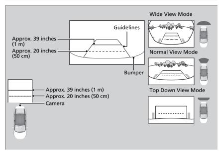
The rear camera view is restricted. You cannot see the corner ends of the bumper or what is underneath the bumper. Its unique lens also makes objects appear closer or farther than they actually are.
