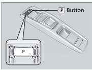
The gear position changes to  $\boxed{P}$  when you press the  $\boxed{P}$  button while the vehicle is parked with the power mode in ON. The indicators on the sides of the  $\boxed{P}$  button come on.
