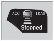
Your vehicle also stops, automatically. The **Stopped** message appears on the driver information interface and the head-up display.
