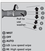
The windshield wipers and washers can be used when the power mode is in ON.
