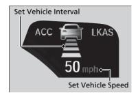
When ACC with Low Speed Follow starts operating, the vehicle icon, interval bars and set speed appear on the driver information interface.
