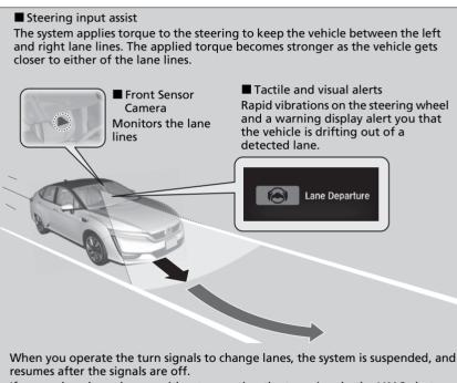
If you make a lane change without operating the turn signals, the LKAS alerts activate, and torque is applied to the steering.
