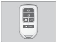
Use the keys to turn on and off the power system, and to lock and unlock the doors and to open the trunk. You can also use the remote transmitter to lock and unlock the doors and trunk
