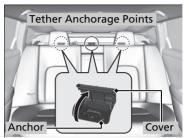
A tether anchorage point is provided behind each rear seating position.
