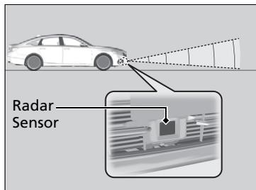
The radar sensor is at the lower part of the front bumper.
