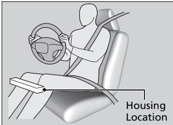
The driver's knee airbag is housed under the steering column.
