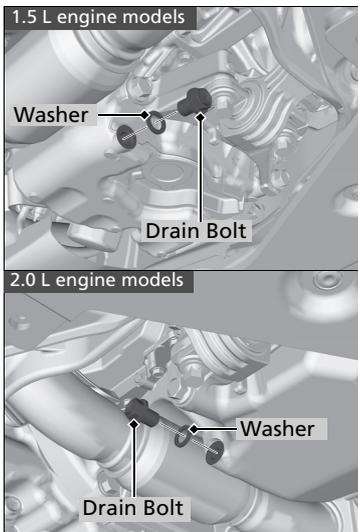
4. Remove the drain bolt and washer from the bottom of the engine, and drain the oil into a suitable container.
