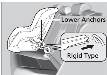
3. Place the child seat on the vehicle seat, then attach the child seat to the lower anchors according to the instructions that came with the child seat.
