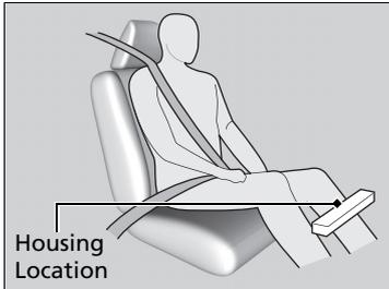
The front passenger's knee airbag is housed under the glove box.
