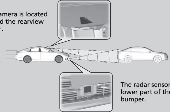
The radar sensor is at the lower part of the front bumper.
