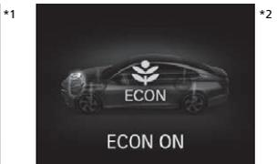
The message is displayed for a few seconds when the **ECON** button is pressed.
