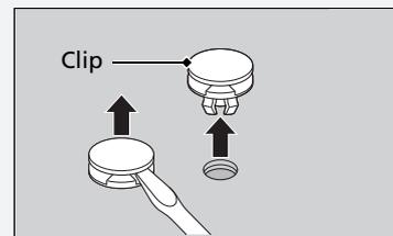
Insert the clip with the pin raised, and push until it is flat.
