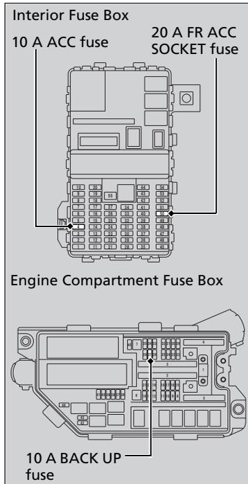
1. Remove the 20 A FR ACC SOCKET and 10 A ACC fuses. These fuses are located in the interior fuse box.
