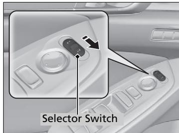
If activated, passenger's side door mirror automatically tilts downward when you put the transmission into **[R]**; this improves close-in visibility on the passenger's side of the vehicle when backing up. The mirror automatically returns to its original position when you take the transmission out of **[R]**.
