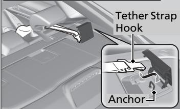
4. Open the tether anchor cover behind the head restraint.
