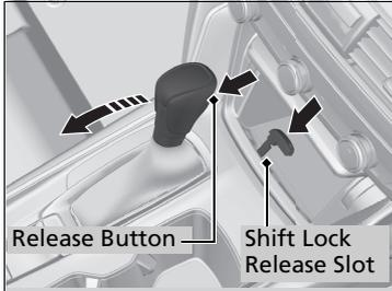
6. Insert the key into the shift lock release slot.
