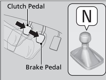
2. Check that the transmission is in neutral. Then depress the brake pedal with your right foot, and the clutch pedal with your left foot.
