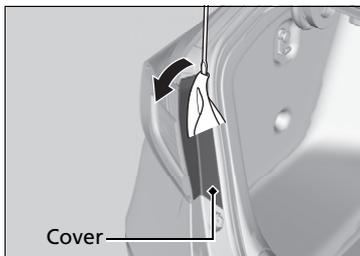
1. Pry on the edge of the cover using a flat-tip screwdriver to remove the covers.
