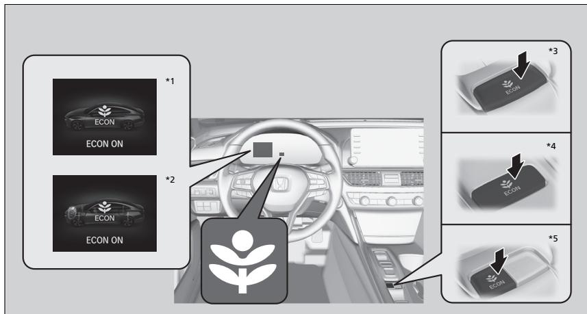
The **ECON** button turns the ECON mode on and off. The ECON mode helps you improve your fuel economy by adjusting the performance of the engine, transmission and climate control system.
