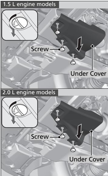
5. Remove the slotted head screws by turning 90° counterclockwise on the undercarriage and remove the under cover.
