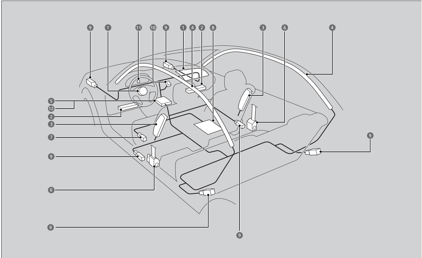
The front, front knee, front side, and side curtain airbags are deployed according to the direction and severity of impact. Both side curtain airbags are deployed in a rollover. The airbag system includes:
