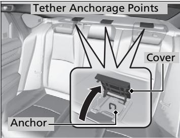
A tether anchorage point is provided behind each rear seating position. If you have a child seat that comes with a tether but can be installed with a seat belt, the tether may be used for additional security.
