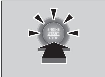
1. Touch the center of the **ENGINE START/STOP** button with the **H** logo on the remote while the **ENGINE START/STOP** button is flashing. The buttons on the remote should be facing you.
