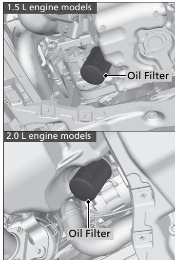
6. Remove the oil filter and dispose of the remaining oil.
