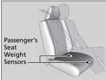
We advise against allowing a child age 12 or under to ride in the front passenger's seat. However, **if you do allow a child age 12 or under to ride in the front passenger's seat**, note that the system will automatically turn off the front passenger's airbag if the sensors detect that the child is approximately 65 lbs (29 kg) or less.
