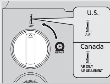
5. Turn the selector knob to **AIR<sup>\*1</sup>, AIR ONLY<sup>\*2</sup>, AIR SEULEMENT<sup>\*2</sup>**.
