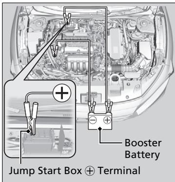
2. Connect the first jumper cable to your vehicle's jump start box  $\oplus$  terminal as shown. Do not connect this jumper cable to any other part.
