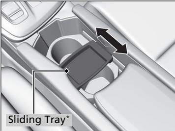
You can put small items in the sliding tray\* located in the console compartment lid. Slide the sliding tray\* forward or rearward.
