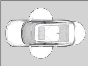
When you carry the remote, you can lock/unlock the doors and open the trunk. You can lock/unlock the doors within a radius of about 32 inches (80 cm) of the outside door handle. You can open the trunk within about 32 inches (80 cm) radius from the trunk release button.
