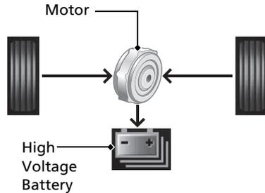
When the vehicle is decelerating or descending a hill, the electric motor acts as a generator that recovers a portion of the energy that was used to accelerate the vehicle.
