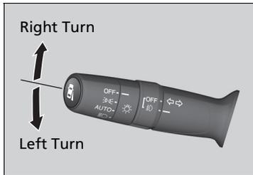
The turn signals can be used when the power mode is in ON.
