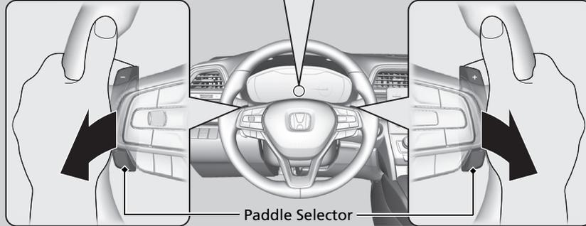
Increase the deceleration stage when pulling the **-** paddle selector (left side)
