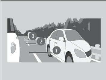
Three lines that appear on the screen can give an idea of how far the vehicles or objects on the screen are from your vehicle, respectively. If an object is near line 1 (in red), it indicates that it is close to your vehicle whereas an object near line 3 is farther away.
