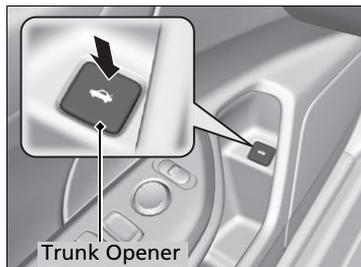
Pressing and holding the trunk opener on the driver's door unlocks and opens the trunk.
