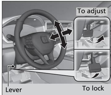
1. Pull the steering wheel adjustment lever up.
