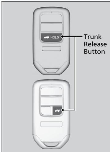
Press the trunk release button for approximately one second to unlock and open the trunk.
