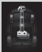
The engine is running and the motor is charging the High Voltage battery.
