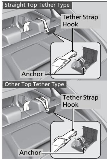
4. Open the tether anchor cover behind the head restraint.
