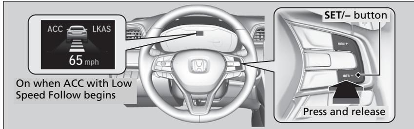
**When driving at about 25 mph (40 km/h) or above:** Take your foot off the pedal and press the **SET/-** button when you reach the desired speed. The moment you release the button, the set speed is fixed, and ACC with Low Speed Follow begins.
