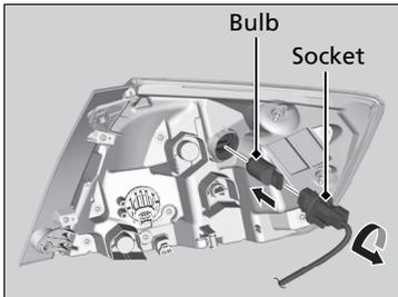
3. Turn the socket counterclockwise and remove it.
