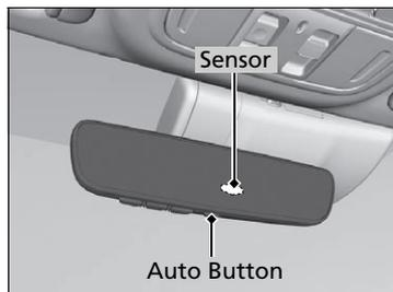
When you are driving after dark, the automatic dimming rearview mirror reduces the glare from headlights behind you, based on inputs from the mirror sensor. Press the auto button to turn this function on and off. When activated, the auto indicator comes on.
