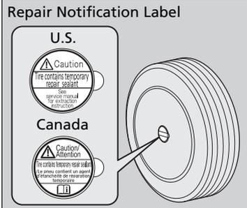
**12.** Apply the repair notification label to the flat surface of the wheel.
