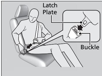
2. Insert the latch plate into the buckle, then tug on the belt to make sure the buckle is secure.
