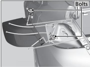
1. Use a Phillips-head screwdriver or socket to remove the bolts.
