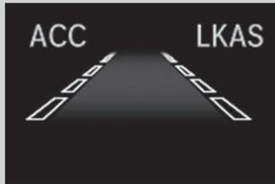
When the LKAS is suspended, the lane lines on the driver information interface change to contour lines, and the beeper sounds (if activated).
