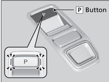
The shift position changes to **P** when you press the **P** button while the vehicle is parked with the power mode in ON. The indicators on the sides of the **P** button come on.
