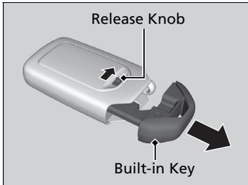
The built-in key can be used to lock/unlock the doors when the remote battery becomes weak and the power door lock/unlock operation is disabled.
