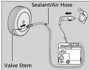
▶▶ Injecting Sealant and Air
