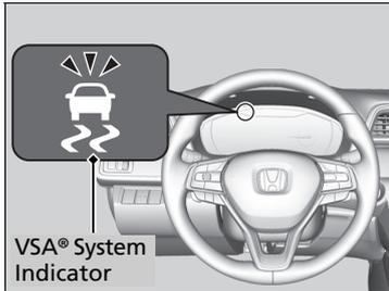
When VSA® activates, you may notice that the engine and motor does not respond to the accelerator. You may also notice some noise from the hydraulic system. You will also see the indicator blink.
