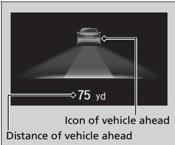
Shows the distance between your vehicle and the vehicle detected ahead.
