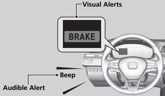
At system's earliest collision alert stage, you can change the distance (**Long/Normal/Short**) between vehicles at which alerts will come on through driver information interface or audio/information screen setting options.
