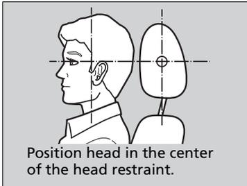
Head restraints are most effective for protection against whiplash and other rear-impact crash injuries when the center of the back of the occupant's head rests against the center of the restraint. The tops of the occupant's ears should be level with the center height of the restraint.
