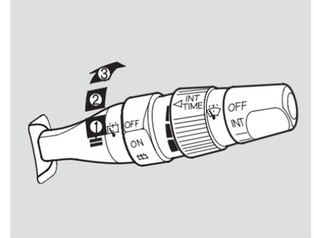
The rear window wiper switch is located next to the windshield wiper switch.
