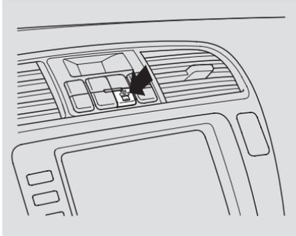
The rear window defogger will clear fog, frost, and thin ice from the window. Push the defogger button to turn it on and off. The indicator in the button lights to show the defogger is on. If you do not turn it off, the defogger will shut itself off after about 15 minutes. It also shuts off when you turn off the ignition. You have to turn it on again when you restart the vehicle.
