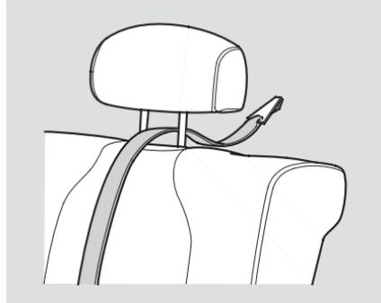
1. After properly securing the child seat (see page 47), lift the head restraint, then route the tether strap over the seat-back.
