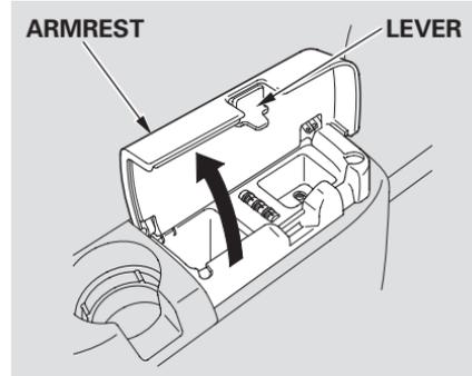
Auxiliary input jacks and wired headphone jacks for the rear entertainment system are under the third seat armrest on the passenger's side. To access these jacks, open the cover by pulling up on the lever.
