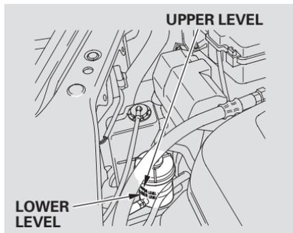
Check the level on the side of the reservoir when the engine is cold. The fluid should be between the UPPER LEVEL and LOWER LEVEL. If not add power steering fluid to the UPPER LEVEL mark.
