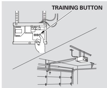
3. Press the training button on the garage door opener unit until the indicator next to the button comes on. The indicator may blink, or come on and stay on. You then have approximately 30 seconds to complete the following steps.
