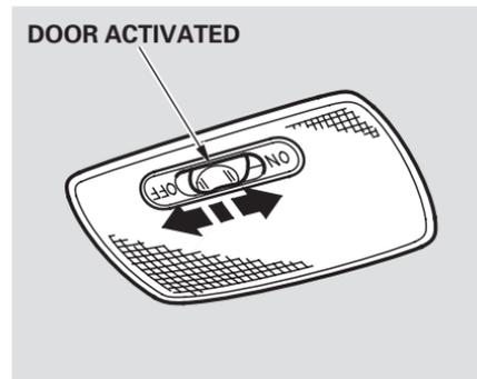
*The light control switch must be in either the ON or DOOR ACTIVATED position for the cargo area light to come on.*
