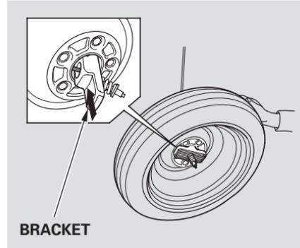
9. Keep turning the wheel nut wrench to create slack in the cable.
