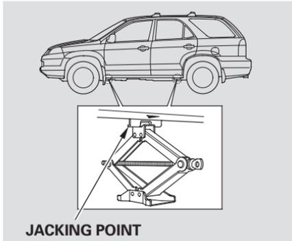
12. Place the jack under the jacking point nearest the tire you need to change. It is pointed to by a  $\triangle$  mark molded into the underside of the body. Turn the end bracket clockwise until the top of the jack contacts the jacking point. Make sure the jacking point tab is resting in the jack notch.
