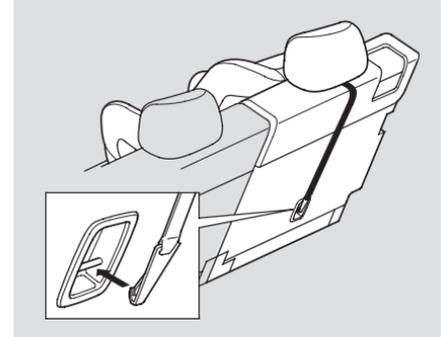
2. Attach the tether strap hook to the anchor, making sure the strap is not twisted.
