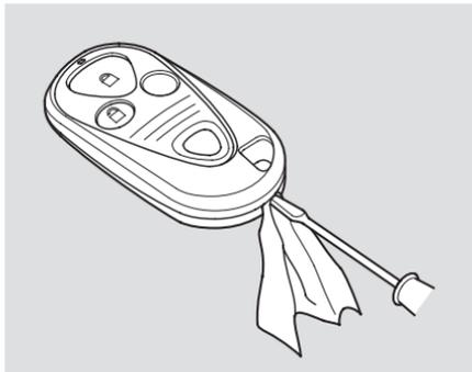
If it takes several pushes on the button to lock or unlock the doors and the tailgate, replace the battery as soon as possible.
