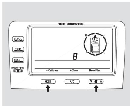
1. Press and hold the CLOCK and TRIP buttons until the display changes (about 1 second).
