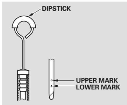
4. Remove the dipstick and check the fluid level. It should be between the upper and lower marks.
