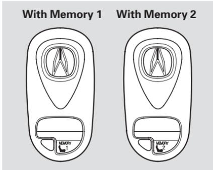
Each remote transmitter will also activate the Driving Position Memory System (see page 97 ). When you unlock and open the driver's door with the remote transmitter, you will hear a beep. The driver's seat, except power lumbar, and outside mirrors move to the positions stored in that memory location. You will hear two beeps
