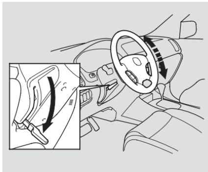
1. Push the lever under the steering column all the way down.
