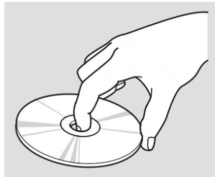
Handle a CD by its edges; never touch either surface. Do not place stabilizer rings or labels on the CD. These, along with contamination from fingerprints, liquids, and felt-tip pens, can cause the CD to not play properly, or possibly jam in the drive.
