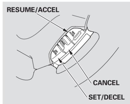
The cruise control may not hold the set speed when you are going up and down hills. If your speed increases going down a hill, use the brakes to slow down. This will cancel the cruise control. To resume the set speed, press the RESUME/ACCEL button. The indicator on the instrument panel will come back on.
