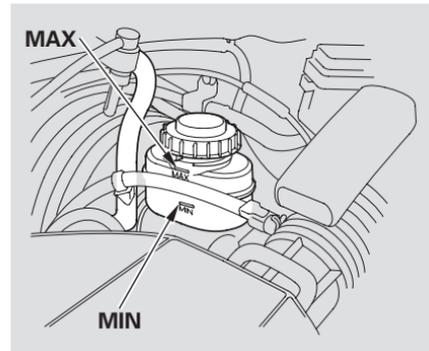
The fluid level should be between the MIN and MAX marks on the side of the reservoir. If the level is at or below the MIN mark, your brake system needs attention. Have the brake system inspected for leaks or worn brake pads.
