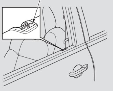
Once the security system is set, opening any door or the tailgate without using the key or the remote transmitter, or the hood, will cause it to alarm. It also alarms if the radio, navigation and DVD components are removed from the dashboard or the wiring is cut.
