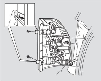
1. Open the tailgate. Use a screwdriver protected with a cloth to pry open the two covers.
