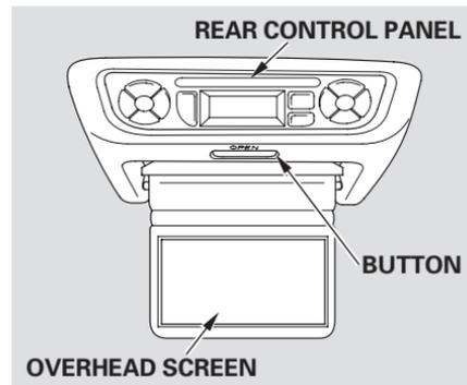
Open the overhead screen by pushing on the button. The screen will swing down part-way. Pivot the screen the rest of the way (to detent one or two). If you pivot the screen too far forward, past detent three, the display will turn off. Pivot the screen back to the detent to turn the display back on. To close the screen, pivot it up until it latches.
