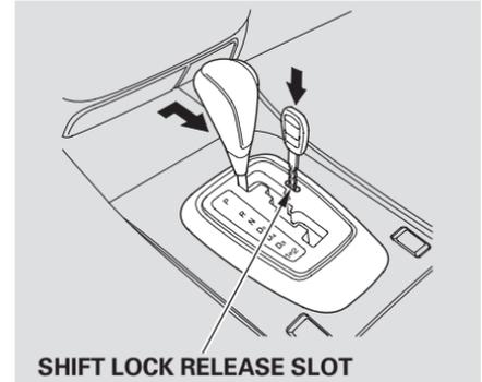
To release the reverse lockout, move the shift lever from Neutral to Reverse, then to Park.
