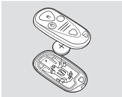
To replace the battery, place a cloth on the edge of the transmitter and remove the upper half by carefully prying on the edge with a small flat-tip screwdriver. Remove the old battery and insert a new battery with the + side facing up. Snap the two halves of the transmitter case back together.
