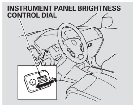
The dial on the instrument panel controls the brightness of the instrument panel lights, the blue lighting in the upper console and the front foot wells.
