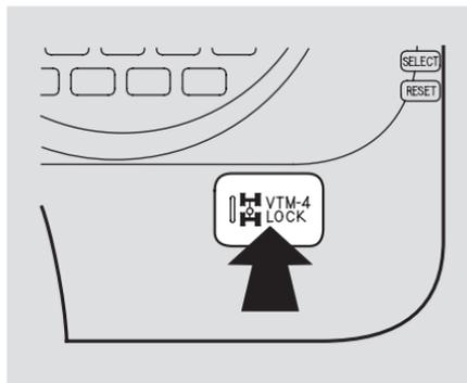
The Variable Torque Management 4WD System (VTM-4) automatically transfers varying amounts of engine torque to the rear wheels under lower traction conditions.
