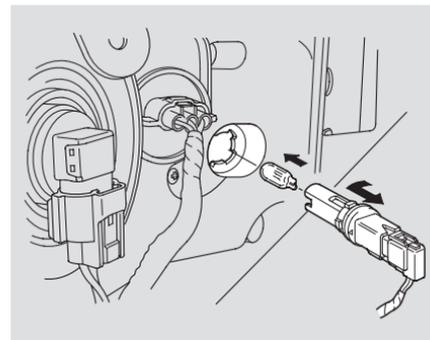
3. Install the new bulb into the socket.
