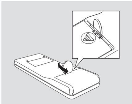
The remote control uses two AA batteries. To replace the batteries, put a coin in the notch on the back. Turn it one-quarter, then slide the cover off. Remove the old batteries. Make sure the polarity of the new batteries is correct when you install them. Slide the cover on until it locks.
