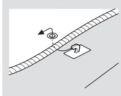
The driver's floor mat that came with your vehicle hooks over the floor mat anchor. This keeps the floor mat from sliding forward and possibly interfering with the pedals.
