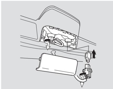
1. Remove the light assembly cover by prying carefully with a cloth-covered screwdriver in the notches along the top edge. Then pivot the cover out and down.
