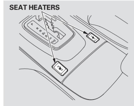
Both front seats are equipped with seat heaters. The passenger seat is only heated in the seat bottom because of the side airbag off system. The ignition switch must be in the ON (II) position to use them. Push the front of the switch, HI, to rapidly heat up the seat. After the seat reaches a comfortable temperature, select LO by pushing the back of the switch. This will keep the seat warm.
