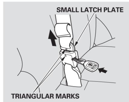
To unlatch the detachable anchor, insert a key into the slot on the side of the small buckle. Line up the triangle marks on the plate and buckle when reattaching the belt and buckle.
