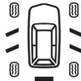
The appropriate indicator comes on in this display if the tailgate or any door is not closed tightly.
