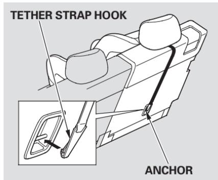
5. Lift the head restraint (see page 88 ), then route the tether strap through the legs of the head restraint, over the seat-back, making sure the strap is not twisted.
