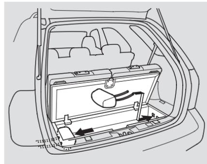
3. Use the ignition key to release the seat belt from the detachable anchor.
