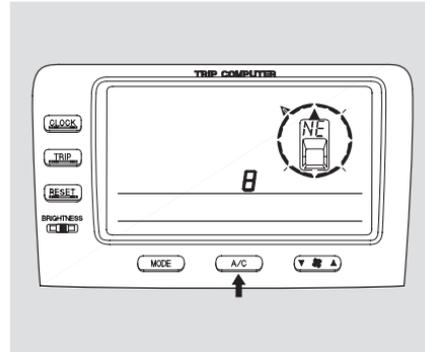
2. Press the Zone (A/C) button. The zone the compass is currently set to is displayed.
