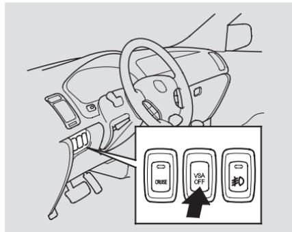
This switch is under the left vent. Press it to turn the VSA system on and off.
