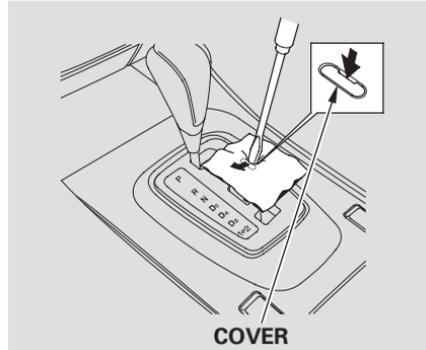
3. Put a cloth on the edge of the Shift Lock Release slot cover. Using a key, carefully pry on the edge of the cover to remove it.
