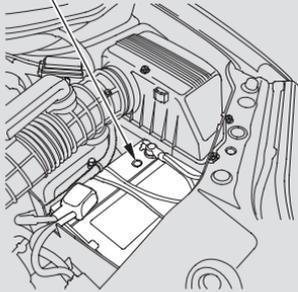
Check the condition of the battery monthly by looking at the test indicator window. The label on the battery explains the test indicator's colors.
