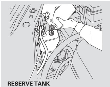
If the coolant level in the reserve tank is at or below the MIN line, add coolant to bring it up to between the MIN and MAX lines. Inspect the cooling system for leaks.
