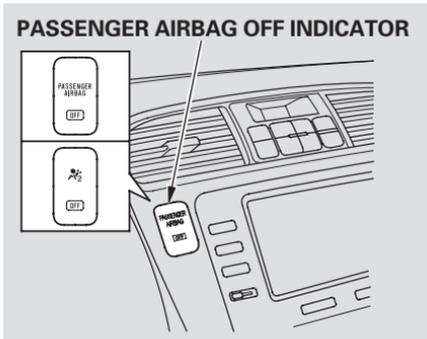
This indicator alerts you that the passenger's front airbag has been shut off because weight sensors detect the weight of an infant or small child on the front passenger's seat. It does **not mean** there is a problem with the airbag.
