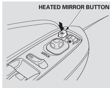
The outside mirrors are heated to remove fog and frost. With the ignition switch in the ON (II) position, turn on the heaters by pressing the button. The indicator in the button comes on as a reminder. Press the button again to turn the heaters off.
