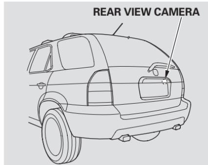
Whenever you shift to R (Reverse) with the ignition switch in the ON (II) position, the rear view is shown on the navigation system screen.
