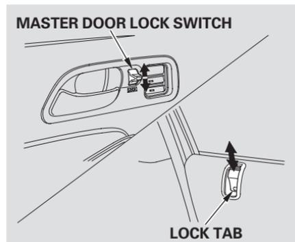
To lock all doors and the tailgate, press the master door lock switch on either front door, press the lock tab down on the driver's door, or use the key on the outside lock on the driver's door.
