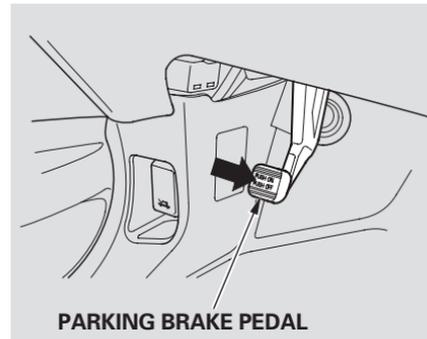
To apply the parking brake, push the pedal down with your foot. To release it, push on the pedal again. The parking brake indicator on the instrument panel should go out when the parking brake is fully released with the engine running (see page 61).
