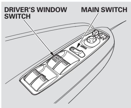
Turn the ignition switch to ON (II) to raise or lower any window. To open the window, push the switch down and hold it. Release the switch when you want the window to stop. Pull back on the switch and hold it to close the window.
