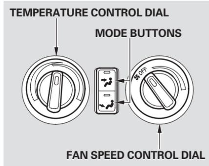
Press the RR A/C MANUAL button to enable the rear A/C control panel. The indicator in the button will come on. A passenger in the second row can then use the temperature control dial, fan speed dial, and mode buttons to adjust the temperature and airflow to their preference. This is limited by the system's minimum and maximum temperature.
