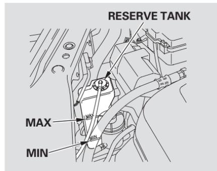
Look at the coolant level in the radiator reserve tank. Make sure it is between the MAX and MIN lines. If it is below the MIN line, see **Adding Engine Coolant** on page 240 for information on adding the proper coolant.
