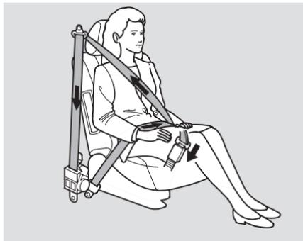
For added protection, the front seat belts are equipped with automatic seat belt tensioners. When activated, the tensioners immediately tighten the belts to help hold the driver and a front passenger in place. The tensioners are designed to activate in any collision severe enough to cause the front airbags to deploy, or if a sensor detects your vehicle is about to rollover (see page 31).
