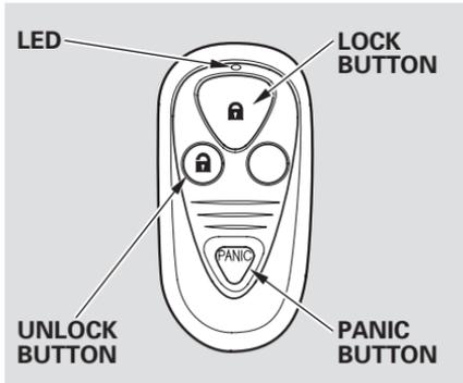
**LOCK** – Press this button once to lock all doors and the tailgate. Some exterior and interior lights will flash. When you push LOCK twice within 5 seconds, you will hear a beep to verify that the doors and tailgate are locked and the security system has set. This button does not work if any door or tailgate is not fully closed.
