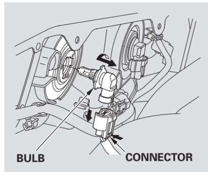
2. Remove the electrical connector from the bulb by squeezing the connector to unlock the tab, then slide the connector off the bulb.
