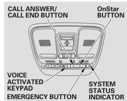
The OnStar buttons and indicator are located on the ceiling near the front map lights.
