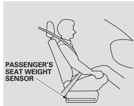
The passenger's advanced front airbag system has weight sensors under the seat. Although Acura does not encourage carrying an infant or small child in front, if the sensors detect the weight of an infant or small child, the system will automatically turn the passenger's front airbag off.
