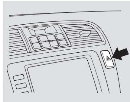
Push the red button to the right of the display to turn on the hazard warning lights (four-way flashers). This causes all four outside turn signals and both indicators in the instrument panel to flash. Use the hazard warning lights if you need to park in a dangerous area near heavy traffic, or if your vehicle is disabled.
