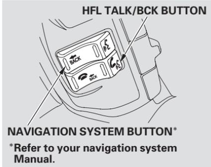
To operate the HFL, use the HFL TALK/BACK button on the left side of the steering wheel.
