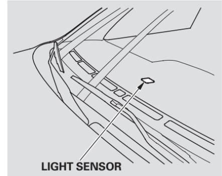
The automatic lighting feature is controlled by a sensor located on top of the dashboard. Do not cover this sensor or spill liquids on it.
