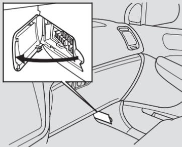
To open the passenger's side fuse box, pull the right edge of the cover.
