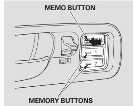
3. Press and release the MEMO button on the control panel. You will hear a beep. Immediately press and hold one of the memory buttons (1 or 2) until you hear two beeps. The indicator in the memory button will come on. The current positions of the driver's seat and outside mirrors are now stored.
