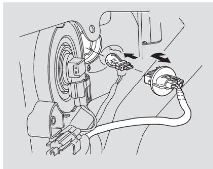
1. Remove the socket from the headlight assembly by turning it one-quarter turn counterclockwise.
