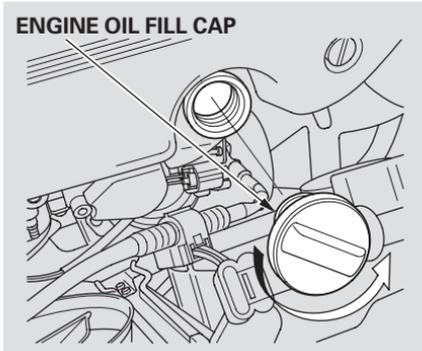
Unscrew and remove the engine oil fill cap on top of the valve cover. Pour in the oil slowly and carefully so you do not spill. Clean up any spills immediately. Spilled oil could damage components in the engine compartment. Install the engine oil fill cap, and tighten it securely. Wait a few minutes and recheck the oil level (see page 189). Do not fill above the upper mark; you could damage the engine.
