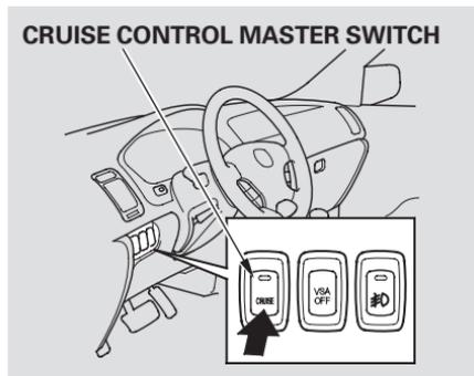
1. Push in the Cruise Control Master Switch. The indicator in the switch will come on.
