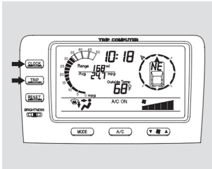
1. Press and hold the CLOCK and TRIP buttons until the display changes (about 1 second).
