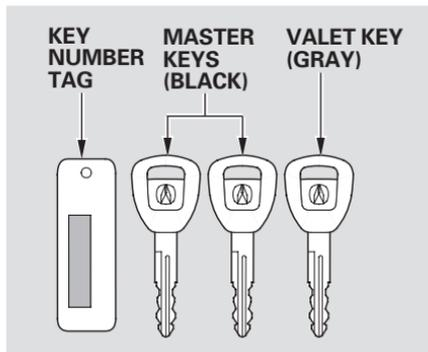
The master key fits all the locks on your vehicle. The valet key works only in the ignition and the door locks. You can keep the glove box locked when you leave your vehicle and the valet key at a parking facility.
