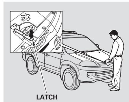
2. Put your fingers under the front edge of the hood near the center. Slide your hand to your left until you feel the hood latch handle. Push this handle up until it releases the hood. Lift the hood.
