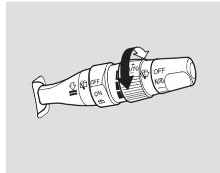
You can adjust the sensitivity of the system by turning the AUTO SENS ring next to the rotary switch.
