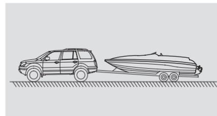
4. Remember, maximum gross combined weight should be decreased 2 % for every 1,000 feet (305 meters) of elevation.
