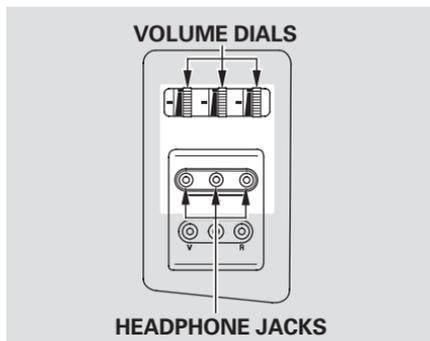
There are three wired headphone jacks for the third seat passengers. Each jack has its own volume control. These headphones are not supplied with the vehicle.
