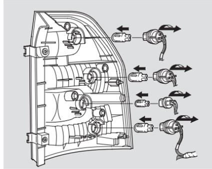
4. Remove the socket by turning it one-quarter turn counterclockwise.
