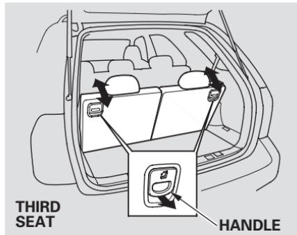
Pull on the handle on the back of the seat-back, move the seat-back to the desired position, and release the handle. Let the seat-back latch in the new position.
