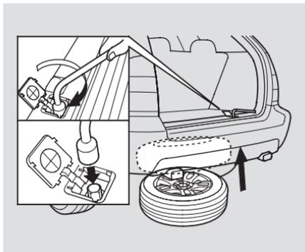
22. Slowly turn the wheel nut wrench clockwise to take up the slack of the hoist cable. Make sure the bracket is seated in the center hole of the spare tire.
