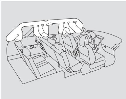
Your vehicle also has side curtain airbags to help protect the heads of the driver, front passenger, and passengers in the outer rear seating positions during a moderate to severe side impact or rollover (see page 31 for more information on how your side curtain airbags work).
