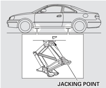
9. Locate the jacking point nearest the tire you need to change. It is pointed to by a  $\triangle$  mark molded into the underside of the body. Place the jack under the jacking point. Turn the end bracket clockwise until the top of the jack contacts the jacking point. Make sure the jacking point tab is resting in the jack notch.
