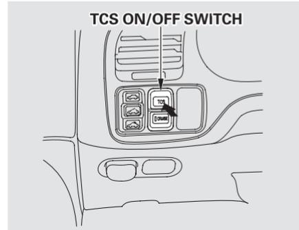
This switch is under the side vent. It lets you turn the Traction Control System on and off. You cannot turn off the TCS while the TCS indicator light is flashing.
