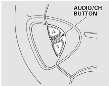
Two controls for the audio system are mounted in the steering wheel hub. These let you control basic functions without removing your hand from the wheel.
