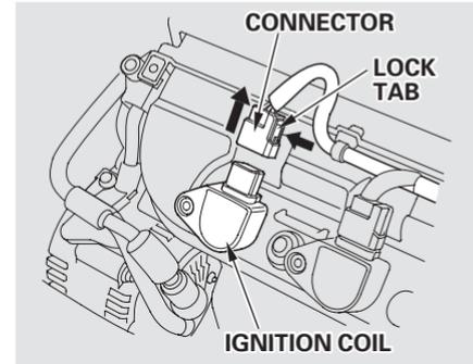
3. Disconnect the wire connector from the ignition coil by pushing on the lock tab and pulling on the connector. Pull on the plastic connector, not the wires.
