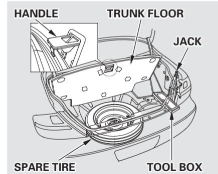
4. The tools are in the tool box on the right side of the trunk. Take the tools out of the tool box.
