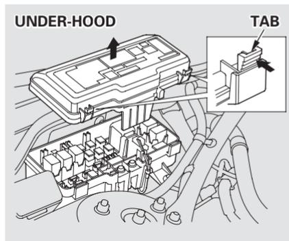
The under-hood fuse box is located in the back of the engine compartment on the passenger's side. To open it, push the tabs as shown.
