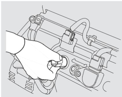
6. Put the new spark plug into the socket; then screw it into the hole. Screw it in by hand so you do not crosstread it.
