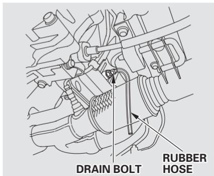
4. Install a rubber hose on the drain bolt at the rear of the engine cylinder block. Loosen the drain bolt. Drain the coolant into an appropriate container.
