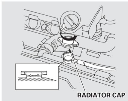
2. Turn the radiator cap counter-clockwise, without pressing down on it, until it stops. This relieves any pressure remaining in the cooling system.
