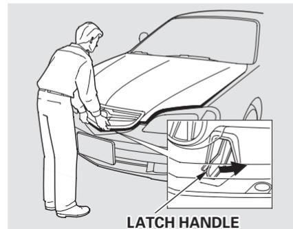
2. Standing in front of the car, reach in between the hood and the front bumper with your finger. The hood latch handle is under the "A" logo. Slide the latch handle to the right.
