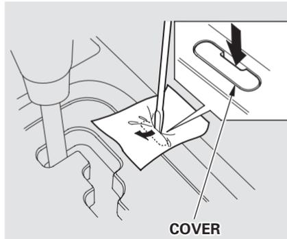
4. Insert a screwdriver in the Shift Lock Release slot.
