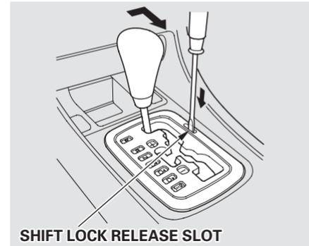
6. Remove the screwdriver from the Shift Lock Release slot, then reinstall the cover. Make sure the notch on the cover is on the right side. Depress the brake pedal and restart the engine.
