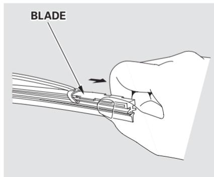
4. Remove the blade from its holder by grasping the tabbed end of the blade. Pull firmly until the tabs come out of the holder.
