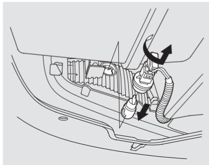
3. Pull the bulb straight out of its socket.
