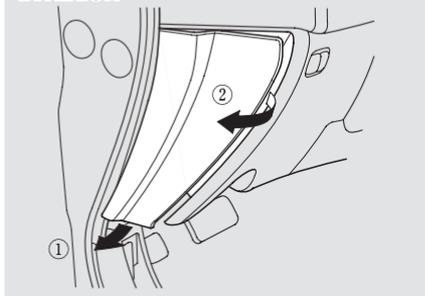
The interior fuse boxes are located on each side of the dashboard. To open an interior fuse box, open the car door. Pull the bottom of the cover open, then take it out of its side hinges by pulling it toward you.
