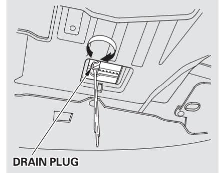
3. Loosen the drain plug on the bottom of the radiator. The coolant will drain through the splash guard. Drain the coolant into an appropriate container.
