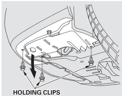
1. Use a flat-tipped screwdriver to remove the three holding clips from the splash shield. Pull the splash shield down.
