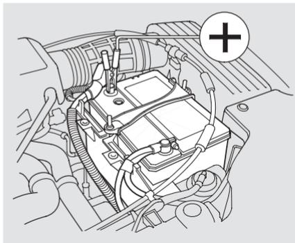
4. Connect one jumper cable to the positive (+) terminal on your Acura's battery. Connect the other end to the positive (+) terminal on the booster battery.
