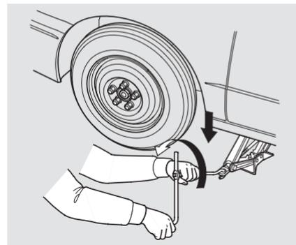
14. Lower the car to the ground and remove the jack.
