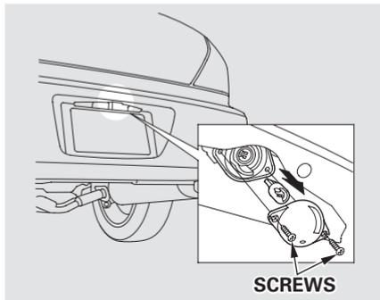
1. Use a small Phillips-head screwdriver to remove the two screws. Remove the lens from the license plate assembly.
