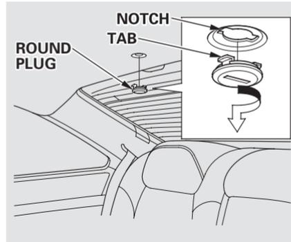
4. To remove the round plug in the center of the headliner, turn the plug by using a screwdriver or coin and pry it off. Make sure to align the tabs on the round plug to the notches on the ceiling as shown in the illustration.
