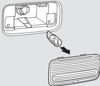
2. Remove the bulb by pulling it straight out of its metal tabs.
