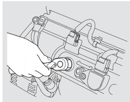
7. Torque the spark plug. (If you do not have a torque wrench, tighten the spark plug two-thirds of a turn after it contacts the cylinder head.)
