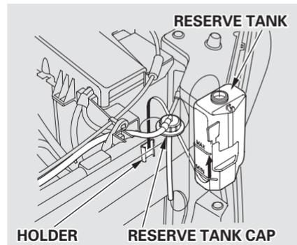
6. Remove the reserve tank from its holder by pulling it straight up. Drain the coolant into an appropriate container, then put the tank back in its holder.
