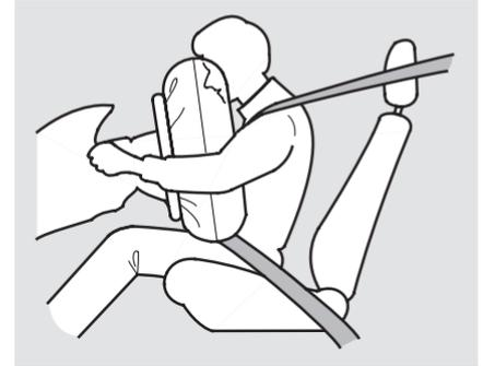
If you ever have a moderate to severe frontal collision, the sensors will detect the vehicle's rapid deceleration. If the rate of deceleration is high enough, the control unit will instantly inflate the front airbags.
