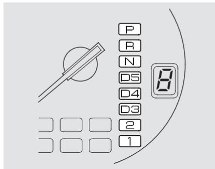
This indicator in the tachometer shows which position the shift lever is in. The illuminated number next to the "D5" indicator shows you the gear you have selected in the Sequential SportShift mode.
