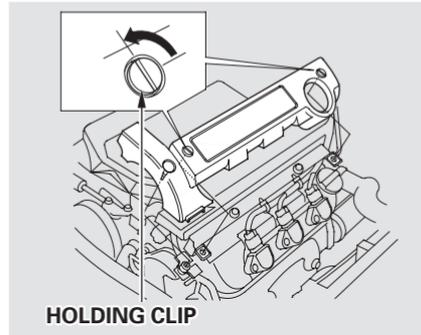
1. Loosen the two holding clips by turning the heads one-quarter turn counterclockwise with a flat-tipped screwdriver. Remove the cover on the front cylinder bank by pulling it straight up.
