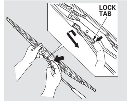
3. Disconnect the blade assembly from the wiper arm by pushing in the lock tab. Hold it in while you push the blade assembly toward the base of the arm.
