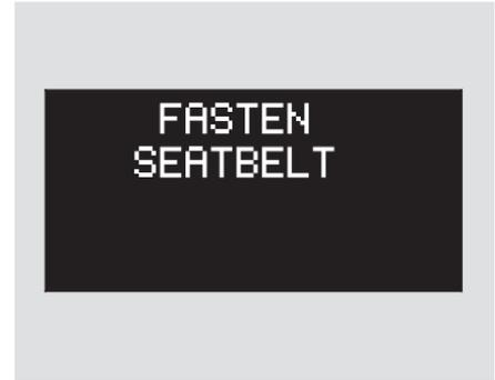
In addition to the seat belt reminder in the instrument panel, the multi-information display interrupts the current display and shows "FASTEN SEAT BELT" for about 6 seconds if you do not fasten your seat belt while driving. This message repeats if you ignore it and do not wear your seat belt while the vehicle is moving.
