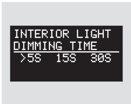
The interior lights fade out when you close all doors (see page [113](#)). Select how long it takes for the interior lights to fade out (in seconds) from 5S, 15S, or 30S, and enter your selection by moving the pointer with the > side of the INFO button.
