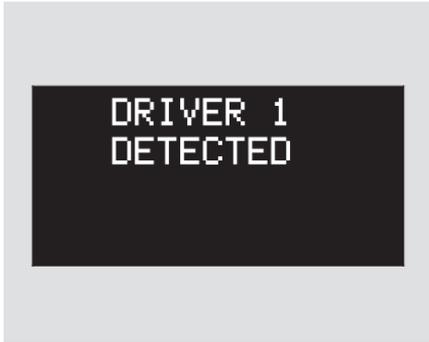
When you unlock and open the driver's door with the key, the display shows "DRIVER 1 DETECTED" or "DRIVER 2 DETECTED", depending on which remote transmitter was used last. (The driver's "ID" is determined by the transmitter.)
