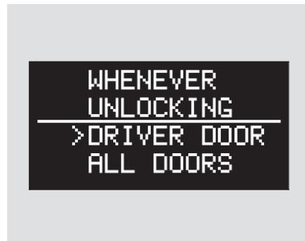
4. To designate the door(s) that unlock under the previous step, select "DRIVER'S DOOR" or "ALL DOORS" by moving the pointer with the INFO button. Then enter your selection by moving the pointer with the > side of the INFO button.
