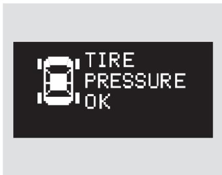
When you press the
