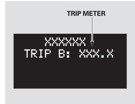
This meter shows the number of miles (U.S.) or kilometers (Canada) driven since you last reset it. There are two trip meters: Trip A and Trip B. When you first turn the ignition switch to ON (II), Trip A is displayed. Switch between Trip A and Trip B by pressing the Select/Reset button repeatedly. Each trip meter works independently, so you can keep track of two different distances.
