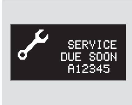
When the engine oil life reaches 15 percent, the display shows "SERVICE DUE SOON" and the code for the maintenance items to be performed.
