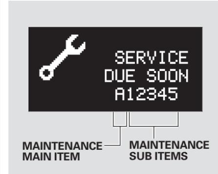
When the remaining engine oil life is 15%, you will see the message “SERVICE DUE SOON” along with all maintenance items that are needed at oil change time. Refer to page 213 for a complete list of the maintenance main items and sub items.
