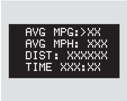
When the multi-information display is in the trip computer mode, press the Select/Reset button. The display changes as shown above.
