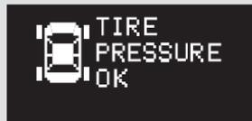
Your vehicle is equipped with a tire pressure monitoring system (TPMS) that turns on every time you start the engine and monitors the pressure in your tires while driving.
