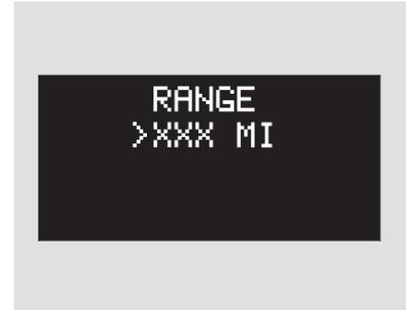
When the display shows the initial trip computer screen, press the > side of the INFO button to display "RANGE". This is the estimated distance you can travel on the fuel remaining in the tank. This distance is estimated from the fuel economy you received over the last several miles, so it will vary with changes in speed, traffic, etc.
