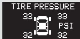
To see the inflation pressures of all four tires, press the SEL/RESET button. The display changes as shown above.
