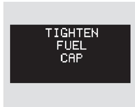
If the fuel fill cap is missing or not tightened properly, you will see "TIGHTEN FUEL CAP". Make sure the fuel cap is installed and tightened properly at least once.
