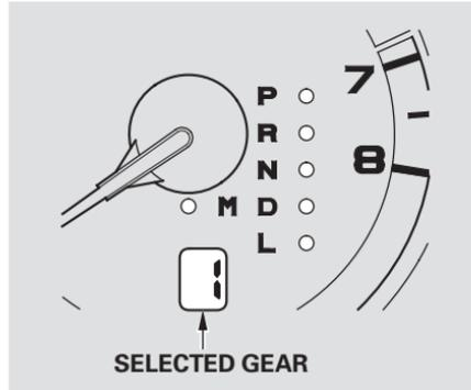
passenger’s side. When you move the shift lever from “D” to the Sequential SportShift mode, the display shows the selected gear.
