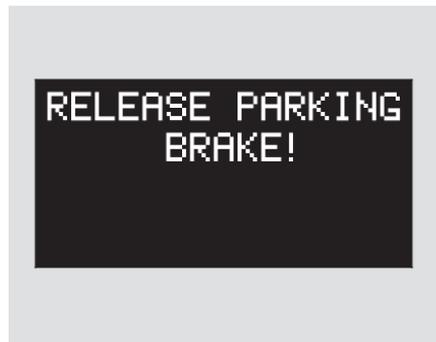
If you start driving without releasing the parking brake, the multi-information display interrupts the current display and shows "RELEASE PARKING BRAKE."
