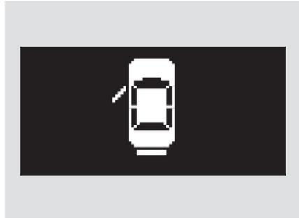
If the trunk or any door is not closed tightly, the display reminds you to close the open trunk or the door(s) before you start driving.
