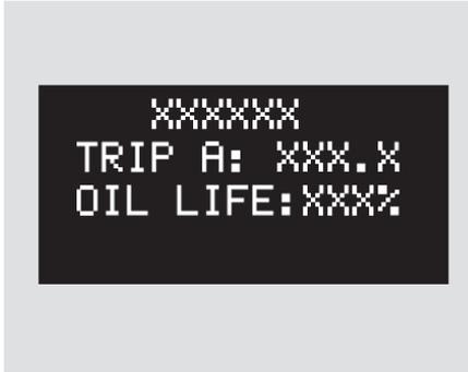
This shows the remaining life of the engine oil. It shows 100% after the engine oil is replaced and the display is reset. The engine oil life is calculated based on engine operating conditions and accumulated engine revolutions.
