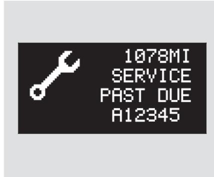
If the indicated maintenance service is not done and the remaining engine oil life gets less than 0%, you will see the message “SERVICE PAST DUE” on the display. Immediately have the service performed, and make sure to reset the display as previously described.
