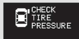
Each tire has its own pressure sensor. If the air pressure of a tire becomes significantly low, the sensor in that tire immediately sends a signal that causes the low tire pressure indicator in the instrument panel to come on. If this happens, you will see which tire is losing the pressure in the multi-information display along with a "CHECK TIRE PRESSURE" message.
