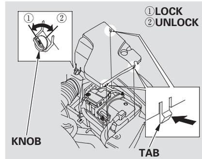
1. Turn the knob of the battery cover to UNLOCK as shown in the illustration.
