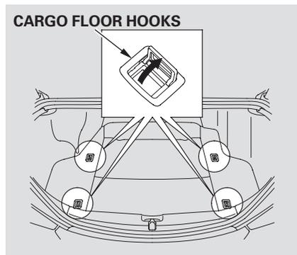
The cargo floor hooks can also be used to tie down and secure items on the floor.
