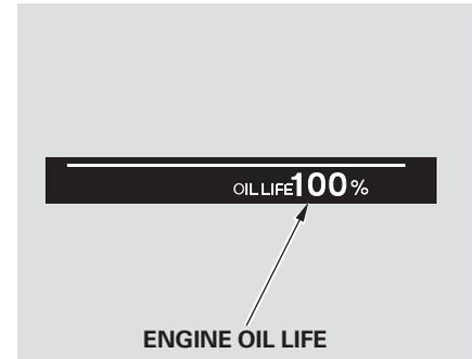
This shows the remaining life of the engine oil. It shows 100% after the engine oil is replaced and the display is reset. The engine oil life is calculated based on engine operating conditions and accumulated engine revolutions. For more information, see page 291.
