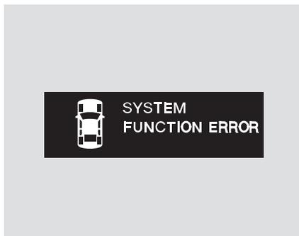
If there is a system error with the TPMS, the multi-information display shows a “SYSTEM FUNCTION ERROR” message (see page 72 ), and the tire pressure readings will not be displayed. You will also see a “CHECK TPMS SYSTEM” message on the multi-information display (see page 280 ).
