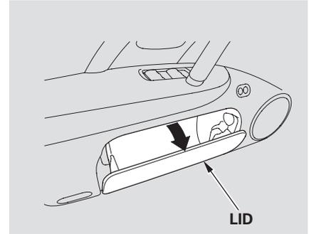
The interior of each front door has an extendable pocket for maps and other small, lightweight items. For safety, be sure both front door pockets are closed while driving.
