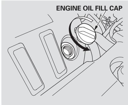
Unscrew and remove the engine oil fill cap on top of the left valve cover. Pour in the oil slowly and carefully so you do not spill. Clean up any spills immediately. Spilled oil could damage components in the engine compartment.
