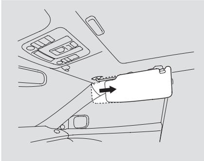
To use a sun visor, pull it down. You can also use a sun visor at the side window. Remove the support rod from the clip, and swing the sun visor toward the side window. You can extend the sun visor further by pulling it back.
