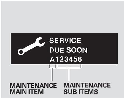
When the remaining engine oil life is 15 to 6 percent, the multi-information display shows a “SERVICE DUE SOON” message along with the maintenance schedule code indicating the main and sub items required at the time of the oil change. Refer to page [299](#) and [300](#) for a complete list of the maintenance main items and sub items.
