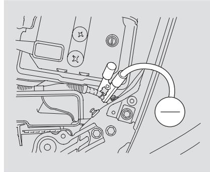
5. Connect the second jumper cable to the negative (-) terminal on the booster battery. Connect the other end to the grounding point as shown. Do not connect this jumper cable to any other part of the engine.
