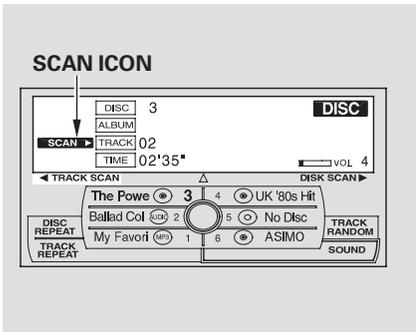
When you press the SCAN button or scroll down and push the interface selector to the left, the first track of the current disc plays for about 10 seconds. You will see SCAN next to TRACK on the screen. To hear the rest of the track, press the SCAN button or push the interface selector
