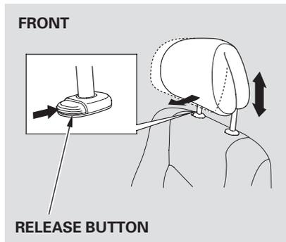
The head restraints adjust for height. The tilt of the front head restraints is also adjustable. You need both hands to adjust the restraint. Do not attempt to adjust it while driving. To raise it, pull upward. To lower the restraint, push the release button sideways, and push the restraint down. To adjust the tilt, pivot the front head restraint to the desired position.
