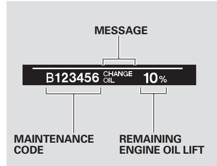
Press the SEL/RESET button on the steering wheel repeatedly to select the engine oil life minder, the message “CHANGE OIL” along with the percentage of oil life remaining, and the maintenance item code, are displayed on the lower part of the multi-information display.
