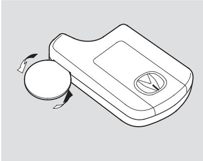
Replace the batteries if necessary.
