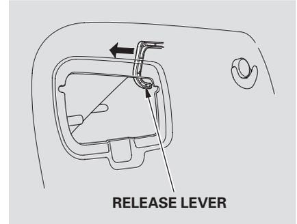
To open the fuel fill door, pull the release lever rearward.
