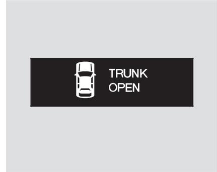
When the trunk is not tightly closed, the “TRUNK OPEN” indicator will stay on.
