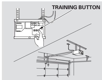
3. Press the training button on the garage door opener unit until the indicator next to the button comes on, then release it. The indicator may blink, or come on and stay on.
