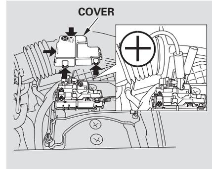
3. Remove the battery cover (see page 332), then remove the secondary under-hood fuse box cover from the positive (+) terminal on the battery.
