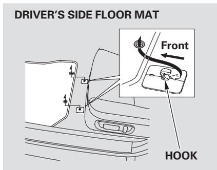
The floor mats that came with your vehicle hook over floor mat anchors. This keeps the floor mats from sliding forward/rearward and possibly interfering with the pedals or making the front passenger's weight sensor's ineffective. If you remove a floor mat, make sure to re-anchor it when you put it back in your vehicle.
