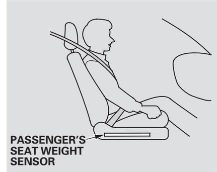
The passenger's advanced front airbag system has weight sensors under the seat. If the sensors detect an infant or small child may be in the seat, the system will automatically turn the passenger's front airbag off.
