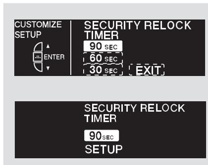
If you unlock the doors by pressing the button on the remote or grabbing the driver's door handle while carrying the remote, but do not open any of the doors within 30 seconds, the doors automatically relock and the security system sets. You can select this relock time to be 90, 60, or 30 seconds.
