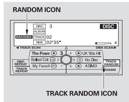
To play the tracks of the current disc in random order, use the interface selector to scroll down, select TRACK RANDOM, and press ENTER on the interface selector. As a reminder, you will see RANDOM next to TRACK on the screen. To turn this feature off, highlight TRACK RANDOM (if not already highlighted), and press ENTER on the interface selector again.
