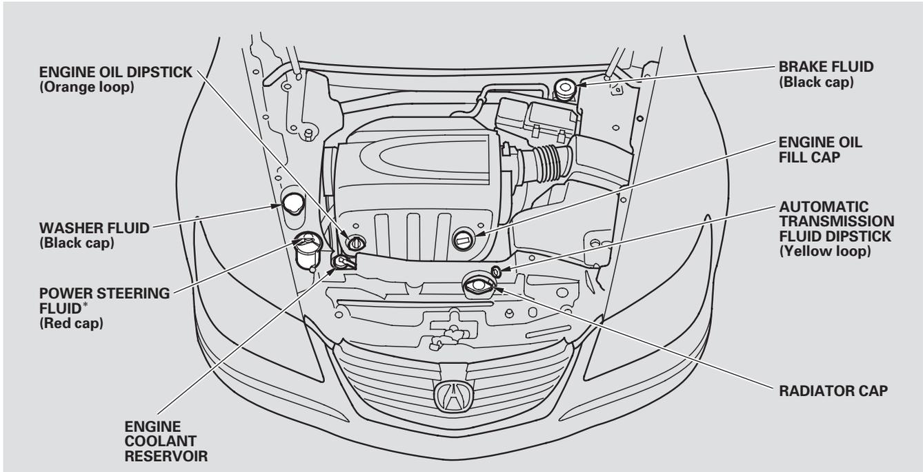
\*: The power steering fluid reservoir is located under the right compartment cover.
