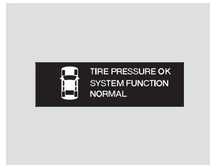
When all tire pressures are normal, the multi-information display will show “TIRE PRESSURE OK SYSTEM FUNCTION NORMAL.”
