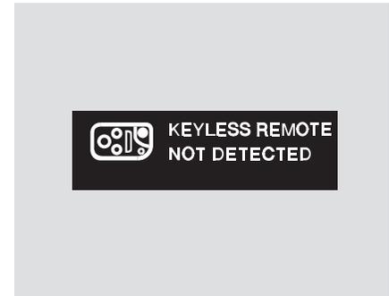
When you are pressing the ignition switch, or when the ignition switch is in the ON (II) position, the beeper sounds if you take the remote out of the vehicle and close the door.
