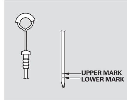
3. Insert the dipstick all the way into the transmission as shown.
