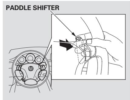
While in the Sequential SportShift Mode, you can also shift up or down using the + (right side) or – (left side) paddle shifters on the right and left side of the steering wheel.
