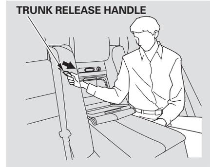
If your vehicle's battery goes dead or is disconnected, you can open the trunk from the rear seat by pulling the trunk release handle. Reach the handle through the trunk pass-through.
