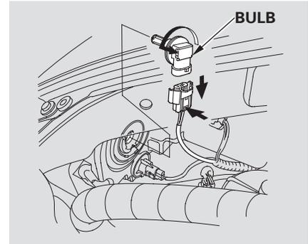
2. Remove the electrical connector from the bulb by pushing on the tab and pulling the connector down.
