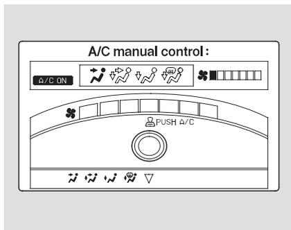
Press the A/C
