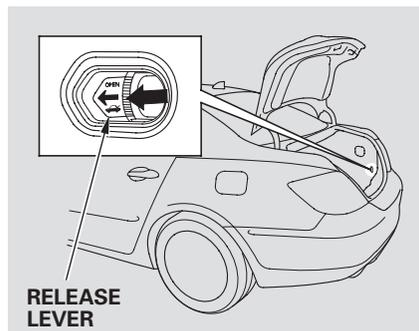
As a safety feature, your vehicle has a release lever on the right corner in the trunk so the trunk can be opened from the inside. To open the trunk, push the release lever to the left.
