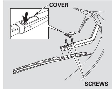
2. Push the edge of the cover on the blade assembly until the other side of edge is pivoted out, and remove the cover.
