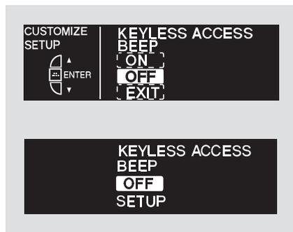
If you unlock the doors by grabbing the driver's door handle while carrying the remote, the beeper sounds twice. When you lock the doors, the beeper sounds once. You can turn this feature on or off.
