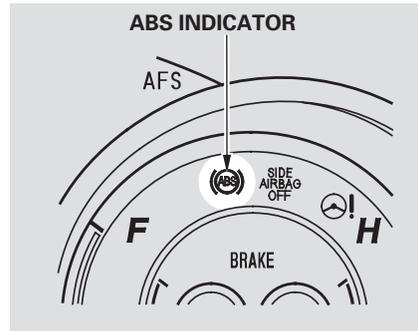
If the ABS indicator comes on, the anti-lock function of the braking system has shut down. The brakes still work like a conventional system, but without anti-lock. You should have your dealer inspect your vehicle as soon as possible.
