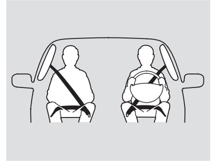
Your vehicle also has side curtain airbags to help protect the heads of the driver, front passenger, and passengers in the outer rear seating positions during a moderate to severe side impact. For more information, see page [32](#).
