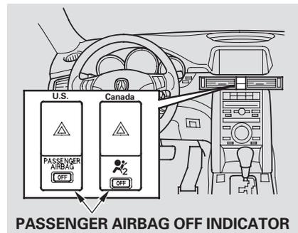
This indicator alerts you that the passenger’s front airbag has been shut off because weight sensors detect an infant or small child may be in the front passenger’s seat. It does **not mean** there is a problem with the airbag.
