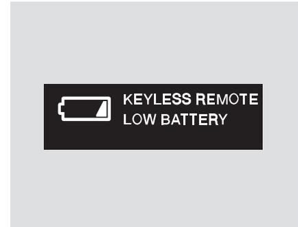
The batteries in the remote normally lasts about 2 years. To ensure maximum battery life, do not store the remote close to electrical devices such as computers or TVs. When the multi-information display shows “KEYLESS REMOTE LOW BATTERY,” replace the batteries as soon as possible (see page [135](#) ).
