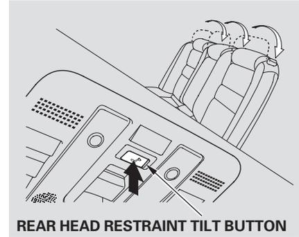
3. Push the rear head restraint tilt button on the ceiling console to pivot the head restraints down.
