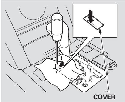
3. Put a cloth on the edge of the shift lock release slot cover next to the shift lever. Use a small flat-tipped screwdriver or a metal fingernail file to remove the cover. Carefully pry on the edge of the cover.
