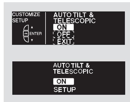
When you turn the ignition switch to LOCK (0) and release it, or remove the built-in key from the ignition switch, the steering wheel automatically moves fully in and up. You can turn this feature on or off.
