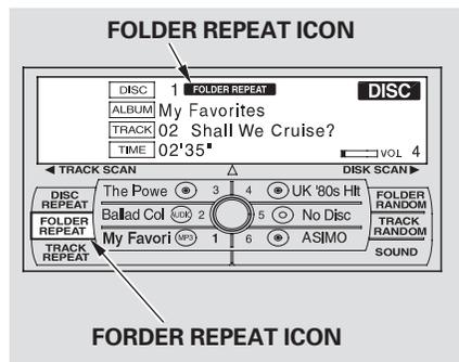
To replay the current folder continuously, use the interface selector to scroll down, select FOLDER REPEAT with the interface knob, and press ENTER on the interface selector. As a reminder, you will see FOLDER REPEAT next to the disc number on the screen. To turn this feature off, highlight FOLDER REPEAT (if not already highlighted), and press ENTER on the selector again.
