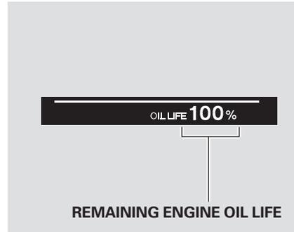
To see the remaining engine oil life displayed on the lower right corner on the multi-information display as a percentage, turn the ignition switch to ON (II), and press the SEL/RESET button on the steering wheel repeatedly until the engine oil minder appears (see page 71 ).
