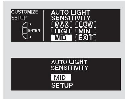
The headlights automatically come on when the headlight switch is in the AUTO position and ambient light reaches a customizable level. You can select the auto light sensitivity.
