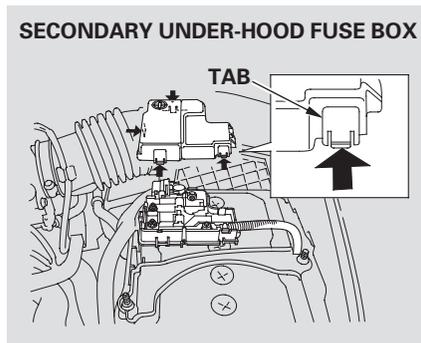
The secondary under-hood fuse box is on the battery. To open it, push the tabs as shown.
