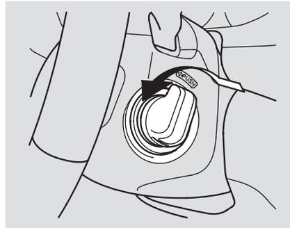
To turn the ignition switch to the LOCK (0) position, put the transmission in Park, press the switch in, and turn it to LOCK (0). When the transmission is not in Park, you cannot turn the ignition switch to the LOCK (0) position.
