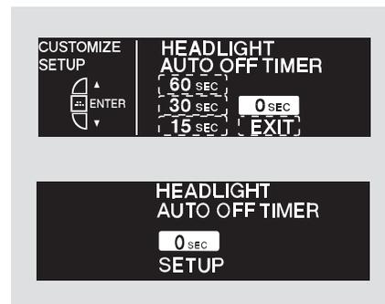
The headlights, parking lights, side marker lights, taillights, and license plate light turn off after the selected time when you close the driver's door and take the remote with you.
