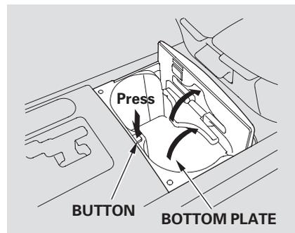
For a long container, press the button in the beverage holder to raise the bottom plate. Stand the separator up.
