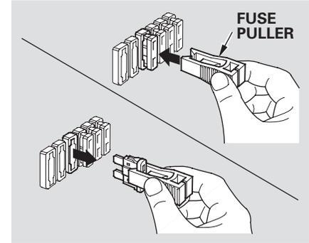
4. Check the smaller fuses in the under-hood fuse box and all the fuses in the interior fuse boxes by pulling out each fuse with the fuse puller. The fuse puller is inside the primary under-hood fuse box.
