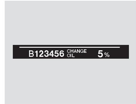
Press the SEL/RESET button on the steering wheel repeatedly to select the engine oil life minder, the message “CHANGE OIL” along with the percentage “5%,” and the maintenance item code are displayed on the lower part of the multi-information display when the calculated engine oil life is 1–5 percent (see page [291](#) ).
