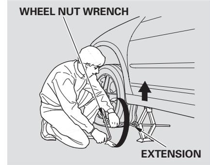
8. Use the extension and the wheel nut wrench as shown to raise the vehicle until the flat tire is off the ground.
