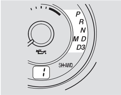
These indicators on the instrument panel show which position the shift lever is in. In the Sequential SportShift Mode, the “M” indicator next to the “D” indicator comes on, and the illuminated number under the low oil pressure indicator shows you the gear you have selected.
