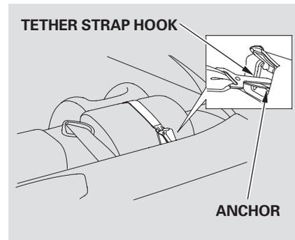
7. Attach the tether strap hook to the tether anchor, then tighten the strap as instructed by the child seat maker.
