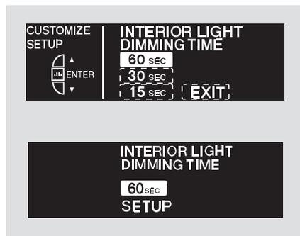
The interior lights fade out when you close all doors (see page 160 ). Select how long it takes for the interior lights to fade out (in seconds) from 60 SEC, 30 SEC, or 15 SEC by pressing the ▲ or ▼ button, and enter your selection by pressing the SEL/RESET button.
