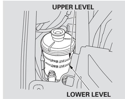
After removing the right engine compartment cover (see page 304 ), check the level on the side of the reservoir when the engine is cold. The fluid should be between the UPPER LEVEL and LOWER LEVEL. If not, add power steering fluid to the UPPER LEVEL mark.
