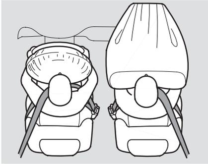
Your vehicle has a supplemental restraint system (SRS) with front airbags to help protect the heads and chests of the driver and a front seat passenger during a moderate to severe frontal collision. For more information, see page [27](#).
