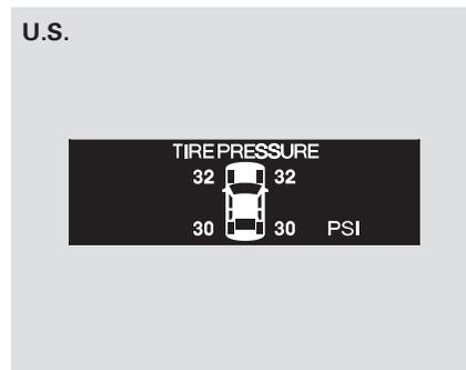
When the TPMS is functioning normally, you can press the SEL/RESET button on the steering wheel to see the pressure readings of each tire in psi (U.S. models) or kPa (Canadian models) (see page 74 ).
