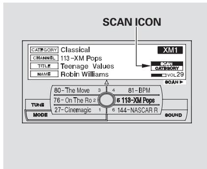
**SCAN** – The scan function gives you a sampling of all channels while in the channel mode. In the category mode, only the channels within that category are scanned. To activate SCAN, press the SCAN button. To scan with the interface dial, scroll down, and push interface selector to the right. You will see SCAN on the screen.
