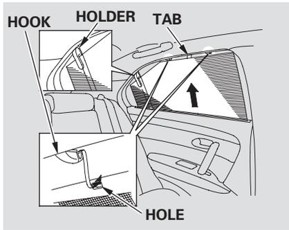
Each rear door has an integrated sunshade. To use a sunshade, hold the tab on the top, insert the sunshade into the holder, and pull the sunshade all the way up. Insert the holes on the sunshade into the hooks on the window frame.
