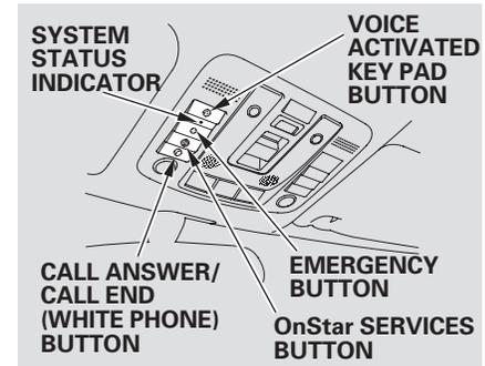
The OnStar buttons and indicator are located on the ceiling near the front ceiling light.
