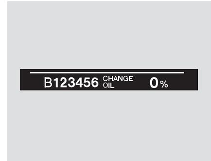
Press the SEL/RESET button on the steering wheel repeatedly to select the engine oil life minder, the message “CHANGE OIL” along with the percentage “0%,” and the maintenance item code are displayed on the lower part of the multi-information display when the calculated engine oil life is 0–1 percent.
