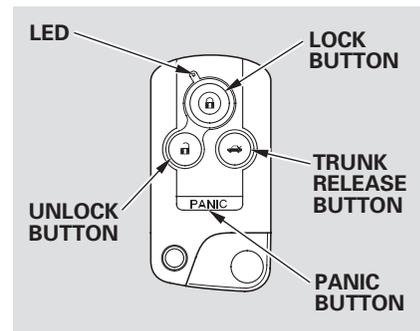
**LOCK** – Press this button once to lock all doors. Some exterior lights will flash. When you push LOCK twice within 5 seconds, you will hear a beep to verify that the doors are locked and the security system is ready.
