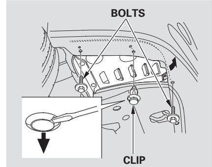
1. Use a Phillips-head screwdriver to remove the two mounting bolts and remove the holding clip with a flat-tipped screwdriver.
