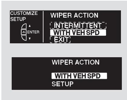
You can select from two settings when the wiper switch is in the INT position.
