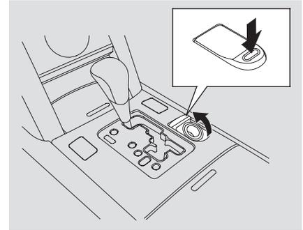
There are two accessory power sockets. One is located in the front of the center console. To use the power socket, push and release the lid, then push it forward until the socket comes to the proper position to use.
