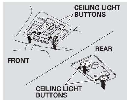
Push each ceiling light button to turn its light on and off.
