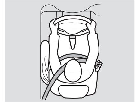
If you ever have a moderate to severe side impact, the sensors will detect rapid deceleration and signal the control unit to instantly inflate either the driver’s or the passenger’s side airbag.
