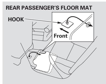
Make sure the rear floor mats are properly hooked to the floor mat anchors. Your vehicle is equipped with front passenger's seat weight sensors. If the rear passenger's floor mat is on the seat rail of the front passenger's seat, the sensors will detect the decreased weight on the seat and they may not work properly.
