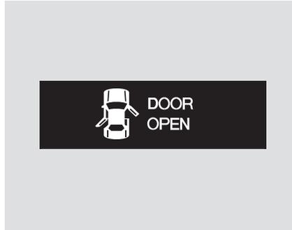
When one or more doors are not tightly closed, the “DOOR OPEN” indicator will stay on.
