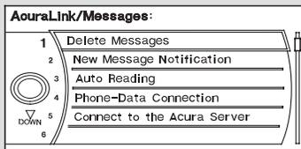
To access the following functions, press the SETUP button, push the interface dial to the right to select MORE, then rotate the interface dial to select AcuraLink/Messages.
