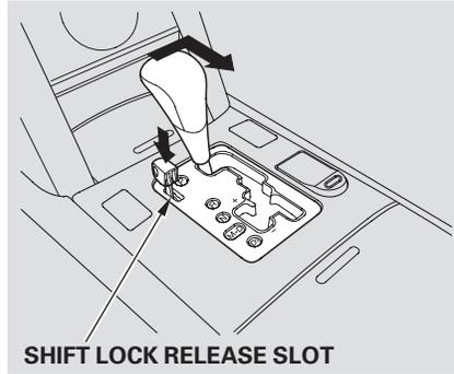
4. Insert a built-in key into the shift lock release slot.
