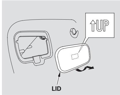
If the fuel fill door release button does not work, use the release lever inside the left maintenance lid in the trunk.
