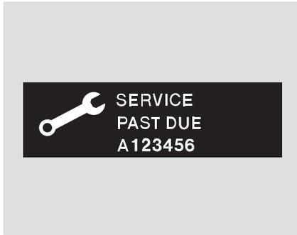
If the indicated maintenance service is not done and the remaining engine oil life reaches 0 percent, the multi-information display will show the message “SERVICE PAST DUE” and the maintenance item code. This message is displayed when the total mileage after reaching 0 percent engine oil life is less than 10 miles (for U.S. models)/10 km (for Canadian models).
