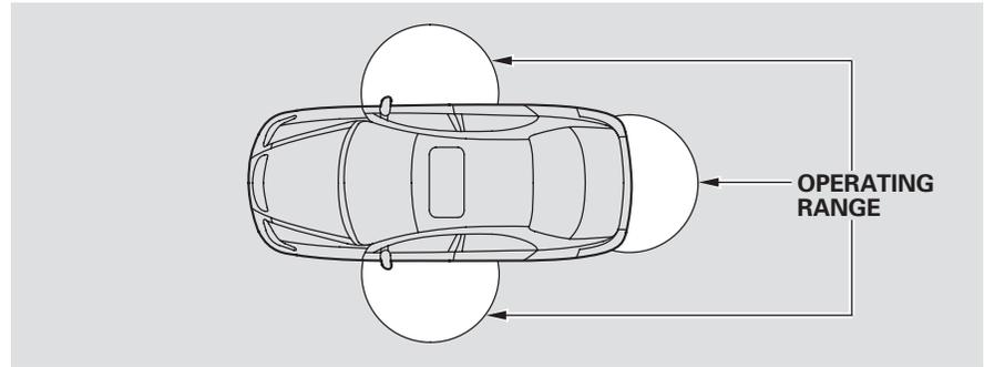
the doors and unlock the trunk. When you carry the remote, you can lock/unlock the doors, unlock the trunk, and start the engine without a key.
