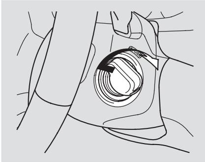
When you push the ignition switch, the remote and the vehicle recognize each other. After the recognition, the remote indicator flashes, and a beeper sounds once. After the beep, turn the ignition switch.
