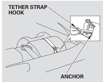
1. After properly securing the child seat with the lap/shoulder belt (see page 47 ), pivot the head restraint down (see page 120 ) and route the tether strap over the head restraint.
