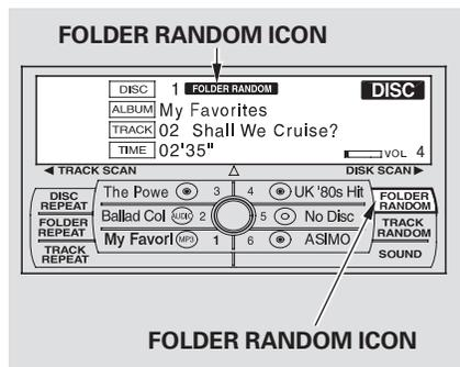
To play the tracks of the current folder in random order, use the interface selector to scroll down, select FOLDER RANDOM with the interface knob, and press ENTER on the interface selector. As a reminder, you will see FOLDER RANDOM next to the disc number on the screen. To turn this feature off, highlight FOLDER RANDOM (if not already highlighted), and press ENTER on the selector again.
