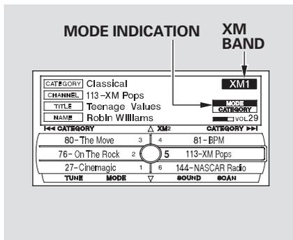
**Preset** — You can store up to 12 preset channels using the six preset buttons. Each button stores one channel from the XM1 band and one channel from the XM2 band.
