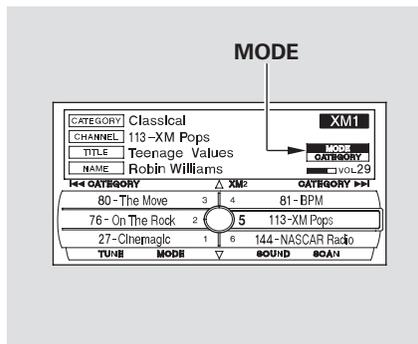
**MODE** – To switch between the category mode and channel mode, press and hold the DISP/MODE button until the mode changes. The CATEGORY or CHANNEL mode is displayed on the screen.
