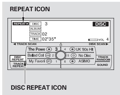
To replay the current disc continuously, use the interface selector to scroll down, select DISC REPEAT, and press ENTER on the interface selector. As a reminder, you will see REPEAT next to DISC on the screen. To turn this feature off, highlight DISC REPEAT (if not already highlighted), and press ENTER on the interface selector again.
