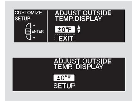
You can adjust the outside temperature shown on the multi-information display in the range of  $-5^{\circ}\text{F}$  ( $-3^{\circ}\text{C}$ ) to  $5^{\circ}\text{F}$  ( $3^{\circ}\text{C}$ ). Adjust the temperature by pressing the ▲ or ▼ button, and enter your selection by pressing the SEL/RESET button. The confirmation screen is shown for 2 seconds, then the CUSTOMIZE ENTRY screen returns.
