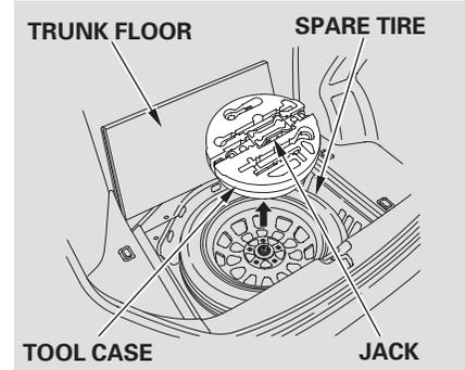
3. Open the trunk, and fold the trunk floor forward.
