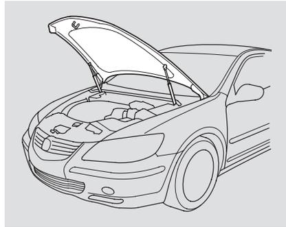
3. Lift the hood up most of the way. The hydraulic supports will lift it up the rest of the way and hold it up.
