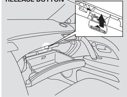
Your vehicle has an owner's manual tray inside the glove box. To open the tray, push the release button up.
