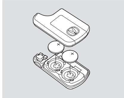
Replace the old batteries with new batteries. Place the batteries so the + side is facing up. Snap the two halves of the remote case back together.
