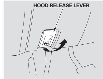
1. Park the vehicle, and set the parking brake. Pull the hood release lever located under the lower left corner of the dashboard. The hood will pop up slightly.
