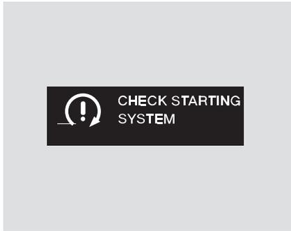
If there is a problem with the starting system, you will see a “CHECK STARTING SYSTEM” message on the multi-information display when the ignition switch is turned to ON (II). You will also see this message when the auto control mode of the starting system has a problem.
