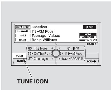
To change channels, press the TUNE button, or scroll down with the interface selector, select TUNE, and press ENTER on the selector. Then turn the interface knob to the desired channel. In the category mode, you can only select channels within that category.
