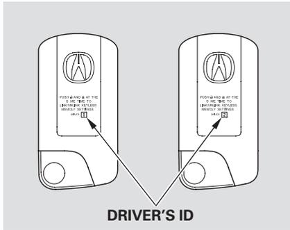
When you unlock the door with your remote, each remote activates the keyless memory settings related to that remote. The driver's ID (Driver 1 or Driver 2) is shown on the back of each remote.
