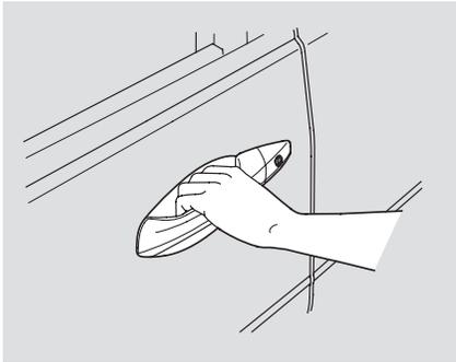
The handle of each front door has a sensor. That sensor works with the remote so you can automatically unlock/lock the door(s).
