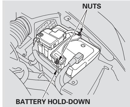
If you are replacing the bulb on the driver's side, remove the battery cover (see page 332), then remove the battery hold-down by removing the two nuts with a 10 mm wrench. Then carefully slide the battery toward the engine to access the bulb.
