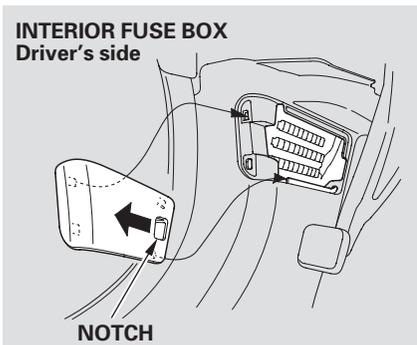
The fuses are located in five fuse boxes. The interior fuse boxes are located under the dashboard on the driver's and passenger's side.
