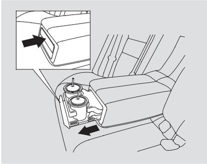
The rear beverage holder is in the rear seat armrest. Open the beverage holder by pushing the front of it.
