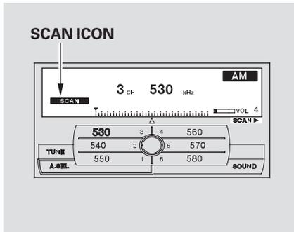
**SCAN** – The SCAN function samples all stations with strong signals on the selected band. To activate it, press the SCAN button, then release it.
