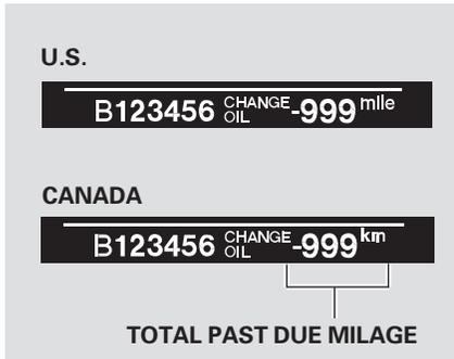
When you press the SEL/RESET button to select the engine oil life minder, the message “CHANGE OIL” along with the maintenance item code, and the total negative mileage after the oil life became 0 percent, will be displayed on the lower part of the multi-information display.
