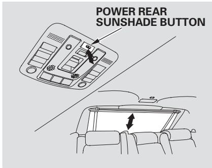
With the ignition switch in the ON (II) position, push the power sunshade button on the ceiling console to raise the rear sunshade. Push the button again to lower it.
