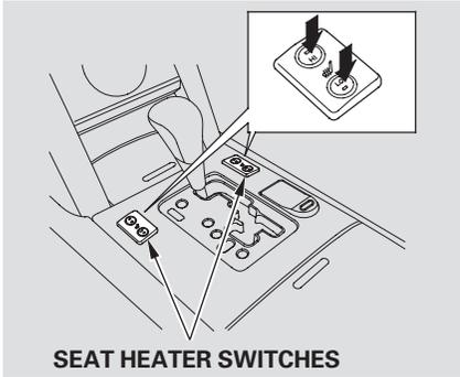
Both front seats are equipped with seat heaters. The passenger seat only has heaters in the seat bottom because of the side airbag system. The ignition switch must be in the ON (II) position to use the heaters. Push the top of the switch, HI, to rapidly heat up the seat. After the seat reaches a comfortable temperature, select LO by pushing the bottom of the switch. This will keep the seat warm.
