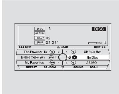
2. "NO DISC" is shown on the screen for an empty position in the changer. When the green load indicator comes on and you see "LOAD" in the upper display, insert the disc into the slot. Insert it only about halfway; the drive will pull it in the rest of the way.
