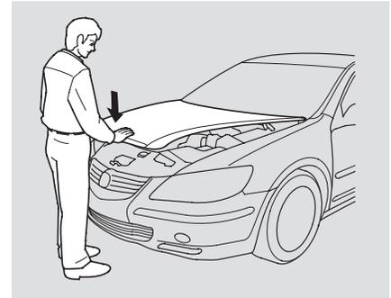
To close the hood, lower the hood to about a foot (30 cm) above the fender, then firmly press down on the front edge of the hood. Make sure it is securely latched.
