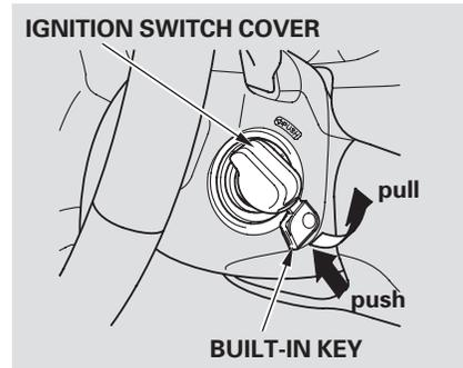
To remove the ignition switch cover, insert the built-in key (see page 141), then pull the cover out by pulling the built-in key while pushing it.
