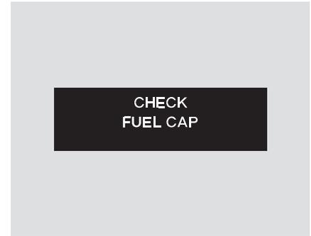
If your fuel cap is loose or missing, a “CHECK FUEL CAP” message appears on the multi-information display after you turn the ignition switch to ON (II), after you start the engine or while you are driving. Turn the ignition switch off and confirm the fuel cap is installed. If it is, loosen the cap, then retighten until it clicks at least once.
