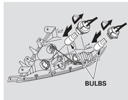
6. Determine which of the two bulbs is burned out: turn signal or back-up light.
