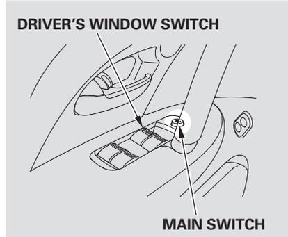
If the MAIN switch is pushed down (OFF), the passenger windows cannot be raised or lowered. Keep the MAIN switch off when you have children in the vehicle so they do not injure themselves by operating the windows unintentionally.
