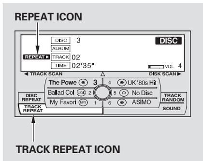
To replay the current track continuously, use the interface selector to scroll down, select TRACK REPEAT, and press ENTER on the interface selector. As a reminder, you will see REPEAT next to TRACK on the screen. To turn this feature off, highlight TRACK REPEAT (if not already highlighted), and press ENTER on the interface selector again.
