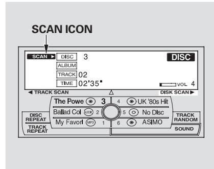
When you press and hold the SCAN button until you hear a beep or scroll down and push the interface selector to the right, the first track of the current disc plays for about 10
