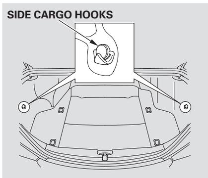
There are hooks on the floor and both sides of the trunk. They can be used to install the cargo net for securing items. The side cargo hooks are designed to hold light items (maximum load: 6 lbf or 3 kgf for each hook). Heavy objects may damage the side hooks.
