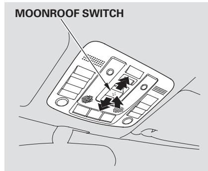
To open the moonroof fully, pull back the moonroof switch firmly. The moonroof opens all the way. To stop the moonroof from opening fully, push the switch forward briefly.
