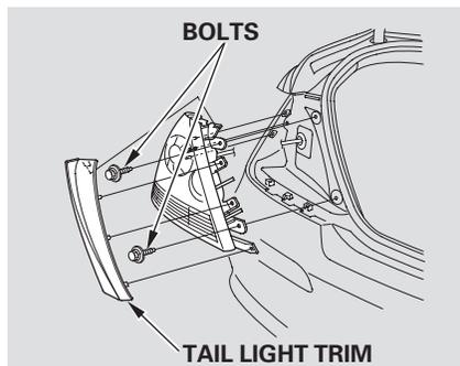
3. Carefully pry in the top or bottom edge of the with a small flat-tipped screwdriver, and pull the trim straight back.
