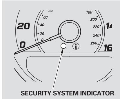
Once the security system is set, opening any door or the hood without using the built-in key or the remote will cause it to sound. It also sounds if the radio is removed from the dashboard or the audio system wiring is cut.
