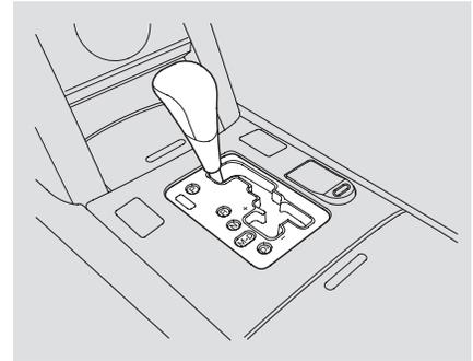
To shift from any position, press firmly on the brake pedal and slide the lever along the guide on the console. You cannot shift out of Park when the ignition switch is in the LOCK (0) or ACCESSORY (I) position.
