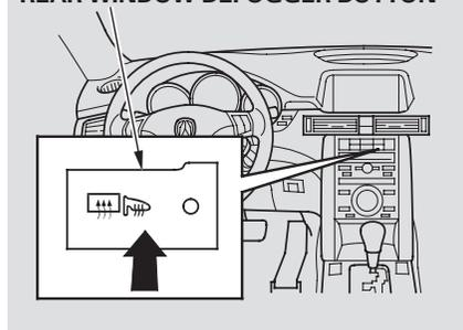
The rear window defogger clears fog, frost, and thin ice from the window. Push the defogger button to turn it on and off. Pushing this button also turns the mirror heaters on and off. The indicator in the button comes on to show the defogger is on. If you do not turn it off, the defogger will shut itself off after 5 to 40 minutes (depending on the ambient temperature). It also shuts off when you turn off the ignition switch. You
