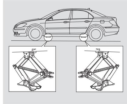
7. Place the jack under the jacking point nearest the tire you need to change. It is pointed to by a  $\triangle$  mark molded into the underside of the body. Turn the end bracket clockwise until the top of the jack contacts the jacking point. Make sure the jacking point tab is resting in the jack notch.
