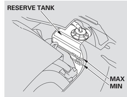
Look at the coolant level in the radiator reserve tank. Make sure it is between the MAX and MIN lines. If it is below the MIN line, see **Adding Engine Coolant** on page [308](#).
