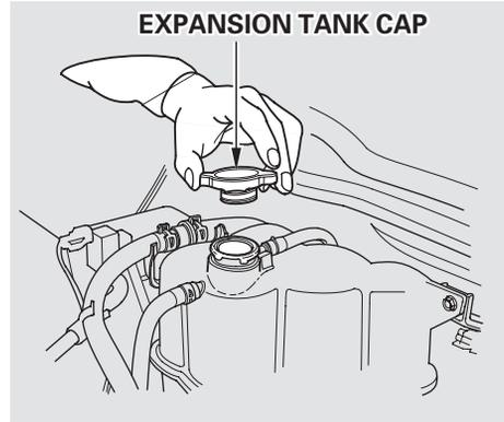
13. Fill the expansion tank to about 1 in. (2.5 cm) above the MAX line. Put the cap back on the tank, only tighten it to the first stop. Start the engine and let it run until it warms up (the radiator cooling fan comes on at least twice).
