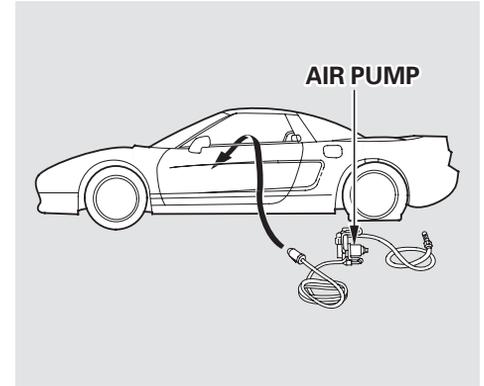
5. Place the air pump near the flat tire. Open the nearest window, and route the air pump's power cord through the open window.
