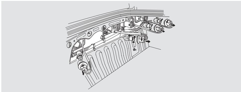
The bulbs for the taillights, tail/stoplights, rear turn signals, and back-up lights are behind the trunk liner.
