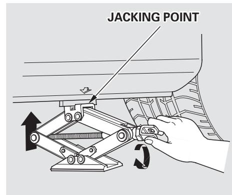
8. Locate the jacking point nearest the tire you need to change. It is pointed to by an arrow molded into the underside of the body. Place the jack under the jacking point. Turn the end bracket clockwise until the top of the jack contacts the jacking point. Make sure the jacking point tab is resting in the jack notch.
