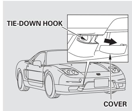
For very short distances such as freeing the car, you can use the tie-down hook on the lower right of the front bumper. Remove the cover to expose the hook. This hook is not for open-road towing (see **Emergency Towing**, page [268](#) ).
