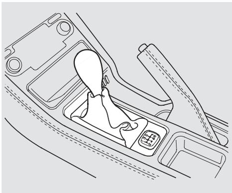
The manual transmission is synchronized in all forward gears for smooth operation. It has a lockout so you cannot shift directly from Fifth to Reverse instead of sixth (see page 150). When shifting up or down, make sure you push the clutch pedal down all the way, shift to the next gear, and let the pedal up gradually. When you are not shifting, do not rest your foot on the clutch pedal. This can cause your clutch to wear out faster.
