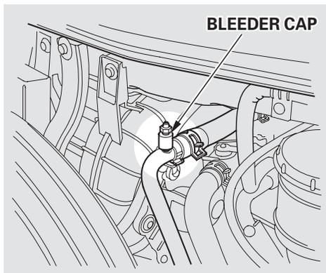
9. Remove the bleeder cap from the top of the heater inlet.
