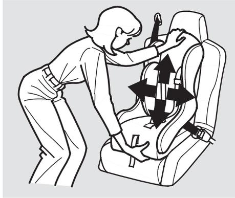
6. Push and pull the child seat forward and from side to side to verify that it is secure enough to stay upright during normal driving maneuvers. If the child seat is not secure, unlatch the belt, allow it to retract fully, then repeat these steps.
