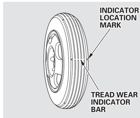
The folding spare tire has a shorter tread life than a regular tire. Replace it when you can see the tread wear indicator bars. The spare tire is not designed to be mounted on a regular wheel, and the compact wheel is not designed for mounting a regular tire.
