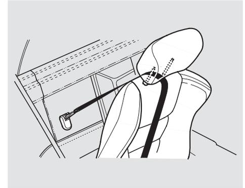
Pass the strap between the top of the seat and the bottom of the head restraint.
