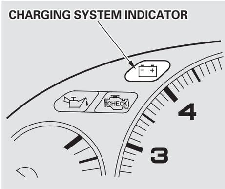
This indicator should come on when the ignition switch is ON (II), and go out after the engine starts. If it comes on brightly when the engine is running, it indicates that the charging system has stopped charging the battery.
