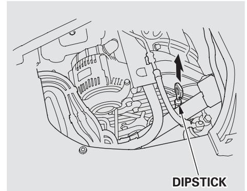
Check the engine oil level every time you fill the car with fuel. Wait a few minutes after turning the engine off before you check the oil.
