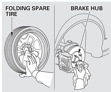
11. Before you put on the folding spare tire, wipe any dirt off the mounting surface of the wheel and hub with a clean cloth. This will assure a tight, even contact between the wheel and hub.
