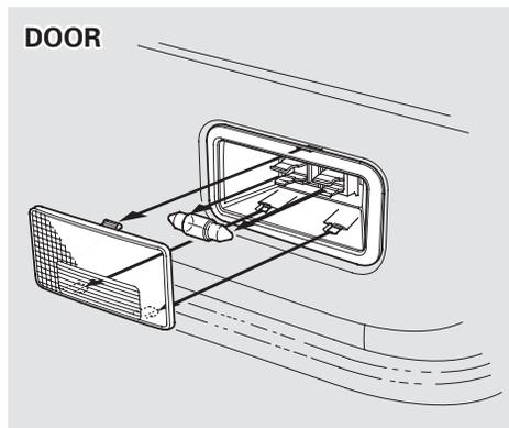
1. Remove the lens by carefully prying on the edge with your fingernail or a small flat-tip screwdriver. The two lenses on the roof-mounted interior light come out as a unit.
