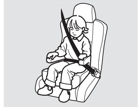
If a child needs a booster seat, we recommend choosing a style that allows the child to use the lap/shoulder belt directly, without a shield, as shown.
