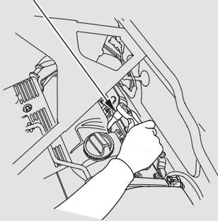
6. Torque the spark plug. (If you do not have a torque wrench, tighten the spark plug two-thirds of a turn after it contacts the cylinder head.)
