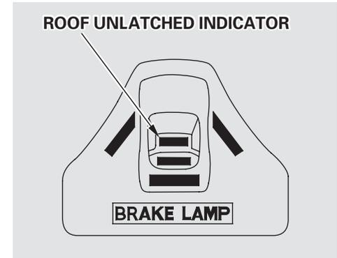
This indicator lights when the roof is installed if either release lever is not fully locked. Check both release levers to make sure they are locked. This indicator also lights when the roof is removed but is not properly stored in the holder.
