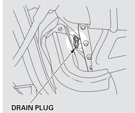
7. Loosen the drain plugs on the engine.
