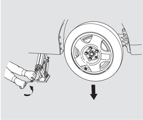
18. Lower the car to the ground and remove the jack.
