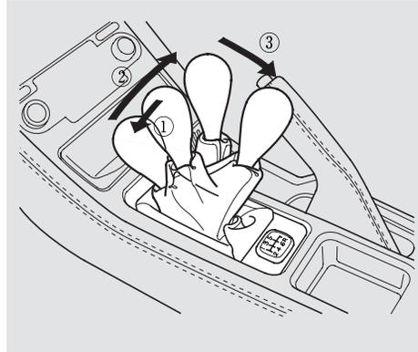
1. With the clutch pedal depressed, move the shift lever to the First/Second gear side of the Neutral gate, then shift to Reverse.
