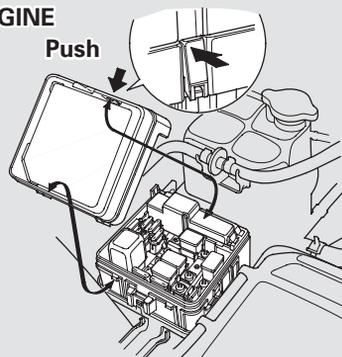
The engine compartment fuse box is located next to the air cleaner housing. To open, push the tab as shown.
