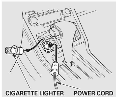
6. Remove the cigarette lighter from its socket and plug the power cord end into the socket. Make sure the key is in the ignition switch at LOCK (0).
