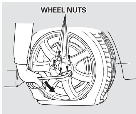
7. Loosen the five wheel nuts 1/2 turn with the wheel wrench.
