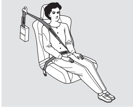
Your Acura has automatic seat belt tensioners for added protection during a moderate to severe frontal collision.
