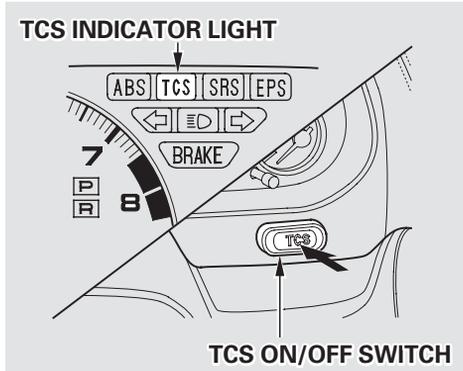
This switch is on the dashboard behind the right control pod. It lets you turn the Traction Control System on and off. You cannot turn off the TCS while the TCS indicator light is flashing.
