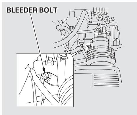
10. Loosen the bleeder bolt on top of the engine.
