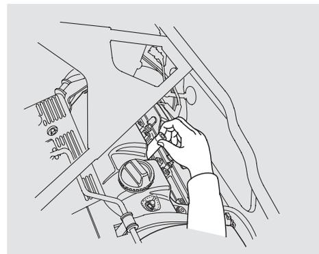
5. Put the new spark plug into the socket, then screw it into the hole. Screw it in by hand so you do not crossthead it.
