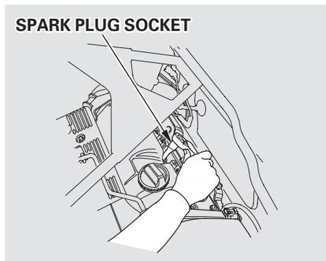
4. Remove the spark plug with a five-eighths inch (16 mm) spark plug socket.
