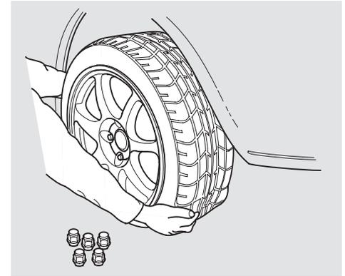
10. Remove the wheel nuts and flat tire. Temporarily place the flat tire on the ground with the outside surface of the aluminum wheel facing up. Placing the wheel face down could mar its finish.
