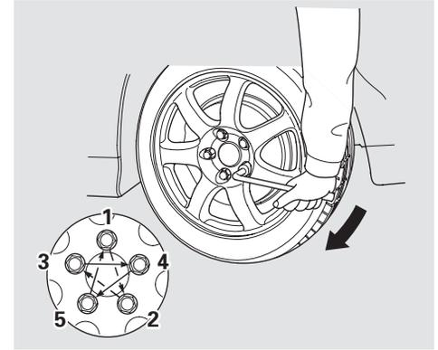
6. Remove the folding spare tire and install the original tire and wheel nuts. Lower the car and tighten the wheel nuts securely in a criss-cross pattern. Tighten to: 80 lbf·ft (108 N·m , 11 kgf·m)
