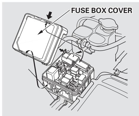
3. Open the rear window and engine cover. Locate the engine compartment fuse box on the driver's side of the compartment. Remove the fuse box cover.
