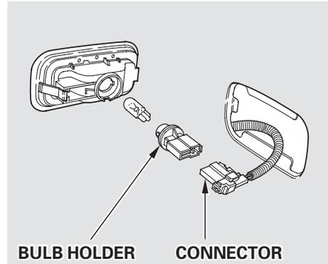
3. Remove the electrical connector from the bulb holder by squeezing the connector and pulling them apart.
