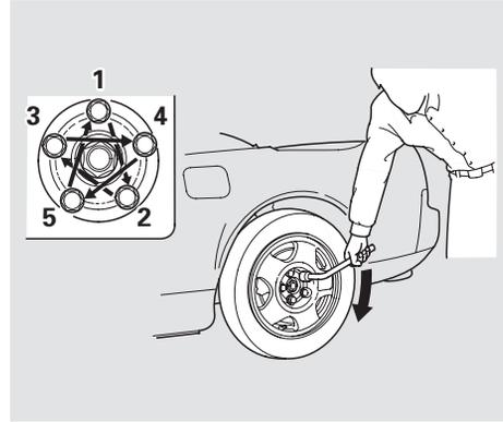
19. Tighten the wheel nuts securely in the same crisscross pattern. Have the wheel nut torque checked at the nearest automotive service facility.
