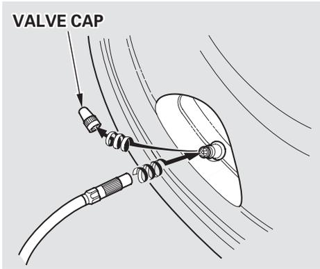
13. Unscrew the valve cap from the folding spare tire's air valve by turning it counterclockwise. Then screw on the air pump hose.
