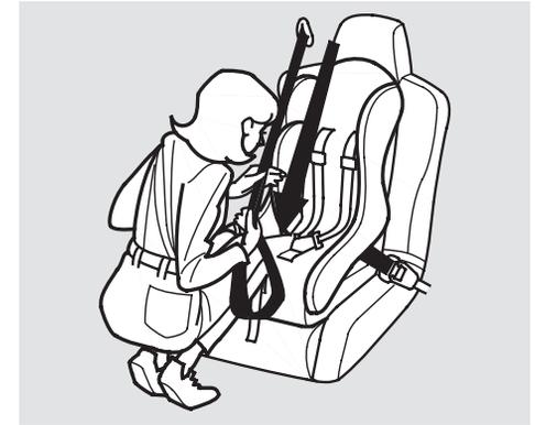
3. To activate the lockable retractor, slowly pull the shoulder part of the belt all the way out until it stops, then let the belt feed back into the retractor (you might hear a clicking noise as the belt retracts).
