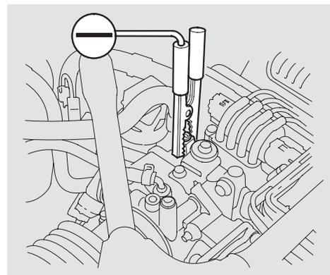
5. Connect the second jumper cable to the negative (-) terminal on the booster battery. Connect the other end to the boss on the intake manifold as shown. Do not connect this jumper cable to any other part of the engine.
