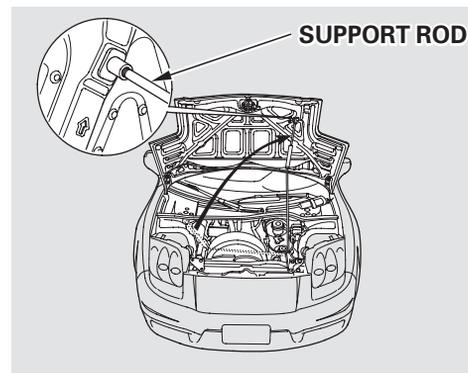
3. Pull the support rod out of its clip and insert the end into the square hole on the right side of the hood.
