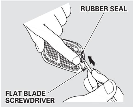
1. Use your fingernail to lift the rubber seal along the back edge of the side marker lens.
