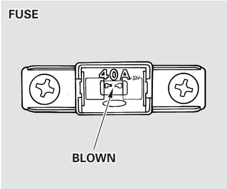
3. Check each of the large fuses in the under-hood and engine compartment fuse boxes by looking through the top at the wire inside. Removing these fuses requires a Phillips-head screwdriver.
