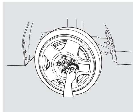
12. Put on the folding spare tire with the air valve toward the bottom. Put the wheel nuts back on finger-tight, then tighten them in a crisscross pattern with the wheel wrench until the wheel is firmly against the hub. Do not try to tighten them fully. Inflate the folding spare tire only when it is on the car. Inflating it while it is lying on the ground may trap stones or other foreign matter between the tire and the wheel rim.
