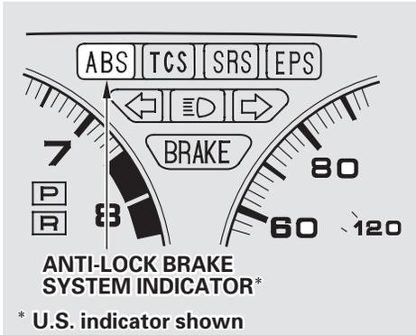
The ABS is self-checking. If anything goes wrong, the ABS indicator on the instrument panel comes on (see page 50). This means the anti-lock function of the braking system has shut down. The brakes still work like a conventional system without anti-lock, providing normal stopping ability. You should have the dealer inspect your car as soon as possible.
