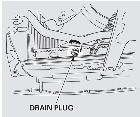
4. Remove the drain plug from the bottom of the radiator.
