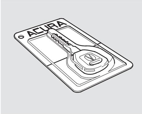
You should also receive a small case containing a learning key. It is used by the Acura dealer to code replacement keys to your car's Immobilizer System. It must not be used in your car's ignition switch. Store the learning key with the key number plate in a safe place.
