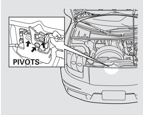
Clean the hood latch assembly with a mild cleaner, then lubricate it with a multipurpose grease. Lubricate all the moving parts, including the pivot. Follow the time and distance recommendations in the Maintenance Schedule. If you are not sure how to clean and grease the latch, contact your Acura dealer.
