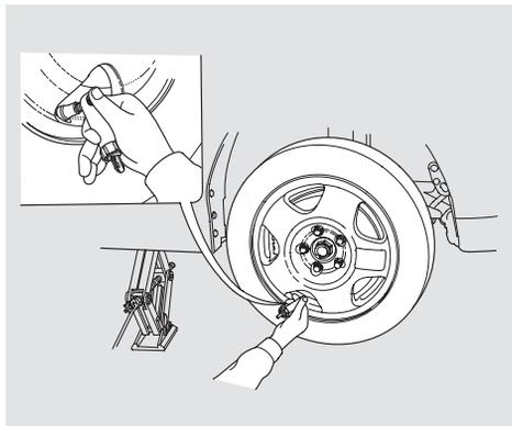
15. After about five minutes, unscrew the air pump hose and check the pressure with the supplied pressure gauge.
