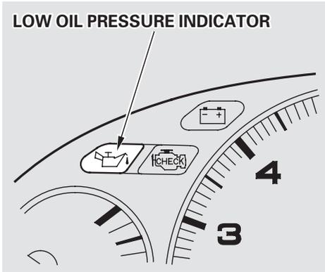
This indicator should light when the ignition switch is ON (II), and go out after the engine starts. It should never come on when the engine is running. If it starts flashing, it indicates that the oil pressure dropped very low for a moment, then recovered. If the indicator stays on with the engine running, it shows that the engine has lost oil pressure and serious engine damage is possible. In either case, you should take immediate action.
