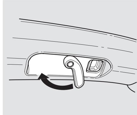
9. Secure the roof by turning each release lever until the lock tab clicks forward. Pull on the levers to make sure they are locked. If the release levers are locked correctly, the roof unlatched indicator will not light when you turn the ignition ON (II).
