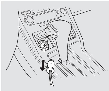
16. When finished, reach in and turn the ignition switch to LOCK (0). Unplug the air pump power cord.
