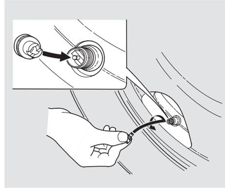
3. Remove the rubber cover on top of the valve cap. Use the notch on the valve cap to unscrew the spare tire valve core until the air starts coming out. Use your hand to shield your eyes. The valve core can fly out under pressure.
