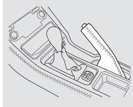
To apply the parking brake, pull the lever up fully. To release it, pull up slightly, push the button, and lower the lever. The parking brake light on the instrument panel should go out when the parking brake is fully released (see page 49). If you try to drive the vehicle without releasing the parking brake, the ABS indicator may come on, and the ABS may not work properly.
