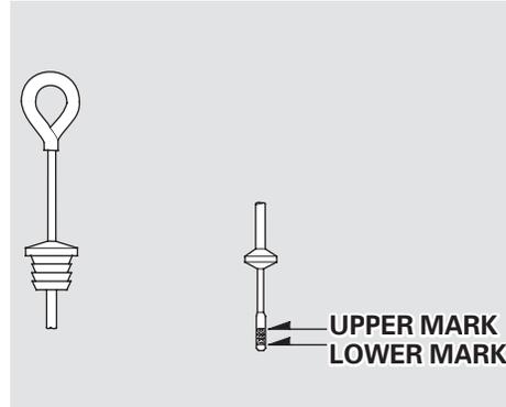
3. Insert the dipstick into the transmission. Make sure the notch in the rubber cap fits in the dipstick guide and that you push the dipstick in all the way.
