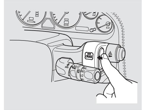
1. Push in the Cruise Control Master Switch on the right pod. The indicator by the switch will light.
