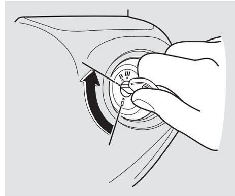
14. Reach into the car and turn the ignition switch to ACCESSORY (I). This will start the air pump to inflate the tire.
