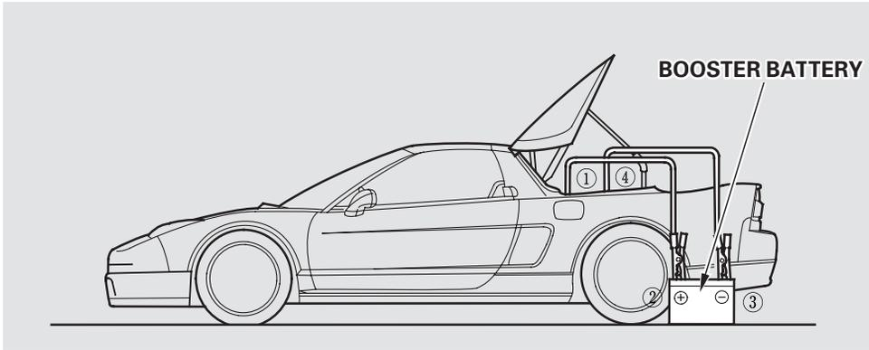
6. If the booster battery is in another car, have an assistant start that car and run it at a fast idle.
