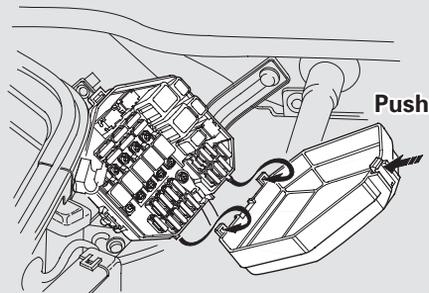
The under-hood fuse box is located in the front of the engine compartment on the passenger's side. To open it, push the tab as shown.
