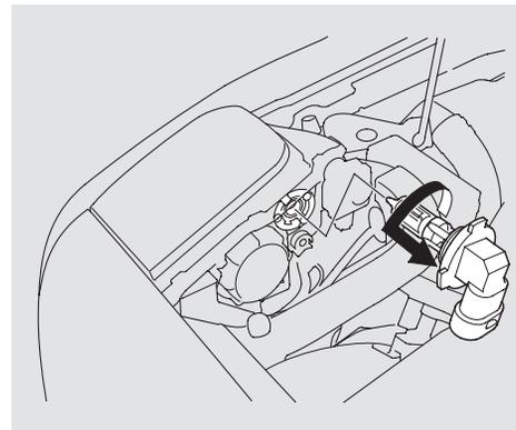
3. Remove the bulb by turning it approximately one-quarter turn counterclockwise.
