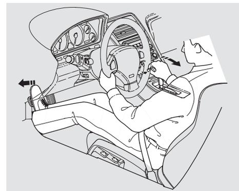
**Park (P)** – This position mechanically locks the transmission. Use Park whenever you are turning off or starting the engine. To shift out of Park, you must press on the brake pedal and have your foot off the accelerator pedal. Press the release button on the side of the shift lever to move it.
