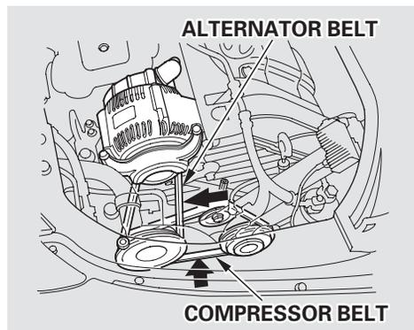
You should check the condition of the two engine belts every 2 years. Examine the edges of each belt for cracks or fraying. Check the tension of each belt by pushing on it at the point shown in the diagram.
