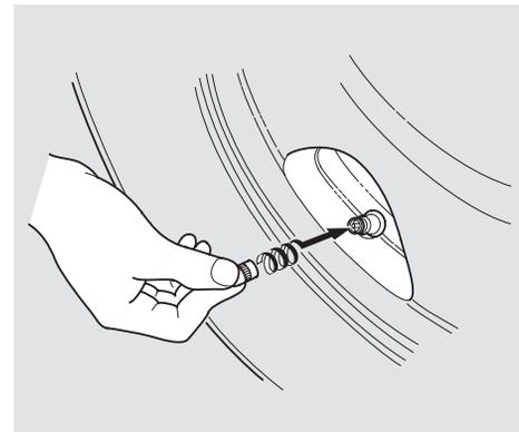
17. Screw the valve cap on the valve tightly with your hands.
