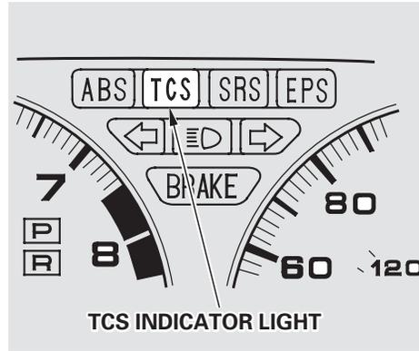
When driving on a loose or slippery road surface, you may notice that the engine does not respond to the accelerator in the same way it does at other times. This is a sign the TCS is activating. You will see the TCS indicator light flash.
