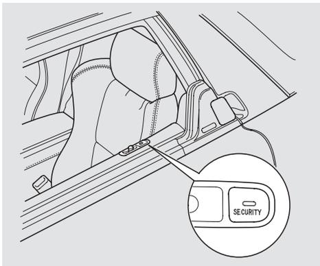
The security system helps to protect your car and valuables from theft. The horn sounds and all the exterior lights flash if someone attempts to break into your car or remove the radio. The system alarms continue for two minutes unless you turn it off manually. To turn the system off, unlock either door with the key.
