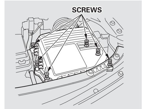
3. Loosen the six Phillips-head screws around the edge of the air cleaner housing cover. Remove the air cleaner housing cover and set it aside.
