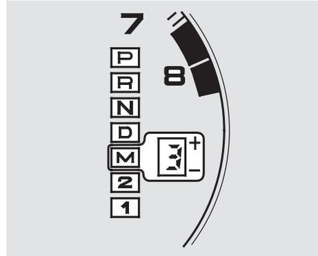
This display is in the tachometer. It shows you the position of the console shift lever. The illuminated number next to the "M" indicator shows you the gear you have selected when selecting 3/M position.
