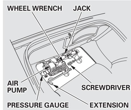
4. Open the trunk (see page 68). Lift the cover; remove the jack, wheel wrench, extension, air pump, pressure gauge, and screwdriver from the trunk. The tools may become very hot while the car is being driven. Wear gloves or use a protective cloth when handling the tools.
