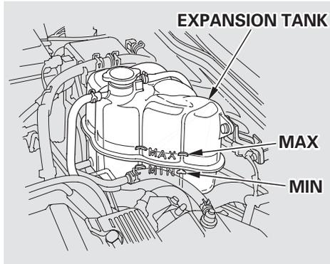
Look at the coolant level in the expansion tank. Make sure it is between the MAX and MIN lines. If it is below the MIN line, see **Adding Engine Coolant** on page 185 for information on adding the proper coolant.
