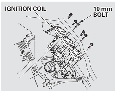
2. Disconnect the three ignition coils from the wire harness by squeezing the harness end of each connector and pulling.
