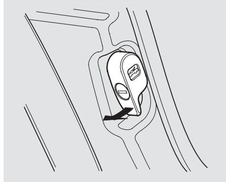
4. Open the door. Locate the rear window release handle on the rear of the driver's door opening, next to the seat. Pivot this handle towards the driver's seat. The rear window will pop up slightly.
