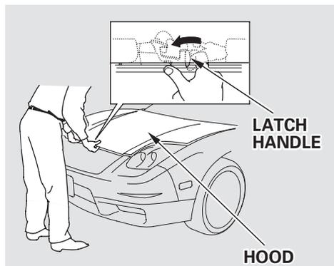
2. Standing in front of the car, put your fingers under the front edge of the hood to the right of center. Slide your hand to the left until you feel the hood latch handle. Push this handle to the left until it releases the hood. Lift the hood.
