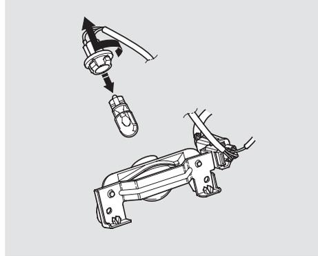
2. Remove the socket from the light assembly by turning it one-quarter turn counterclockwise.
