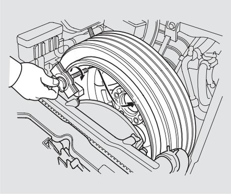
7. Store the folding spare tire in the front compartment with the outside surface of the wheel contacting the bracket of the spare tire well. Securely tighten the wing bolt.
