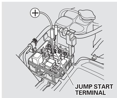
4. Connect one jumper cable to the JUMP START terminal in the fuse box. Connect the other end to the positive (+) terminal on the booster battery.
