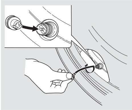
4. As the tire deflates, it will fold back to its original shape. When the air stops coming out of the tire, use the notch on the valve cap to tighten the valve core.
