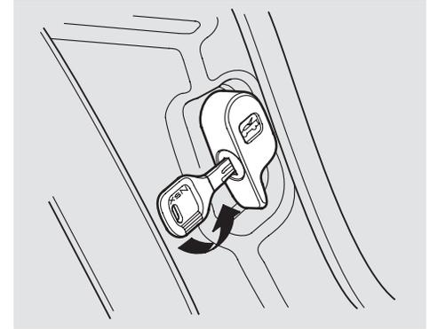
To prevent anyone from getting to the roof panel and the engine when you park the car with the roof removed, lock the rear window release lever with the master key.
