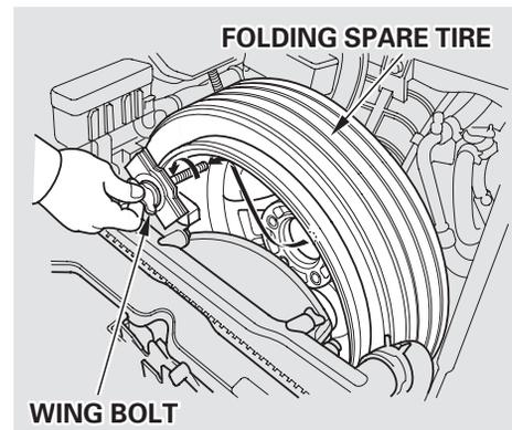
3. Open the hood (see page [135](#)). Unscrew the wing bolt holding the folding spare tire. Remove the folding spare tire from the compartment. The wing bolt and wheel may be very warm from the air passing through the radiator. Use a cloth or gloves (not provided) to protect your hands when removing the spare tire.
