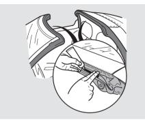
Dust is the main cause of creaks or other sounds coming from the roof. Regularly clean the roof panel and body seals with glass cleaner and a soft cloth.
