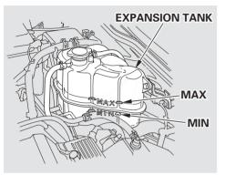
Look at the coolant level in the expansion tank. Make sure it is between the MAX and MIN lines. If it is below the MIN line, see **Adding Engine Coolant** on page 185 for information on adding the proper coolant.
