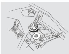
To add oil, unscrew and remove the engine oil fill cap on top of the left valve cover. Pour in the oil, and replace the engine oil fill cap. Tighten it securely. Wait a few minutes and recheck the oil level. Do not fill above the upper mark; you could damage the engine.
