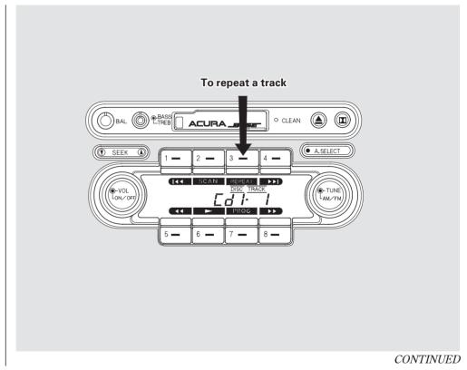
To search for a particular program on a disc, press SCAN. The system will skip forward to the next track and begin to play it. If you do not touch any of the controls, the system skips to the beginning of the next track after ten seconds and begins to play that. When the system gets to a track you want to hear all the way through, press SCAN again. You can only scan tracks on the disc currently being played.
