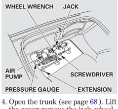
Lift the cover; remove the jack, wheel wrench, extension, air pump, pressure gauge, and screwdriver from the trunk. The tools may become very hot while the car is being driven. Wear gloves or use a protective cloth when handling the tools.
