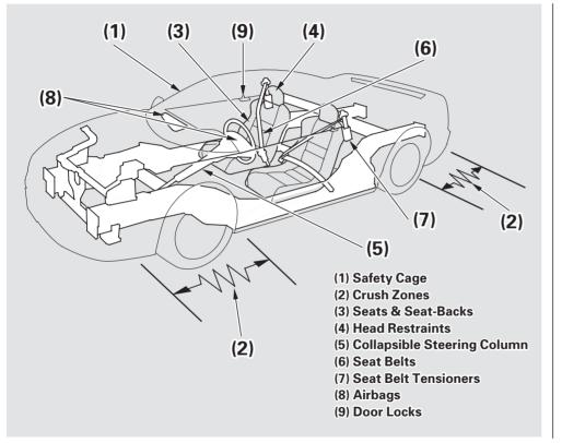
Your car is equipped with many features that work together to protect you and your passenger during a crash.
