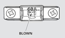
3. Check each of the large fuses in the under-hood and engine compartment fuse boxes by looking through the top at the wire inside. Removing these fuses requires a Phillips-head screwdriver.
