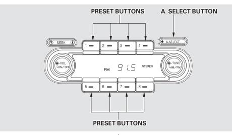
A. SELECT does not erase the stations you have manually preset. When you return to your normal reception area, turn off A. SELECT by pressing the button again. The light in the button goes out and the preset buttons can then select the stations you originally set.
