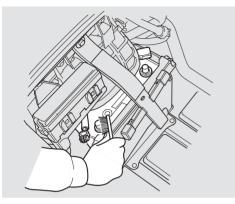
If the terminals are severely corroded, clean them with baking soda and water. Then use a wrench to loosen and remove the cables from the terminals. Always disconnect the negative (-) cable first and reconnect it last. Clean the battery terminals with a terminal cleaning tool or wire brush. Reconnect and tighten the cables, then coat the terminals with grease. If you need to connect the battery to a charger, disconnect both cables to prevent damage to the car's electrical system.
