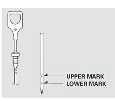
4. Remove the dipstick again and check the level. It should be between the upper and lower marks.
