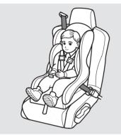
The passenger's airbag poses serious risks to small children. If the vehicle seat is too far forward, or the child's head is thrown forward during a collision, or the child is unrestrained or improperly restrained, an inflating airbag can kill or seriously injure the child.
