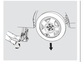
18.Lower the car to the ground and remove the jack.
