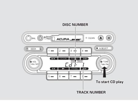
When that disc ends, the next disc in the magazine is loaded and played. When disc 6 has completed, the system will return to disc 1. To select another disc, press PROG. The next CD in the changer is loaded and starts to play from the first track. The new CD and track numbers are displayed.
