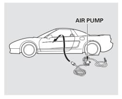
5. Place the air pump near the flat tire. Open the nearest window, and route the air pump's power cord through the open window.
