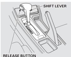
The console shift lever has seven positions. It must be in Park or Neutral to start the engine.
