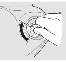
14.Reach into the car and turn the ignition switch to ACCESSORY (I). This will start the air pump to inflate the tire.
