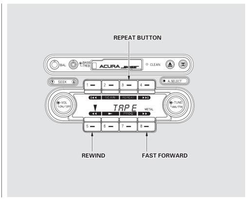
The REPLAY function I◄ is similar to REPEAT. When you press this button, the system immediately goes into rewind. The light in the REPLAY button flashes during rewind. When it senses a silent period on the tape, the system stops rewinding and goes back to PLAY. Unlike REPEAT, this function replays a selection only once. If you do not press I◄ again, the tape will play straight through.
