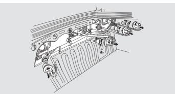
The bulbs for the taillights, tail/stoplights, rear turn signals, and back-up lights are behind the trunk liner.
