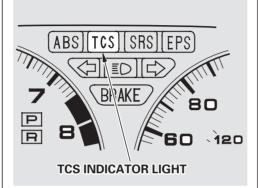
When driving on a loose or slippery road surface, you may notice that the engine does not respond to the accelerator in the same way it does at other times. This is a sign the TCS is activating. You will see the TCS indicator light flash. You should still install winter tires on your car during the winter. Exercise the same caution in winter driving as you would if your car was not equipped with TCS.
