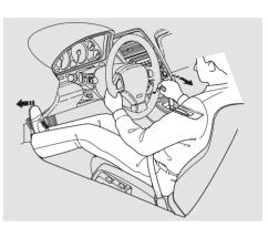
**Park (P)** – This position mechanically locks the transmission. Use Park whenever you are turning off or starting the engine. To shift out of Park, you must press on the brake pedal and have your foot off the accelerator pedal. Press the release button on the side of the shift lever to move it. If you have done all of the above and still cannot move the lever out of Park, see Shift Lock Release on page 156.
