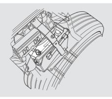
Check the battery condition by looking at the test indicator window on the battery. The label on the battery explains the test indicator's colors. Check the battery terminals for corrosion (a white or yellowish powder). To remove it, cover the terminals with a solution of baking soda and water. It will bubble up and turn brown. When this stops, wash it off with plain water. Dry off the battery with a cloth or paper towel. Coat the terminals with grease to help prevent future corrosion.
