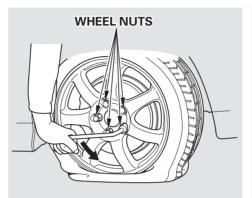
7. Loosen the five wheel nuts 1/2 turn with the wheel wrench.
