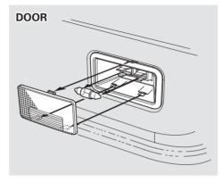
1. Remove the lens by carefully prying on the edge with your fingernail or a small flat-tip screwdriver. The two lenses on the roof-mounted interior light come out as a unit.
