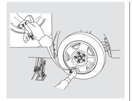
15.After about five minutes, unscrew the air pump hose and check the pressure with the supplied pressure gauge. Inflate to:
