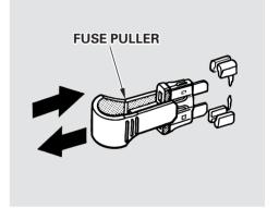
4. Check the smaller fuses by pulling out the fuse with the fuse puller provided in the interior fuse box.
