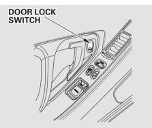
Each door has a door lock switch. Either switch locks and unlocks both doors. Push LOCK to lock both doors, and the top portion of the switch to unlock them.
