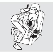
5. After confirming that the belt is locked, grab the shoulder part of the belt near the buckle and pull up to remove any slack from the lap part of the belt. Remember, if the lap part of the belt is not tight, the child seat will not be secure. It may help to put weight on the child seat, or push on the back of the seat, while pulling up on the belt.
