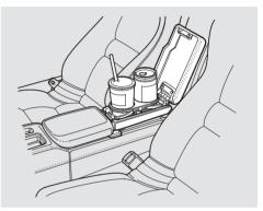
The beverage holder is located in the rear half of the console compartment lid. To use the beverage holder, lift up on the middle of the armrest pad.
