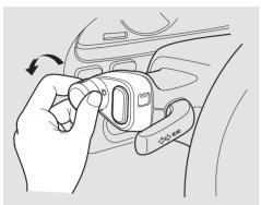
The rotating switch on the left pod controls the lights. Turning this switch to " $\bullet$ " turns on the parking lights, taillights, instrument panel lights, side-marker lights, and rear license plate lights. Turning the switch to " $\bullet$ " turns on the headlights.
