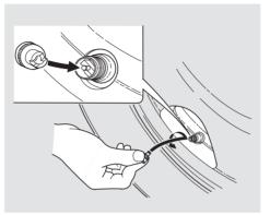
3. Remove the rubber cover on top of the valve cap. Use the notch on the valve cap to unscrew the spare tire valve core until the air starts coming out. Use your hand to shield your eyes. The valve core can fly out under pressure. Keep your fingers and clothing away as the tire deflates and folds back to its compact size.
