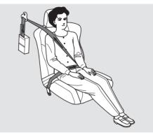
Your Acura has automatic seat belt tensioners for added protection during a moderate to severe frontal collision.
