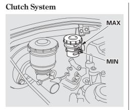
The fluid level should be between the MIN and MAX marks on the side of the reservoir. If it is not, add brake fluid to bring it up to that level. Use the same fluid specified for the brake system.
