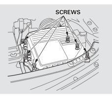
3. Loosen the six Phillips-head screws around the edge of the air cleaner housing cover. Remove the air cleaner housing cover and set it aside.
