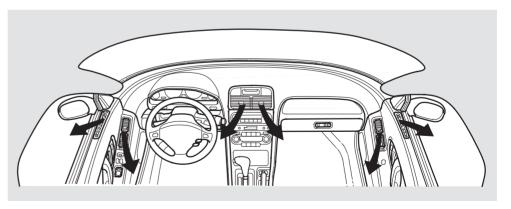
The main air flow is divided between the dashboard/door vents and the floor vents.
