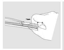
3. Remove the blade from its holder by grasping the tabbed end of the blade. Pull firmly until the tabs come out of the holder. BLADE
