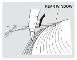
2. Stand just behind the driver's door. Reach under the rear edge of the rear window at its center and raise it. It will stay up by itself.
