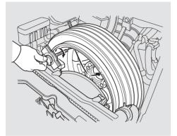
7. Store the folding spare tire in the front compartment with the outside surface of the wheel contacting the bracket of the spare tire well. Securely tighten the wing bolt.
