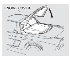
To Close the Rear Window: Snap the support rod back into the clip and lower the engine cover. Pull the rear window down until it is resting on the body, then push on the centre of the back edge until it latches. Make sure it is securely closed before driving away.
