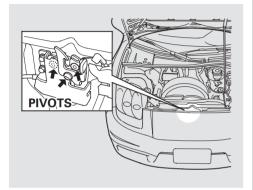
Clean the hood latch assembly with a mild cleaner, then lubricate it with a multipurpose grease. Lubricate all the moving parts, including the pivot. Follow the time and distance recommendations in the Maintenance Schedule. If you are not sure how to clean and grease the latch, contact your Acura dealer.
