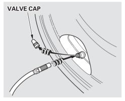
13.Unscrew the valve cap from the folding spare tire's air valve by turning it counterclockwise. Then screw on the air pump hose.
