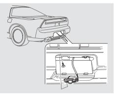
1. Use a Phillips-head screwdriver to remove the two screws holding the license plate light assembly to the bracket. Pull the assembly away from the bracket.
