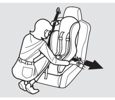
2. With the child seat in position, route the belt through the child seat according to the seat maker's instructions, then insert the latch plate into the buckle.
