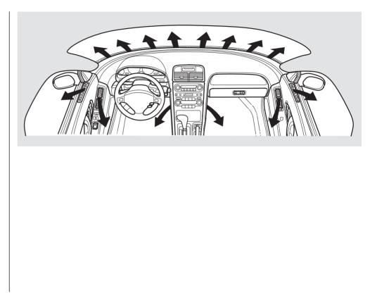
The W button directs the main air flow to the windshield for faster defrosting. It also overrides any MODE selection you may have made. To defrost more quickly, turn the temperature control to 82°F ~86°F (28°C ~30°C).
