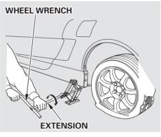
9. Use the extension and wheel wrench as shown to raise the car until the flat tire is off the ground.
