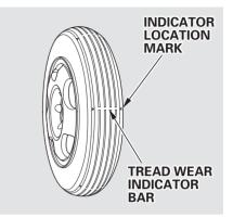
The folding spare tire has a shorter tread life than a regular tire. Replace it when you can see the tread wear indicator bars. The spare tire is not designed to be mounted on a regular wheel, and the compact wheel is not designed for mounting a regular tire. Diagnosing why your engine won't start falls into two areas, depending on what you hear when you turn the key to START (III):
