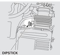
Check the fluid level with the engine at normal operating temperature.
