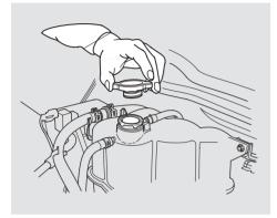
3. Start the engine. Turn the heater temperature control dial to maximum heat and turn off the engine. Make sure the engine and radiator are cool to the touch.
