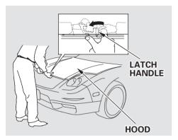
2. Standing in front of the car, put your fingers under the front edge of the hood to the right of center. Slide your hand to the left until you feel the hood latch handle. Push this handle to the left until it releases the hood. Lift the hood. If you can open the hood without lifting the hood latch handle, or the hood latch handle moves stiffly or does not spring back as before, the mechanism should be cleaned and lubricated (see page 199).
