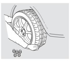
10.Remove the wheel nuts and flat tire. Temporarily place the flat tire on the ground with the outside surface of the aluminum wheel facing up. Placing the wheel face down could mar its finish.
