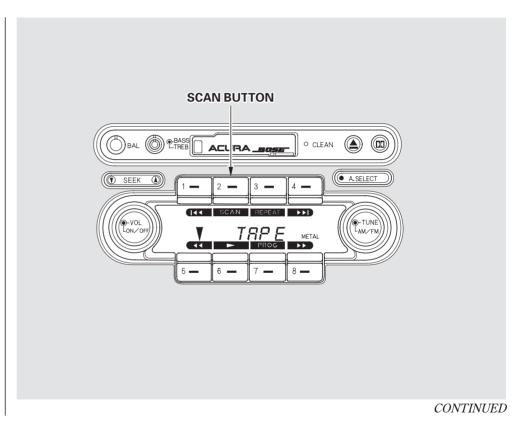
The REPLAY, SKIP and SCAN functions use silent periods on the tape to find the end of a selection. These features may not work satisfactorily on tapes that have almost no gap between songs, a high noise level between songs, or silent periods in the middle of songs.
