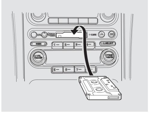
Dolby B noise reduction turns on when you insert a cassette. If the tape was not recorded with Dolby B noise reduction, turn it off by pressing the D button.
