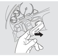
To change between low beams and high beams, pull the turn signal lever as far as it will move towards you, then let go. The blue high beam indicator will light (see page 52). To flash the high beams, pull the turn signal lever back lightly, then release it. The high beams will come on and go off.
