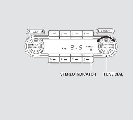
The easiest way to find your favorite stations is to set their frequencies into the eight preset buttons. To do this, tune to the desired station as described previously. Press one of the preset buttons (1-8) and hold it until you hear a beep. You can preset eight stations on each band.
