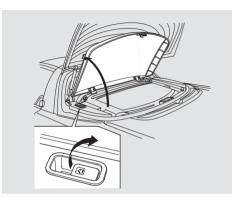
6. Pull up the roof cover release lever and raise the roof cover.
