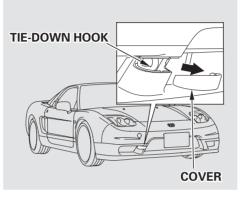
For very short distances such as freeing the car, you can use the tiedown hook on the lower right of the front bumper. Remove the cover to expose the hook. This hook is not for open-road towing (see **Emergency Towing**, page 268). If your car needs to be towed, call a professional towing service or, if you belong to one, an organization that provides roadside assistance. Never tow your car behind another vehicle with just a rope or chain. It is very dangerous.
