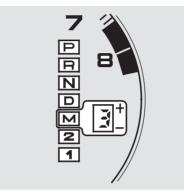
This display is in the tachometer. It shows you the position of the console shift lever. The illuminated number next to the "M" indicator shows you the gear you have selected when selecting 3/M position.
