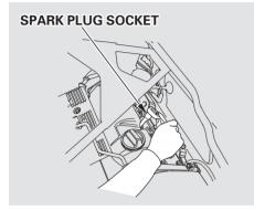
6. Torque the spark plug. (If you do not have a torque wrench, tighten the spark plug two-thirds of a turn after it contacts the cylinder head.) Tightening torque:
