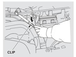
5. Snap the support rod back into its holding clip.
