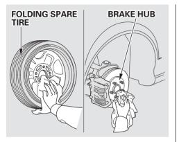
11.Before you put on the folding spare tire, wipe any dirt off the mounting surface of the wheel and hub with a clean cloth. This will assure a tight, even contact between the wheel and hub.
