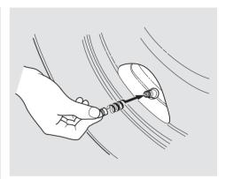
17. Screw the valve cap on the valve tightly with your hands.
