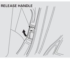
1. Shift to Park or Neutral and set the parking brake. Locate the release handle on the rear of the driver's door opening, next to the seat. Pivot this handle towards the driver's seat. The rear window will pop up slightly.
