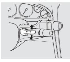
If you move the console shift lever from "D" to "3/M" while the car is moving, the transmission remains in the gear it was in. If you do this while stopped, the transmission selects first gear.
