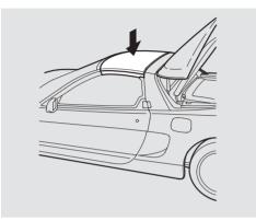
8. Set the roof in place on the car. Make sure all four corners are sitting flush with the car body.
