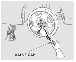
5. Put the rubber cap back on the valve cap. Screw the valve cap back on the folding spare tire valve.
