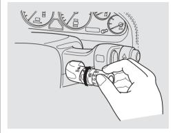
The lever on the right pod controls the windshield wipers and washers. The rotary switch at the end of the lever has three positions: INT: intermittent LO: low speed HI: high speed
