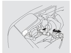
1. Remove the socket from the headlight assembly by turning it one-quarter turn counterclockwise.
