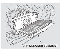
4. Remove the old air cleaner element. Carefully clean the inside of the air cleaner housing with a damp rag.
