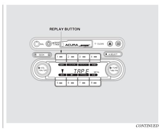
The SKIP function  $\blacktriangleright i$  allows you to skip over a song or other passage. When you press this button, the system goes into fast forward until it senses a silent period on the tape. The light in the SKIP button flashes during fast forward. When the system finds a silent period, it goes back to PLAY.
