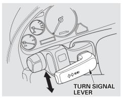
Signal a turn or lane change with this lever. Push down on the lever to signal a left turn, and up to signal a right turn. If you push it up or down all the way, the turn signal continues to blink even when you release the lever. It shuts off automatically as you complete the turn. To signal a lane change, push lightly on the turn signal lever in the proper direction and hold it. The lever will return to the center position as soon as you release it.
