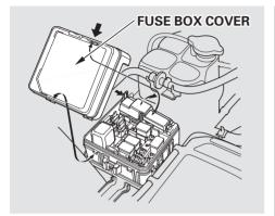
3. Open the rear window and engine cover. Locate the engine compartment fuse box on the driver's side of the compartment. Remove the fuse box cover.
