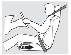
Any driver who sits too close to the steering wheel is at risk of being seriously injured or killed by striking the steering wheel, or from being struck by an inflating airbag during a crash. To reduce the chance of injury, wear your seat belt properly, sit upright with your back against the seat, and move the seat away from the steering wheel to the farthest distance that allows you to maintain full control of the car.
