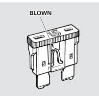
5. Look for a burned wire inside the fuse. If it is burned, replace it with one of the spare fuses of the same rating or lower.
