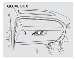
Open the glove box by squeezing the handle. Close it with a firm push. Lock or unlock the glove box with the master key.
