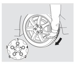
6. Remove the folding spare tire and install the original tire and wheel nuts. Lower the car and tighten the wheel nuts securely in a crisscross pattern. Tighten to: 80 lbf·ft (108 N·m , 11 kgf·m)
