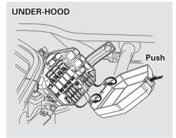
The under-hood fuse box is located in the front of the engine compartment on the passenger's side. To open it, push the tab as shown.
