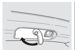
9. Secure the roof by turning each release lever until the lock tab clicks forward. Pull on the levers to make sure they are locked. If the release levers are locked correctly, the roof unlatched indicator will not light when you turn the ignition ON (II). 10.Close the roof cover and snap the hook onto the window frame. Close the rear window.
