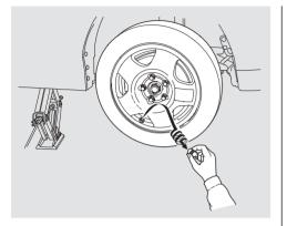
2. Unscrew and remove the folding spare tire valve cap.
