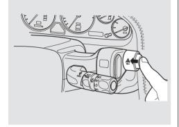
Push the large red button on the right pod to turn on the hazard warning lights (four-way flashers). This causes all four outside turn signals and both indicators in the instrument panel to flash. Use the hazard warning lights if you need to park in a dangerous area near heavy traffic, or if your car is disabled.
