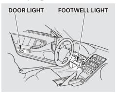
When you open the driver's door, the light for the driver's footwell turns on to assist you.
