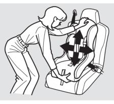
6. Push and pull the child seat forward and from side to side to verify that it is secure enough to stay upright during normal driving maneuvers. If the child seat is not secure, unlatch the belt, allow it to retract fully, then repeat these steps.
