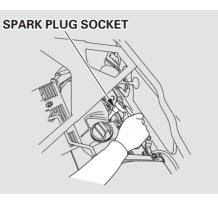
4. Remove the spark plug with a five-eighths inch (16 mm) spark plug socket.
