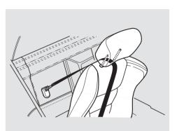
Pass the strap between the top of the seat and the bottom of the head restraint.
