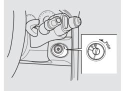
The ignition switch is on the right side of the steering column. It has four positions: •LOCK (0) •ACCESSORY (I) •ON (II) •START (III)
