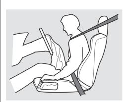
After inflating, the airbags immediately deflate, so they won't interfere with the driver's visibility, or the ability to steer or operate other controls.
