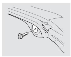
If the wind noise is unpleasant while you are driving with the roof panel removed, you can reduce the noise by inserting a plug in the hole located at each side of the rear roof pillar. These plugs are stored in the glove box.
