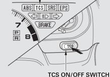
This switch is on the dashboard behind the right control pod. It lets you turn the Traction Control System on and off. You cannot turn off the TCS while the TCS indicator light is flashing.
