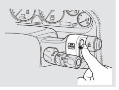
The cruise control master switch is on the right pod. For information on using the cruise control, see page125.
