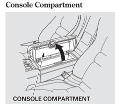
To open the console compartment, lift the tab on the left edge.
