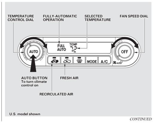
When you set the temperature to its lower limit (60 F/18 C) or its upper limit (90 F/32 C), the system runs at full cooling or heating only. It does not regulate the interior temperature. When the temperature is set between the lower and upper limits, the system regulates the interior temperature to the set value.
