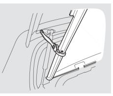
8. Put the hook around the edge of the roof cover to hold it up.
