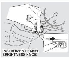
The knob on the dashboard behind the left pod controls the brightness of the instrument panel lights. Push the knob to get it to pop out. Turn the knob to adjust the brightness, then push it back in so you cannot accidentally bump it. **Rear Window Defogger**
