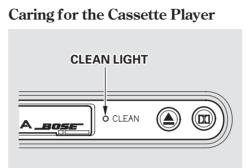
The cassette drive picks up dirt and oxides whenever you play a tape. This builds up over time and causes the sound quality to degrade. To prevent this, you should clean the cassette drive after every 30 hours of use. Your dealer has a cleaning kit available for this purpose. After 50 hours of use, the CLEAN light comes on to remind you to clean the cassette drive. After cleaning the drive, turn off the CLEAN light by pushing it in with the tip of a ballpoint pen or similar object.
