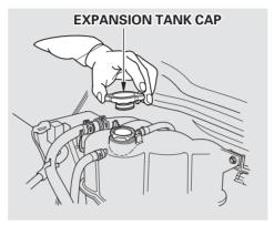
13. Fill the expansion tank to about 1 in. (2.5 cm) above the MAX line. Put the cap back on the tank, only tighten it to the first stop. Start the engine and let it run until it warms up (the radiator cooling fan comes on at least twice). 14.Turn off the engine. Check the expansion tank and, if needed, add coolant to bring it up to the MAX line. Tighten the expansion tank cap. Reinstall the cover on the car's underside.
