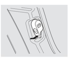
4. Open the door. Locate the rear window release handle on the rear of the driver's door opening, next to the seat. Pivot this handle towards the driver's seat. The rear window will pop up slightly.
