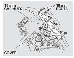
Replace the spark plugs one side at a time. Make sure the front cylinder ignition coils and the back side of the cover are marked "FR" and the rear cylinder ignition coils and the back side of the cover are marked "RR". To replace them:
