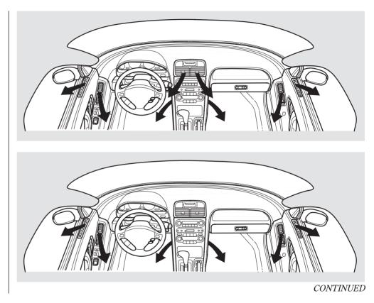
The main air flow is divided between the floor vents and windshield defroster vents.
