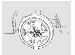
12. Put on the folding spare tire with the air valve toward the bottom. Put the wheel nuts back on fingertight, then tighten them in a crisscross pattern with the wheel wrench until the wheel is firmly against the hub. Do not try to tighten them fully. Inflate the folding spare tire only when it is on the car. Inflating it while it is lying on the ground may trap stones or other foreign matter between the tire and the wheel rim.
