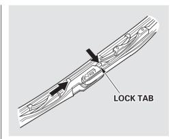
2. Disconnect the blade assembly from the wiper arm by pushing in the lock tab. Hold it in while you push the blade assembly toward the base of the arm.
