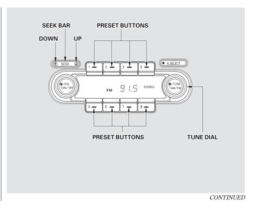
The A. SELECT function allows you to find stations easily when you are in an unfamiliar area. Press the A. SELECT button. The system automatically scans both the AM and FM bands, memorizes the eight strongest stations on each band, and stores them in the eight preset buttons. You can then use the buttons to tune to those stations. The light in the A. SELECT button stays on as a reminder.
