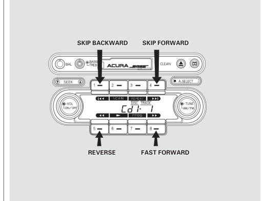
To replay the current track, press REPEAT. The indicator in the preset button will come on as a reminder. At the end of the track, the system skips back to its beginning. That track will repeat continuously until you cancel REPEAT by pressing the button again.
