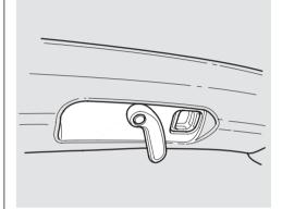
7. Make sure the roof panel release levers are in the unlocked (down) position.
