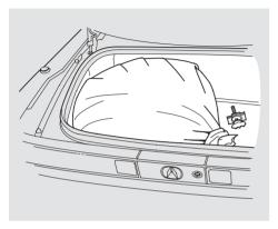
22. Slide the tire in the trunk well with the outside surface of the aluminum wheel facing up.
