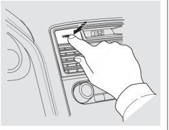
The digital clock displays the time with the ignition switch ON (II). To see the time with the ignition off, press and hold the DISPLAY button.
