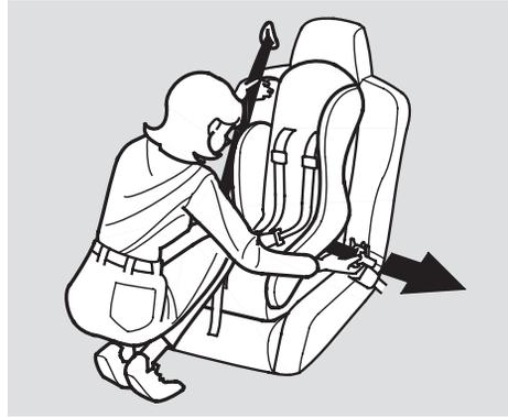
2. With the child seat in position, route the belt through the child seat according to the seat maker's instructions, then insert the latch plate into the buckle.
