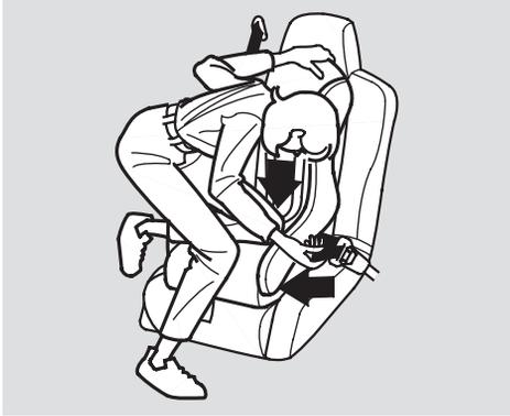
5. After confirming that the belt is locked, grab the shoulder part of the belt near the buckle and pull up to remove any slack from the lap part of the belt. Remember, if the lap part of the belt is not tight, the child seat will not be secure.
