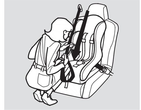
4. After the belt has retracted, tug on it. If the belt is locked, you will not be able to pull it out. If you can pull the belt out, it is not locked and you will need to repeat these steps.
