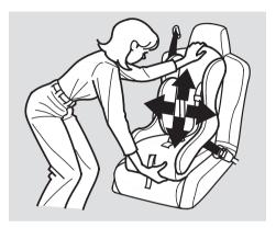
6. Push and pull the child seat forward and from side to side to verify that it is secure enough to stay upright during normal driving maneuvers. If the child seat is not secure, unlatch the belt, allow it to retract fully, then repeat these steps.
