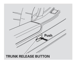
To open the trunk, press the trunk release button on the driver's door. You can also use the master key to open the trunk lock.
