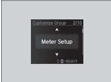
2. Roll the right selector wheel until **Meter Setup** appears on the display.
