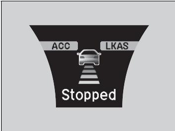
Your vehicle also stops, automatically. The **Stopped** message appears on the multi-information display. When the vehicle ahead of you starts again, the vehicle icon on the multi-information display blinks. If you press the **RES/+SET/-** switch up or down, or depress the accelerator pedal, ACC with LSF operates again within the prior set speed.
