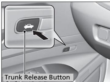
Pressing the trunk release button on the driver's door.
