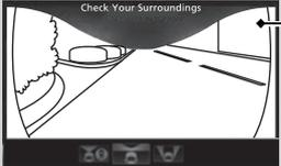
When the vehicle speed is below 12 mph (20 km/h), press the **CAMERA** button repeatedly until the front wide view comes on.
