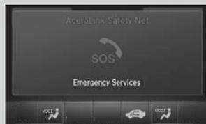
If your vehicle's airbags deploy or if the unit detects that the vehicle is severely impacted, your vehicle automatically will attempt to connect to the AcuraLink operator. Once connected, information about your vehicle, its positioning, and its condition will be sent to the operator; you also can speak to the operator when connected.
