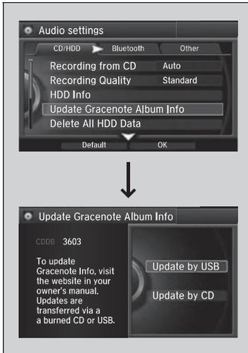
1. Insert the update disc into the disc slot or connect the USB flash drive that includes the update.
