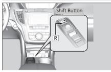
Change the gear position to  $\mathbb{R}$  with the brake pedal depressed.
