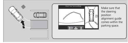
**4.** Stop the vehicle when the steering position alignment guide enters the parking space.
