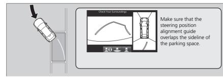
**4.** Stop the vehicle when the steering position alignment guide overlaps the sideline of the parking space.
