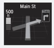
You can turn this feature on or off using the multiinformation display. See the Owner's Manual for instructions. • Direction List: Displays the map and direction list simultaneously on the map screen. When you approach a guidance point, the next guidance point appears.
