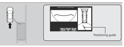
**1.** Move the vehicle forward parallel to the parking space and stop where the initial positioning guide overlaps the front corner of the parking space.
