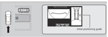
**1.** Move the vehicle forward perpendicular to the parking space and stop where the initial positioning guide comes to the center of the parking space.
