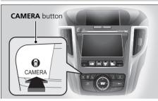
Press the **CAMERA** button while the vehicle is stopped or running slower than 7 mph (12 km/h).
