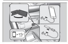
Install the iPod or iPhone USB connector or the USB flash drive to the USB port.
