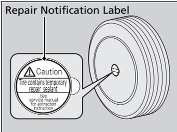
13. Apply the repair notification label to the flat surface of the wheel.
