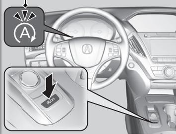
To turn the Auto Idle Stop system off, press this button. The Auto Idle Stop system stops.
