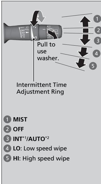
The windshield wipers and washers can be used when the power mode is in ON.
