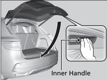
If you close the tailgate when the driver's door is locked, the tailgate locks automatically.
