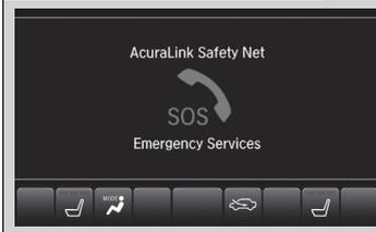
If your vehicle's airbags deploy or if the unit detects that the vehicle is severely impacted, your vehicle will automatically attempt to connect to the AcuraLink operator. Once connected, information about your vehicle, its positioning, and its condition will be sent to the operator; you also can speak to the operator when connected.
