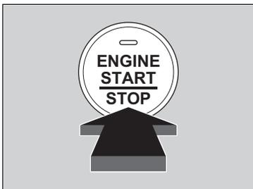
3. Press the **ENGINE START/STOP** button without depressing the accelerator pedal. The engine will crank until it starts.
