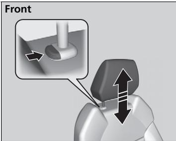
**To raise the head restraint:** Pull it upward.
