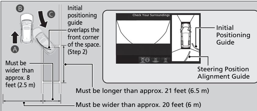
1. Press the **CAMERA** button, then press the **ENTER/MENU** button. Rotate to select **Left Parallel Park Guidance** or **Right Parallel Park Guidance**. Press .
