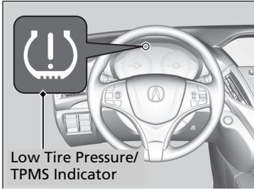
Monitors the tire pressure while you are driving. If your vehicle's tire pressure becomes significantly low, the low tire pressure/TPMS indicator comes on and a message appears on the MID.
