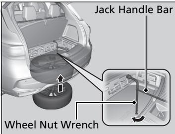
5. Turn the wheel nut wrench with the jack handle bar clockwise until the flat tire rests against the underbody of the vehicle and you hear the hoist click.
