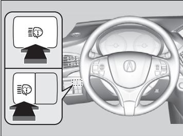
Turn the headlights on and press the headlight washer button to operate. The headlight washers also operate when you turn the windshield washers for the first time after the power mode is set to ON.
