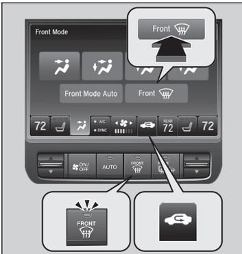
1. Press the
