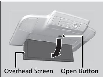
Press the open button to open and pull down the screen.
