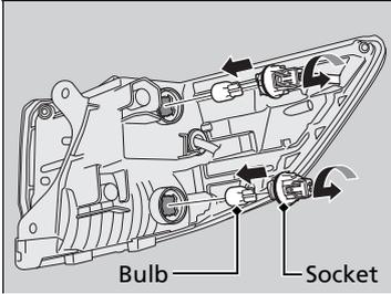
4. Turn the socket counter-clockwise and remove it. Remove the old bulb.
