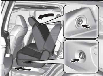
Pressing the button on the seat-back, or seat cushion tilts the second row outer seat's seat-back forward.
