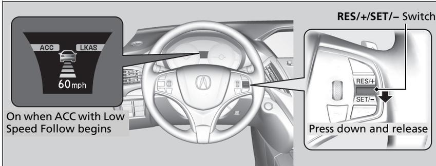
**When driving at about 25 mph (40 km/h) or above:** Take your foot off the pedal and press down the **RES/+ / SET/-** switch when you reach the desired speed. The moment you release the switch, the set speed is fixed, and ACC with Low Speed Follow begins.
