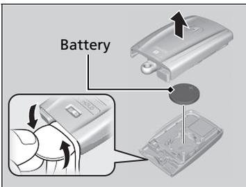
Replacing the Button Battery
