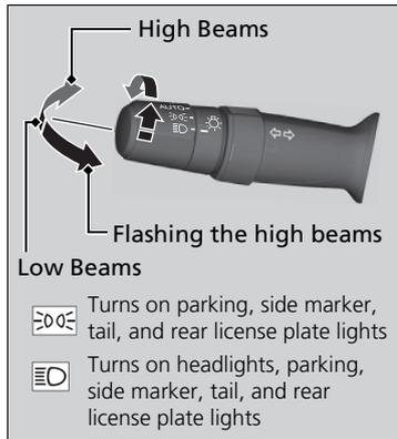
Rotating the light switch turns the lights on and off, regardless of the power mode setting.
