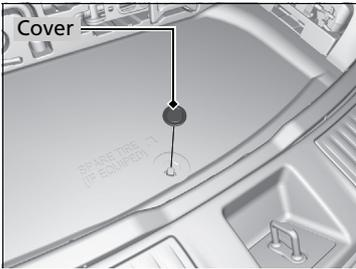
4. Remove the cover on the cargo area lining to access the shaft for the spare tire hoist.
