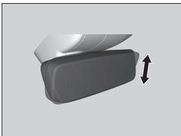
When you are driving after dark, the automatic dimming rearview mirror and power door mirrors\* reduce the glare from headlights behind you, based on inputs from the mirror sensor. This feature is always active.
