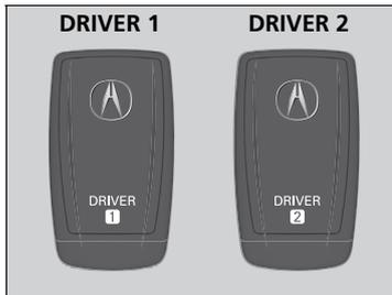
The driver's seat moves rearward and steering wheel fully up depending on the set seating position once you
