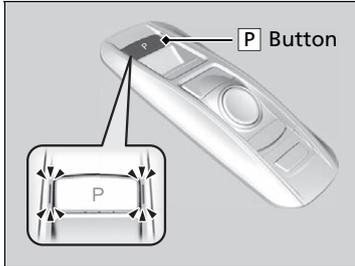
The gear position changes to **P** when you press the **P** button while the vehicle is parked with the power mode in ON. The indicators on the sides of the **P** button come on.
