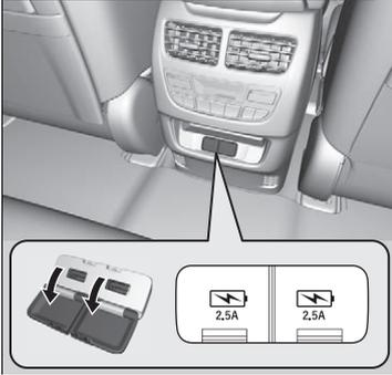
■ On the back of the front console compartment
