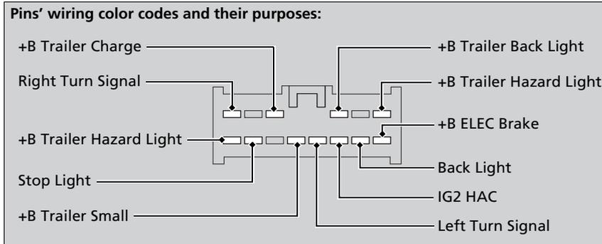
We recommend that you have a dealer install a Acura wiring harness and converter. They are designed for your vehicle.
