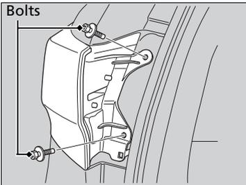
2. Use a Phillips-head screwdriver to remove the bolts.
