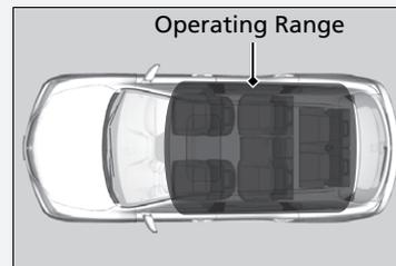
You can start the engine when the keyless access remote is inside the vehicle.
