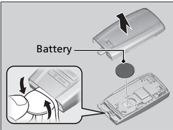
▶▶ Replacing the Button Battery
