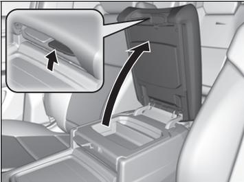
Pull the driver's side handle to open the utility tray in the console lid.
