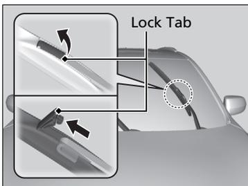
2. Pry on the edge of the lock tab using a flat-tip screwdriver to push it up.
