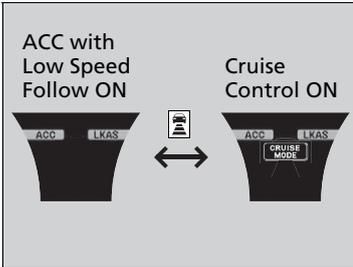
Press and hold the
