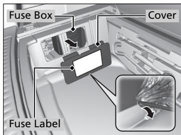
Fuse locations are shown on the cover. Locate the fuse in question by the fuse number and box cover number.
