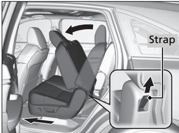
Pulling up on the strap also tilts the seat-back forward.
