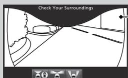
When the vehicle speed is below 7 mph (12 km/h), press the **CAMERA** button repeatedly until the front wide view comes on.
