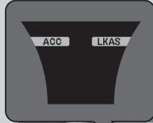
ACC (green) is on in the instrument panel. ACC with Low Speed Follow is ready to use.
