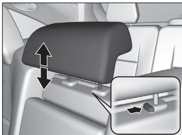
A passenger sitting in the second row center seating position should adjust the height of their head restraint to an appropriate position before the vehicle begins moving.
