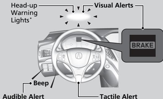
At system's earliest collision alert stage, you can change the distance (**Long/Normal/Short**) between vehicles at which alerts will come on through MID setting options.
