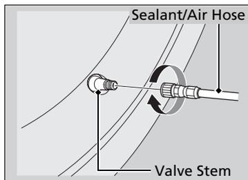
6. Attach the sealant/air hose onto the tire valve stem. Screw it until it is tight.
