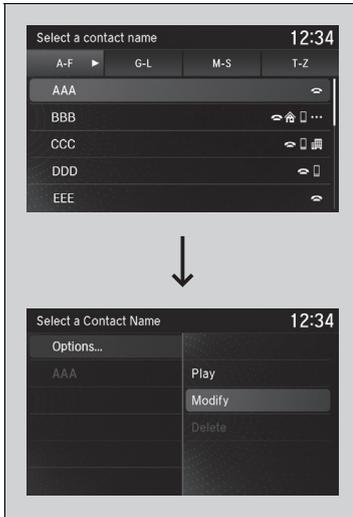
7. Move ◀ or ▶ and rotate to select a contact name, then press .
