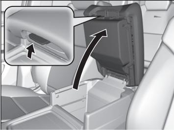
Pull the passenger's side handle to open the console compartment.
