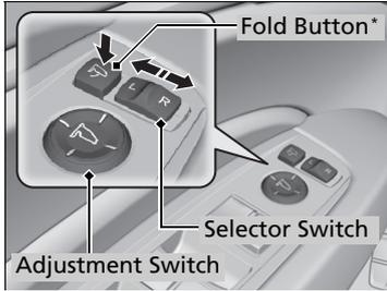
You can adjust the door mirrors when the power mode is set to ON.
