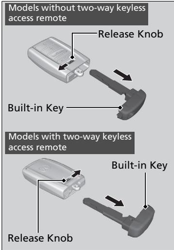
The built-in key can be used to lock/unlock the doors when the keyless access remote battery becomes weak and the power door lock/unlock operation is disabled.
