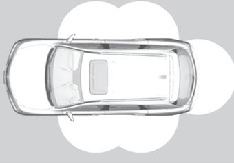
When you carry the keyless access remote, you can lock/unlock the doors and the tailgate.
