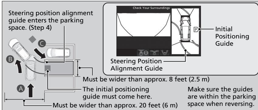
1. With your vehicle at a complete stop, press the **CAMERA** button, then press the **ENTER/MENU** button. Rotate to select **Back-in Left Park Guidance** or **Back-in Right Park Guidance**. Press .
