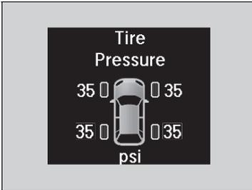
To select the tire pressure monitor, set the power mode to ON, and roll the multi-function steering-wheel controls until you see the tire pressure screen.
