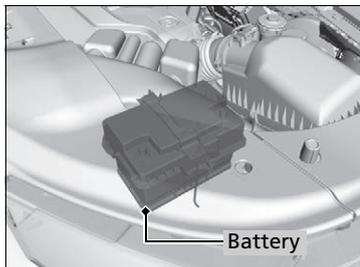
The condition of the battery is monitored by a sensor located on the negative terminal of the battery. If there is a problem with this sensor, the multi-information display (MID) will display a warning message. If this happens, have your vehicle inspected by a dealer.
