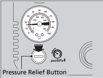
8. Press the pressure relief button until the gauge returns to 0 psi (0 kPa).
