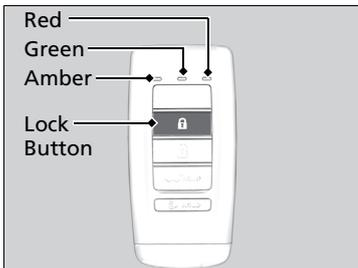
You can remotely check if your vehicle's doors are all locked or any are unlocked using the keyless access remote from extended distances.
