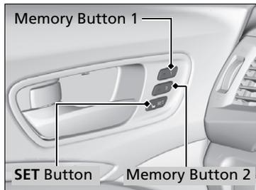
1. Set the power mode to ON. Adjust the driver's seat, the steering wheel and the door mirrors to the desired position.
