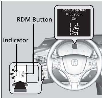
Press the RDM button to turn the system on and off.
