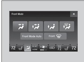
Select a desired vent mode icon, or **Front Mode Auto**: The system automatically selects the vent mode most suitable to the ambient environment.
