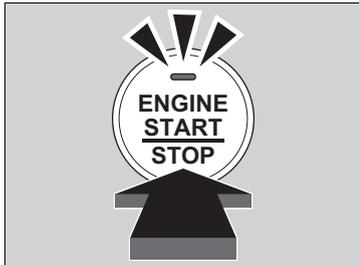
2. Depress the brake pedal and press the **ENGINE START/STOP** button within 10 seconds after the beeper sounds while the indicator stays on.
