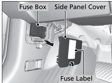
Fuse locations are shown on the label on the back side of the side panel cover. Locate the fuse in question by the fuse number and label number.
