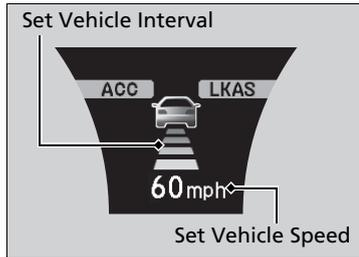
When ACC with Low Speed Follow starts operating, the vehicle icon, interval bars and set speed appear on the MID.
