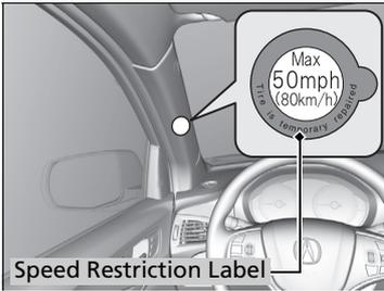
12. Apply the speed restriction label to the location as shown.
